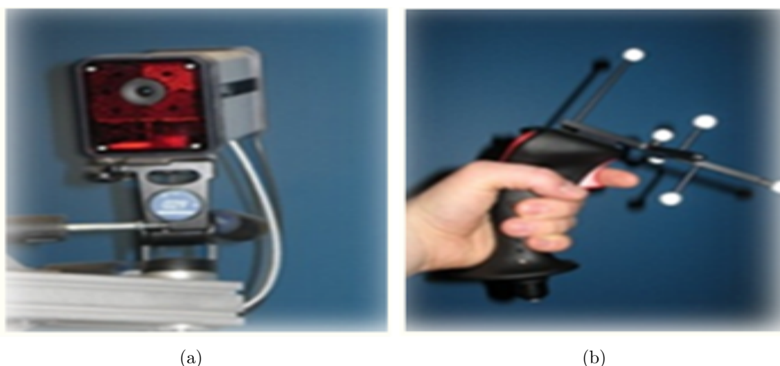
Figure 5.15: Tracking system of the semi-immersive platform (a) Infrared camera (b) Flystick with shining balls
