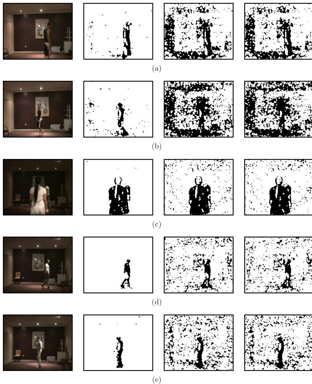
Figure 3.13 Foreground segmentation in indoor environment. For each row and from left to right: original image; foreground mask with the proposed method; foreground mask with Stauffer and Grimson's method; foreground mask with Lee's method. The changes in illumination provoke background surfaces to be detected as foreground with Stauffer and Grimson's and Lee's algorithm.
