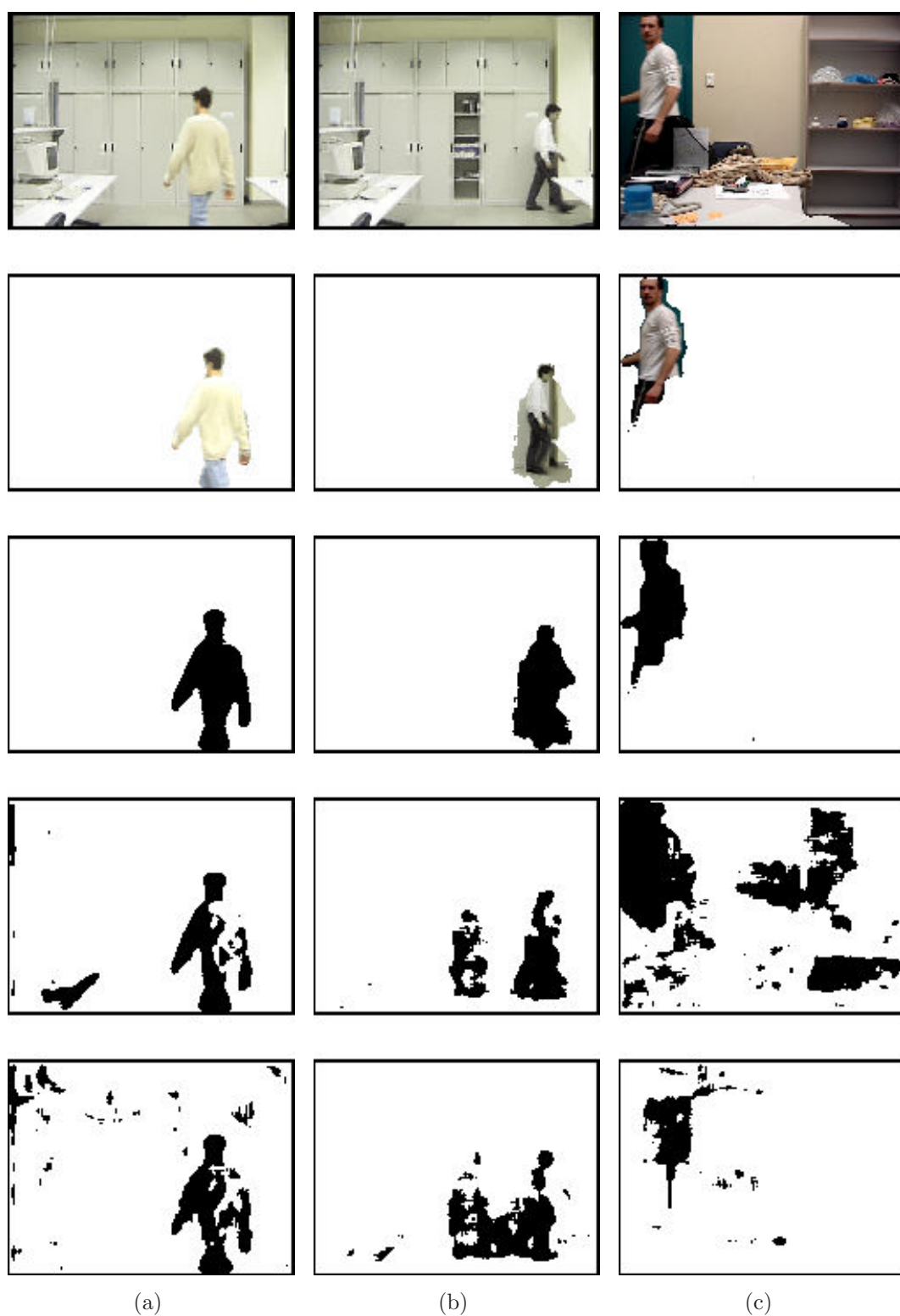
Figure 3.11 Foreground segmentation for office scenes. (a) and (b) are from Laboratory ; (c) is from Office_1 . For each column and from top to bottom: original image; foreground extraction with the proposed method; foreground mask with the proposed method; foreground mask with Stauffer and Grimson's method; foreground mask with Lee's method.
