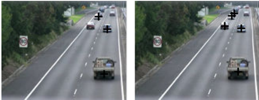
Figure 4.9 Comparison of the standard tracking algorithm ( left ) and the proposed algorithm ( right ). The proposed algorithm presents better ability to track long distance vehicles.
