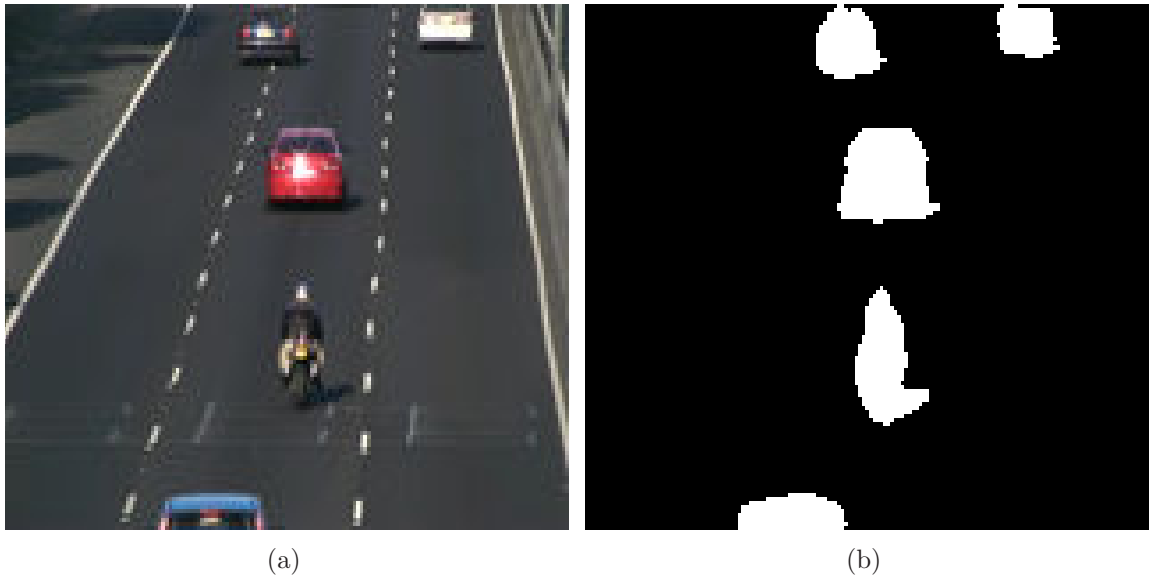
Figure 4.3 Background subtraction on a low definition image ( 128 \times 160 ): (a) original image; (b) motion mask comprising moving objects.
