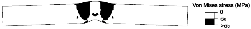
Fig. 20. Deformed shape and von Mises stress distribution in the sandwich beam (configuration 2) with elastoplastic core and global imperfection of 0.01 mm (deflection = 8 mm).
