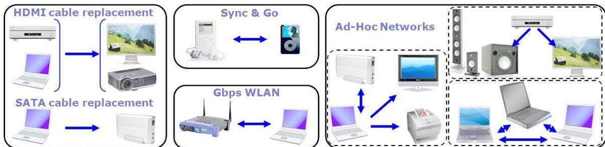
Figure I-1 Targeted applications of the new IEEE 802.15.3c standard
