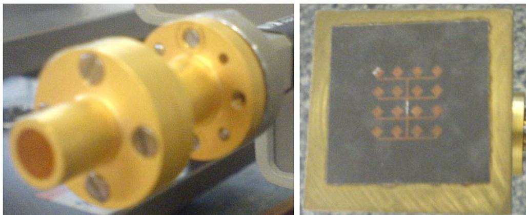
Figure I-21 Horn (left) and Patch (right) antennas
