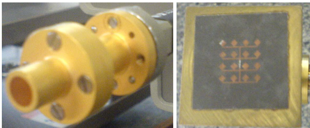
Figure I-21 Horn (left) and Patch (right) antennas
