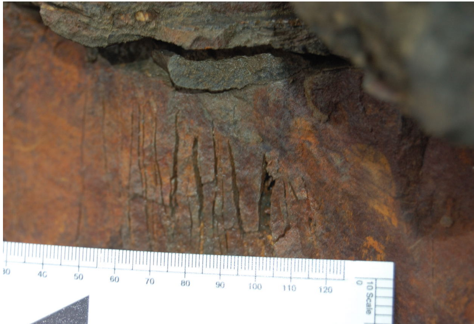
Figure 6.3: Extension fractures (axial splitting) due to a local increase of the vertical stress in combination with releasing horizontal stress. (Bude, SW-England)
