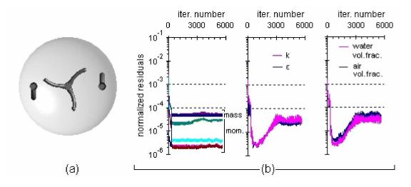
Figure 9.11. CFD simulation of the Beek reactor ( $Re = 6.6 \times 10^6$ ): (a) geometry; (b) normalized residuals versus iteration number for the momentum and mass, turbulence quantities, and volume fraction equations
