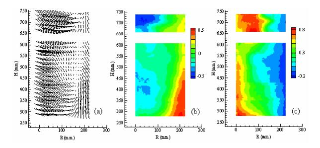
Figure 5.15. Experimental data obtained by PIV ( $\Delta t = 0.3$  ms, 960 couple of frames) for N = 275 RPM on the XY baffle plane: (a) axial-radial velocity vectors; (b) contour plot of axial velocity; (c) contour plot of radial velocity.
