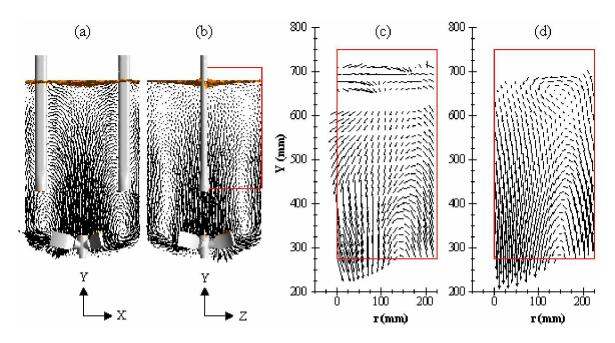
Figure 5.13. Numerical axial-radial velocity vectors for N = 100 RPM on the XY baffle plane (a) and on the YZ plane orthogonal to baffles (b); zoom of the velocity vector field on the PIV plane: (c) experimental; (d) numerical.
