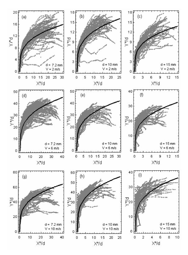
Figure 11.7. Comparison between the Lagrangian particle tracks from CFD (grey symbols) and the jet trajectory correlation (black line) at N=100 RPM for the pilot reactor. The value of the constant B of the model is set to 0.29.
