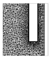
Figure 4.5. Unstructured grid used in the simulations in the region near the right baffle bottom tip and the reactor shell.
