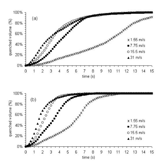
Figure 10.8. Quenching curves from the modelling of the industrial reactor at Mazingarbe for different jet velocities ( $V_o = 1.55 \text{ m/s}$ ): (a) half of the nominal agitator speed; (b) nominal agitator speed.
