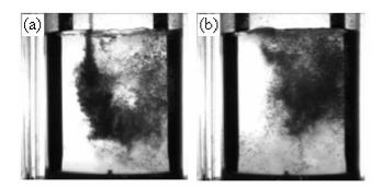
Figure 8.4. Visualisation of a water jet coloured with iodine, injected at the free-surface with classical daylight conditions (d = 10 mm, V =  $6.0 \pm 0.5$  m s<sup>-1</sup>, N = 100 RPM); (a) during injection; (b) after injection.
