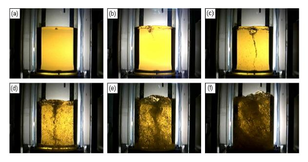
Figure 7.4. Visualization of the mixing vessel aeration for different agitator rotation speeds: (a) 50 RPM, (b) 100 RPM, (c) 150 RPM, (d) 200 RPM, (e) 250 RPM, (f) 400 RPM.
