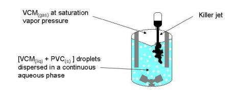
Figure 2.4. Schematic of killer injection into a PVC synthesis reactor
