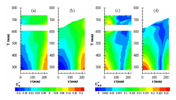
Figure 5.16. Contours plots of normalised velocity on the PIV plane for N = 200 RPM: (a) experimental axial velocity; (b) numerical axial velocity; (c) experimental axial-radial velocity; (d) numerical axial-radial velocity.
