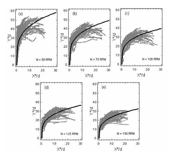
Figure 11.4. Comparison between the Lagrangian particle tracks from CFD (grey symbols) and the jet trajectory correlation (black line) with d = 10 mm and V = 6 m s<sup>-1</sup> at different agitator rotation speeds for the pilot reactor.
