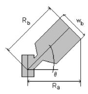
Figure 10.10. Details of an agitator blade for the calculation of A<sub>a</sub>.
