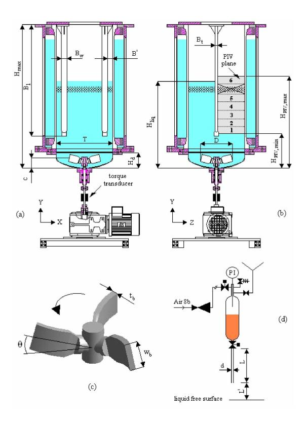
Figure 3.4. Schematic of the mixing vessel: (a) XY view of the mixing vessel; (b) YZ view of the mixing vessel; (c) details of the agitator; (d) injection system.
