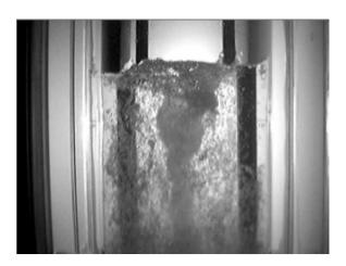
Figure 4.1. Picture of the vortex, webcam ToucamProII in Black and White mode, N=275 RPM, the tank contains 109 L of water giving an initial height of  $H_{\text{init}}=700$  mm.
