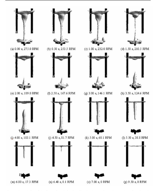
Figure 6.3. Evolution of the free-surface during impeller slowdown and stopping. Each caption gives the simulation time from the start of the impeller slowdown and the impeller rotation rate.
