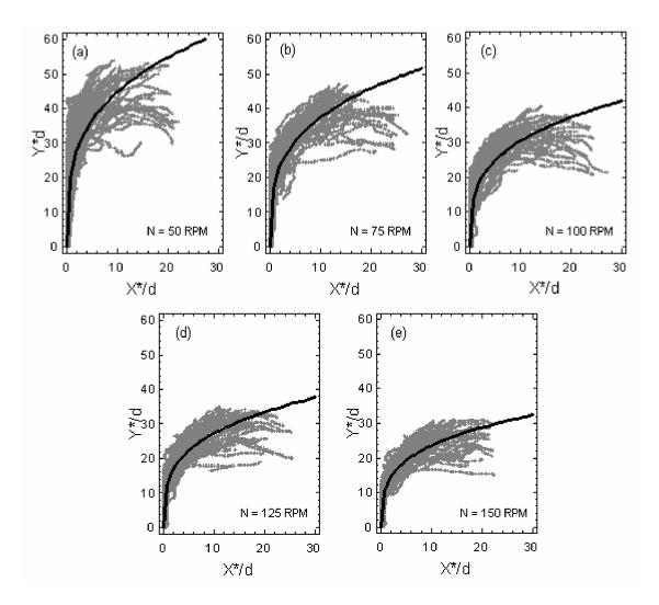
Figure 11.8. Comparison between the Lagrangian particle tracks from CFD (grey symbols) and the jet trajectory correlation (black line) with d=10 mm and V=6 m s<sup>-1</sup> at different agitator rotation speeds for the pilot reactor. The value of the constant B of the model is set to 0.29.
