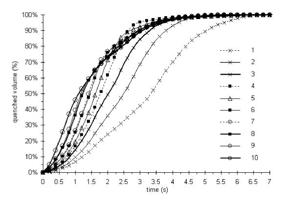
Figure 8.11. Cumulative curves of the percentage of quenched volume versus time for various jet inlet conditions. The description of each case is given in Table 8.1.
