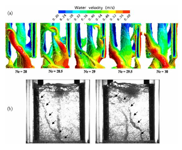
Figure 5.7. (a): Numerical isosurface of vorticity equal to  $10 \text{ s}^{-1}$  for the time period covered from the  $28^{th}$  to  $30^{th}$  agitator rotations obtained using a single-phase simulation and the k- $\epsilon$  turbulence model (N = 100 RPM), coloured by a contour plot of water velocity; (b) two successive experimental snapshots at N = 217 RPM.
