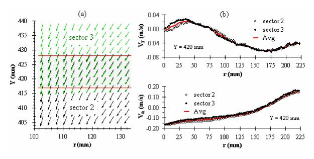
Figure 5.2. Overlapping region between two adjacent fields of view (sector 2 and sector 3). (a): superimposition of the vector fields; (b) radial and axial liquid velocities in each sectors measured on the horizontal line located at Y = 420 mm.
