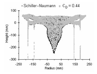
Figure 4.7. Comparison between the vortex shapes obtained using the Schiller-Naumann drag coefficient model or a constant drag coefficient equal to 0.44 (Isosurface of water volume fraction equal to 0.5).
