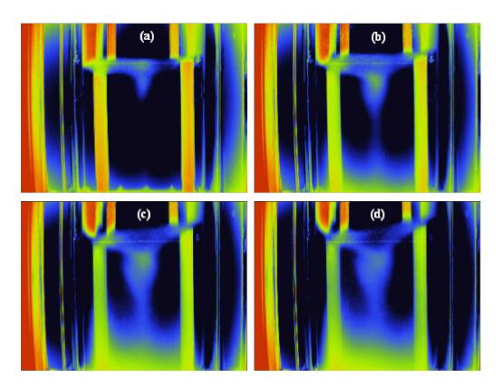
Figure 4.11. Experimental acquisitions of the vortex shapes, negative coloured pictures; (a) N = 200 RPM, G = 26000; (b) N = 250 RPM, G = 22500; (c) N = 300 RPM, G = 20000; (d) N = 350 RPM, G = 18000.
