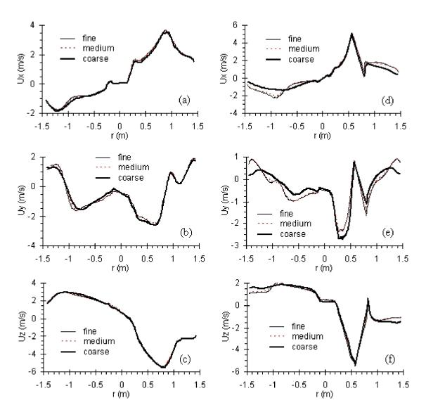
Figure 9.7. Tests of grid independence for the industrial reactors. The figure shows the effect of the grid size on the velocity components  $U_x$ ,  $U_y$  and  $U_z$ . (a), (b), (c): Mazingarbe reactor; (d), (e), (f): Beek reactor
