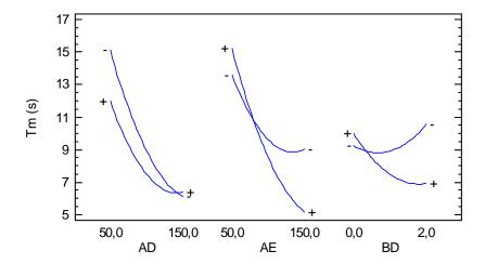
Figure 7.14. AD, AE and BD interaction plots. Abscissa shows the variation of the first letter of the plotted interaction. (+): higher level of the factor; (-): lower level of the factor.
