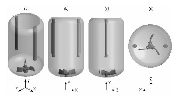
Figure 9.4. Geometry of the Mazingarbe reactor with the standard baffling configuration. (a) 3D view, (b) lateral XY view; (c) lateral YZ view; (d) top view
