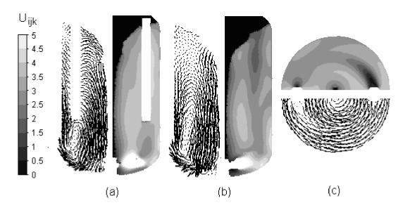
Figure 9.12. Hydrodynamics on the Mazingarbe industrial reactor with the baffles providing the maximum perturbation (Re =  $5.0 \times 10^6$ ): (a) XY baffles plane; (b) YZ orthogonal baffle plane; (c) ZH horizontal plane at Y =  $H_{liq}/2$ ; ( $\alpha_l > 0.9$ ).
