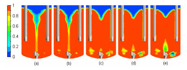
Figure 4.6. Water volume fraction profiles on the XY plane containing the baffles obtained using different air bubble diameter: (a)  $d_b = 1$  mm; (b)  $d_b = 3$  mm; (c)  $d_b = 5$  mm; (d)  $d_b = 7$  mm, (e)  $d_b = 10$  mm.
