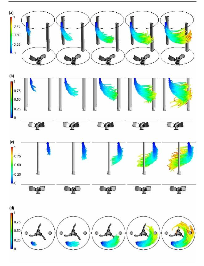
Figure D.3. Lagrangian jet trajectories coloured by the Lagrangian particle travel time normalized by  $T_{inj}$ , for d=0.1 m,  $V=20V_o=15.5$  m s<sup>-1</sup> and  $Re=5\times10^6$ , plotted at  $0.2T_{inj}$ ,  $0.4T_{inj}$ ,  $0.6T_{inj}$ ,  $0.8T_{inj}$  and  $T_{inj}$ . (a) 3D view; (b) XY lateral view; (c) YZ lateral view; (d) top view.
