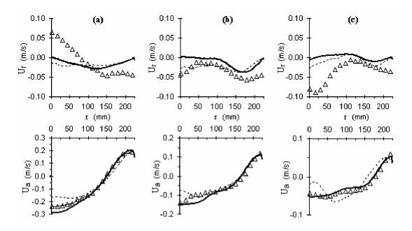
Figure 5.8. Comparisons between radial/axial velocity measurements obtained by PIV and CFD predictions at different heights (N = 100 RPM); symbols: PIV; bold line: CFD with the k- $\epsilon$  model; dashed line: CFD with the Reynolds Stress (SSG) model; (a) Y = 318 mm; (b) Y = 458 mm; (c) Y = 598 mm.
