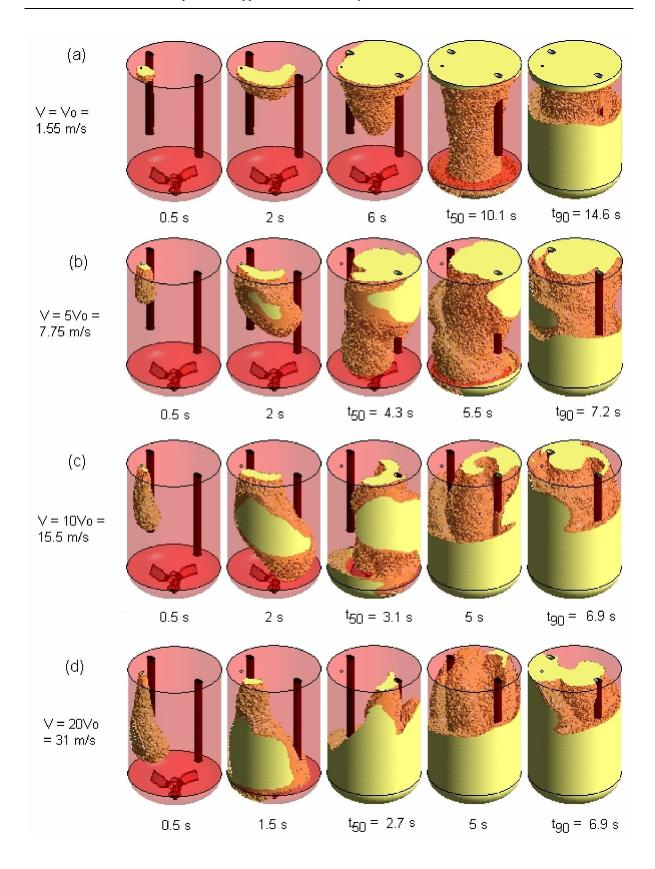
Figure 10.7. Evolution of the reactor quenched volume versus time with different jet injection velocities for half of the nominal agitator speed: (a)  $V_0 = 1.55 \text{ m s}^{-1}$ ; (b)  $V = 7.75 \text{ m s}^{-1}$ ; (c)  $V = 15.5 \text{ m s}^{-1}$ ; (d)  $V = 31 \text{ m s}^{-1}$ .
