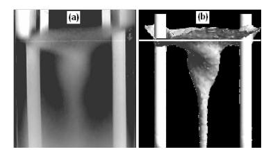
Figure 4.10. Comparison on the same scale of the experimental (a) and the numerical (b) vortex shapes; (a) negative coloured picture, G = 21000, N = 275 RPM; (b) isosurface of water volume fraction equal to 0.9 (N = 275 RPM).
