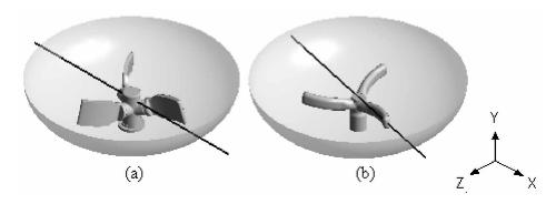
Figure 9.6. Lines where the velocity data was extracted for grid independency tests: (a) Mazingarbe reactor,  $Y_{line} = 400 \text{ mm}$ ; (b) Beek reactor,  $Y_{line} = 350 \text{ mm}$ .
