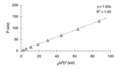
Figure 9.17. Prediction of the power input via the torque calculation for eight rotation speeds (30 RPM < N < 100 RPM) for the industrial Mazingarbe reactor.
