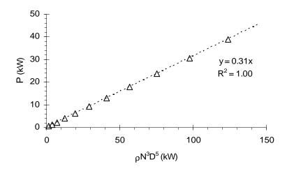
Figure 9.20. Prediction of the power input via the torque calculation for eleven rotation speeds (30 RPM < N < 130 RPM) for the industrial Beek reactor.
