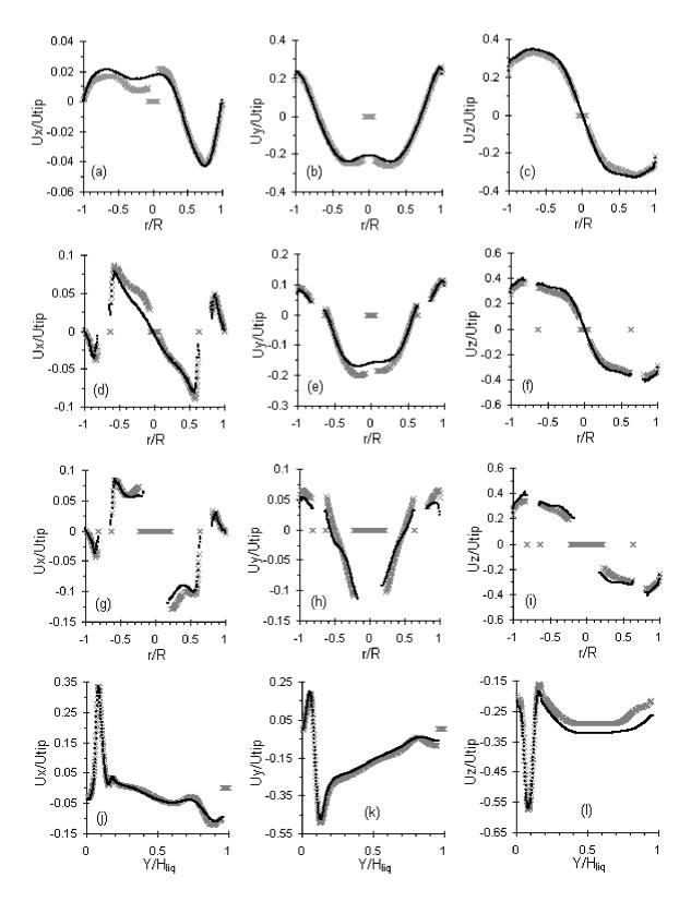
Figure 12.8. Comparison of the radial  $U_x$ , axial  $U_y$  and circumferential  $(U_z)$  velocity values on different locations on the baffle plane (N = 275 RPM) for the inhomogeneous model (black symbols) and the free-surface cut strategy (grey symbols). (a), (b),(c): Y = 200 mm; (c), (d), (e): Y = 400 mm; (f), (g), (h): Y = 600 mm, (i), (j), (k): vertical line at r = 75 mm from the vessel axis.
