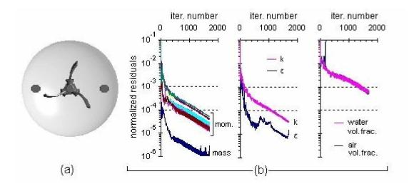
Figure 9.9. CFD simulation of the Mazingarbe reactor with the baffles giving the maximal perturbation (Re =  $5.0 \times 10^6$ ): (a) geometry; (b) normalized residuals versus iteration number for the momentum and mass, turbulence quantities, and volume fraction equations
