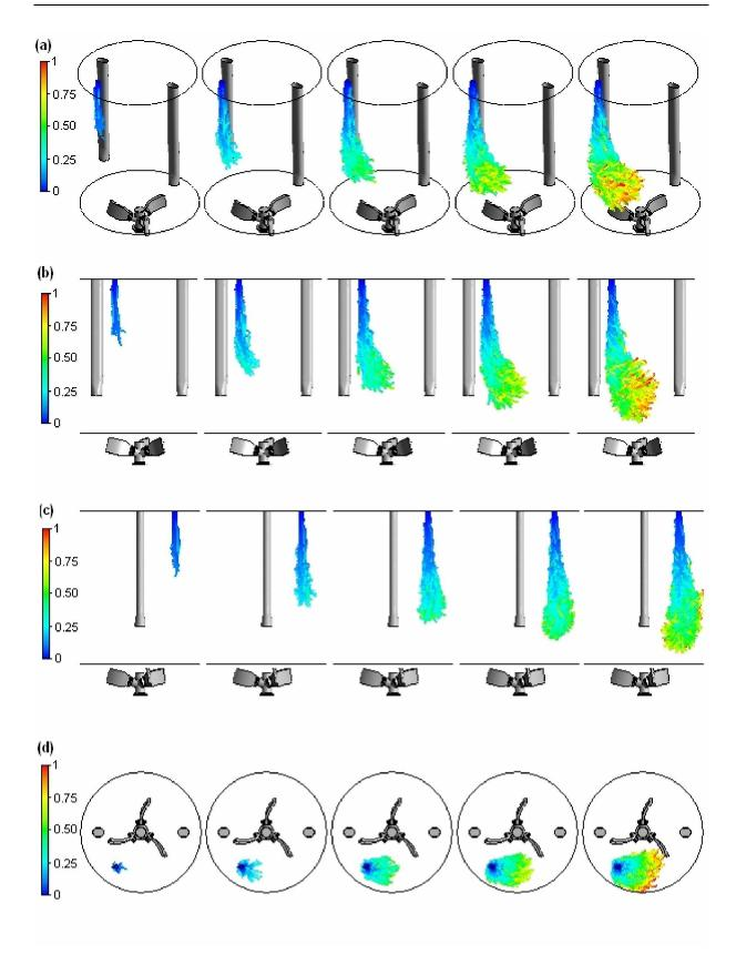
Figure 10.6. Lagrangian jet trajectories coloured by the Lagrangian particle travel time normalized by  $T_{inj}$ , for d=0.1 m,  $V=20V_o=31$  m s<sup>-1</sup> and  $Re=2.5\times10^6$ , plotted at  $0.2T_{inj}$ ,  $0.4T_{inj}$ ,  $0.6T_{inj}$ ,  $0.8T_{inj}$  and  $T_{inj}$ . (a) 3D view; (b) XY lateral view; (c) YZ lateral view; (d) top view.
