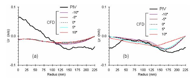
Figure 5.9. Comparison between experimental PIV data and numerical CFD predictions of the radial velocity on other planes inclined at  $\pm 5^{\circ}$  and  $\pm 10^{\circ}$  to the original plane: (a) Y = 318 mm; (b) Y = 458 mm.
