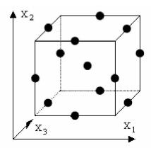
Figure 7.6. Graphical representation of BBD with three factors.
