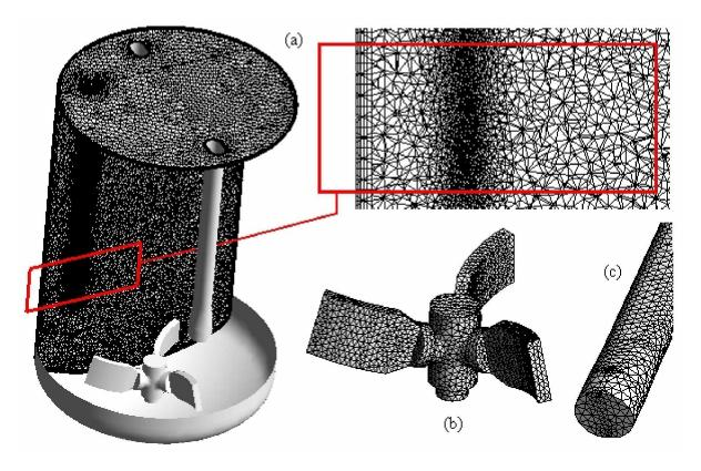
Figure 8.2. The mesh used for the CFD simulations; (a) vertical plane passing through the centre of the injection surface; (b) details of the mesh on the agitator and (c) on a baffle.
