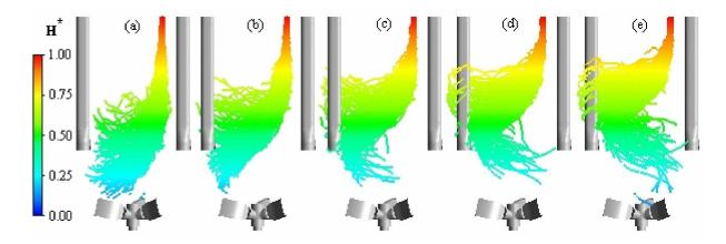
Figure 8.8. Lagrangian particle tracking (300 particles) showing the jet penetration profile (d = 10 mm, V = 6 m s<sup>-1</sup>) at the end of the injection time for different agitator rotation speeds, coloured with the normalized vessel height  $H^*$  (= Y/H<sub>liq</sub>). (a) N = 50 RPM; (b) N = 75 RPM; (c) N = 100 RPM; (d) N = 125 RPM; (e) N = 150 RPM.
