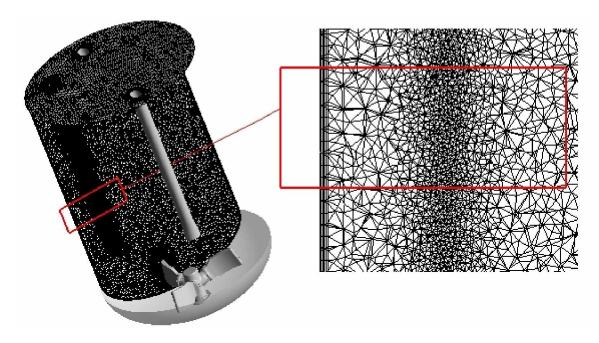
Figure 10.2. Details of the mesh used for the CFD simulations of the Mazingarbe industrial reactor on a vertical plane passing through the centre of the injection surface
