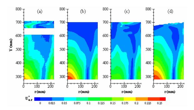
Figure 5.11. Contours plots of normalized axial-radial velocity on the PIV plane for N=100 RPM: (a) experimental PIV data; (b) single phase numerical data using the k- $\epsilon$  model; (c) single phase numerical data using the Reynolds Stress (SSG) model; (d) multiphase numerical data using the k- $\epsilon$  model.
