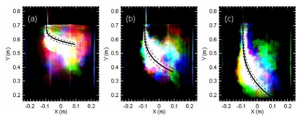
Figure 11.13. Comparison between experimental pictures of jet injections obtained using the trichromy imaging process and the theoretical jet trajectory correlation (full line) at N = 100 RPM. (a)  $V = 2.1 \pm 0.1$  m s<sup>-1</sup>; (b)  $V = 6.0 \pm 0.5$  m s<sup>-1</sup>; (c)  $V = 9.9 \pm 0.6$  m s<sup>-1</sup>. The dotted lines show the uncertainty limits for each trajectory predicted by the correlation.
