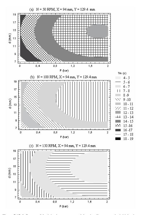
Figure 7.17. Influence of the injection pressure and the pipe diameter at the initial point.
