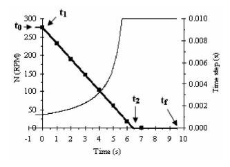
Figure 6.2. Agitator speed (bold line) and time-step (normal line) used in the simulations for modelling the agitator stopping. (n): experimental points for the free-surface shape comparison.
