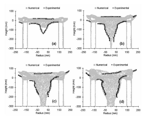
Figure 4.12. Comparison between experimental vortex shapes (negative coloured pictures with the optimal gain) and the projection on the XY vertical plane of isosurfaces of water volume fraction equal to 0.9; (a) 200 RPM; (b) 250 RPM; (c) 300 RPM; (d) 350 RPM.
