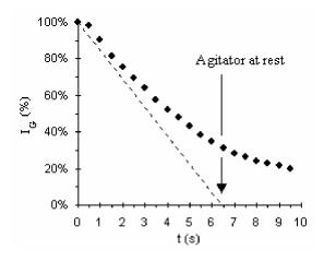
Figure 6.6. The agitation index versus time during the agitator stopping phase and the inertial period.
