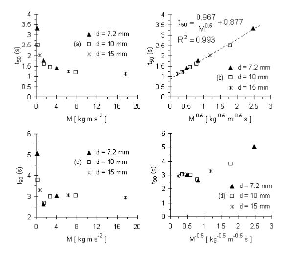
Figure 8.12. Evolutions of the various mixing criteria versus jet momentum flux and jet momentum flux to the power -0.5, at N = 100 RPM; (a)  $t_{50}$  versus M; (b)  $t_{50}$  versus  $M^{-0.5}$ ; (a)  $t_{90}$  versus M; (b)  $t_{90}$  versus  $M^{-0.5}$ .
