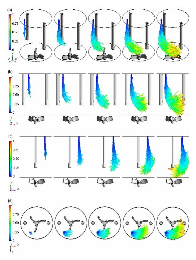
Figure 8.7. Lagrangian jet trajectories coloured by the Lagrangian particle travel time normalized by  $T_{inj}$ , for d=10 mm, V=10 m  $s^{-1}$  and N=100 RPM, obtained at  $0.2T_{inj}$ ,  $0.4T_{inj}$ ,  $0.6T_{inj}$ ,  $0.8T_{inj}$  and  $T_{inj}$ . (a) 3D view; (b) XY lateral view; (c) YZ lateral view; (d) top view.
