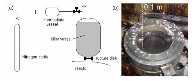
Figure 10.1. Industrial killer system for Mazingarbe reactors. (a) schematic of the installation; (b) picture of the carbon rupture disk.
