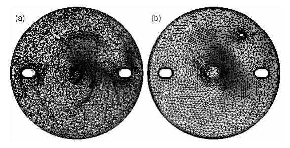
Figure 12.6. Details of the mesh on the free-surface shown from above: (a) inhomogeneous approach; (b) free-surface cut-away, note the jet injection location in the top right quadrant.
