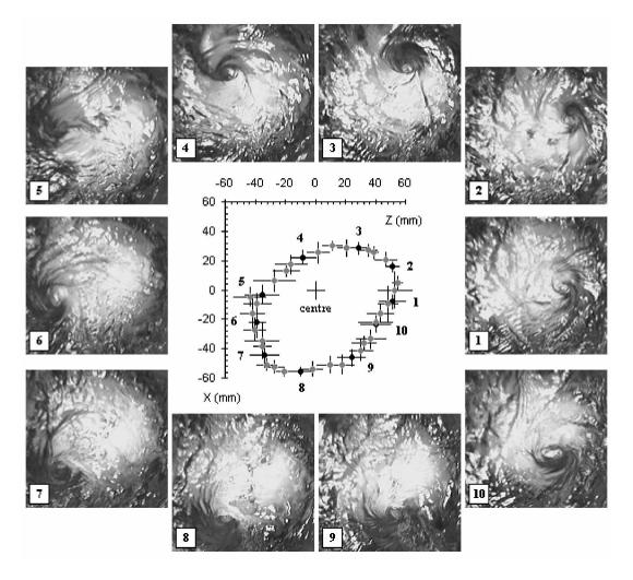
Figure 5.6. Snapshots of the precessing vortex visible on the free-surface (N = 100 RPM) and trajectory around the vessel axis; The Z direction is in the plane orthogonal to the baffles; X direction in the baffle plane; the centre is located on the vessel axis.
