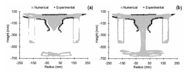
Figure 4.9 Comparison between experimental vortex shape profile (negative coloured picture, G = 21,000, N = 275 RPM) and the projection on the XY vertical plane of isosurfaces of water volume fraction (N = 275 RPM); (a) isosurface of water volume fraction equal to 0.5; (b) isosurface of water volume fraction equal to 0.9.
