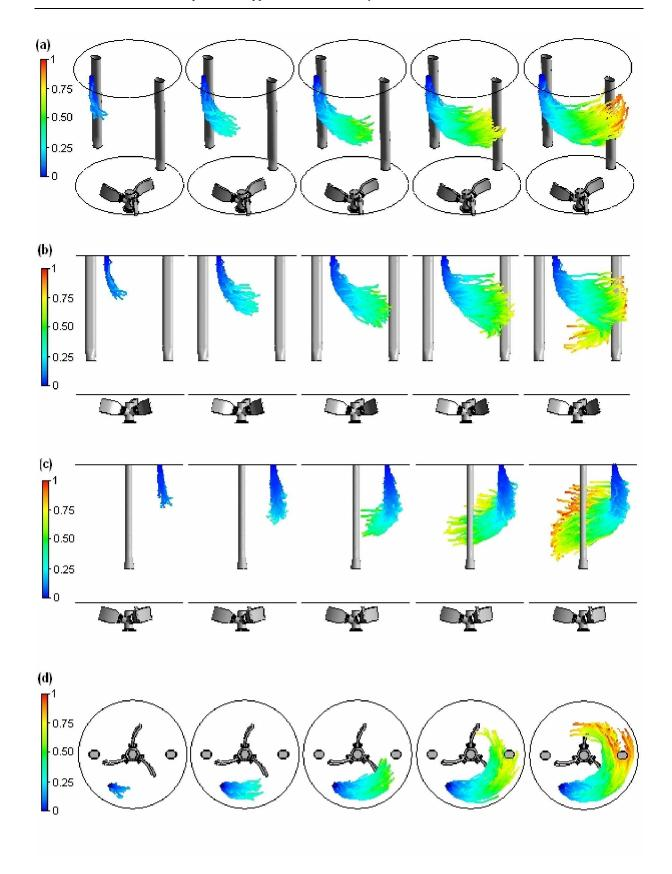
Figure 10.4. Lagrangian jet trajectories coloured by the Lagrangian particle travel time normalized by  $T_{inj}$ , for d = 0.1 m,  $V = 5V_o = 7.75$  m s<sup>-1</sup> and  $Re = 2.5 \times 10^6$ , plotted at  $0.2T_{inj}$ ,  $0.4T_{inj}$ ,  $0.6T_{inj}$ ,  $0.8T_{inj}$  and  $T_{inj}$ . (a) 3D view; (b) XY lateral view; (c) YZ lateral view; (d) top view.
