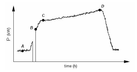
Figure 9.19. General profile of a power curve of an agitator motor obtained during a complete S-PVC polymerization in the Beek reactor: A: reactor empty; B: reactor filled with only water; C: start of polymerization; D: end of polymerization. Note that the agitator was stopped for a period between A and B leading to zero power.
