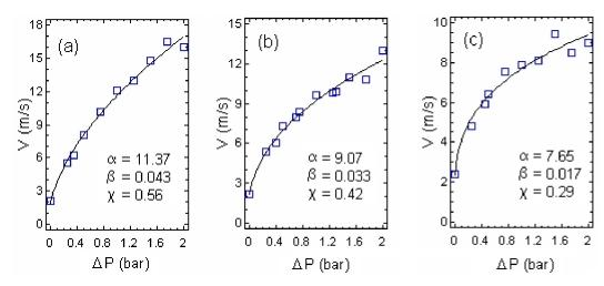
Figure C.1. Non-linear fitting of the jet velocity experimental data for the three jet diameters fitted by a law of the type  $V = \alpha(\Delta P + \beta)^{\chi}$ : (a) d = 7.2 mm; (b) d = 10 mm; (c) d = 15 mm.
