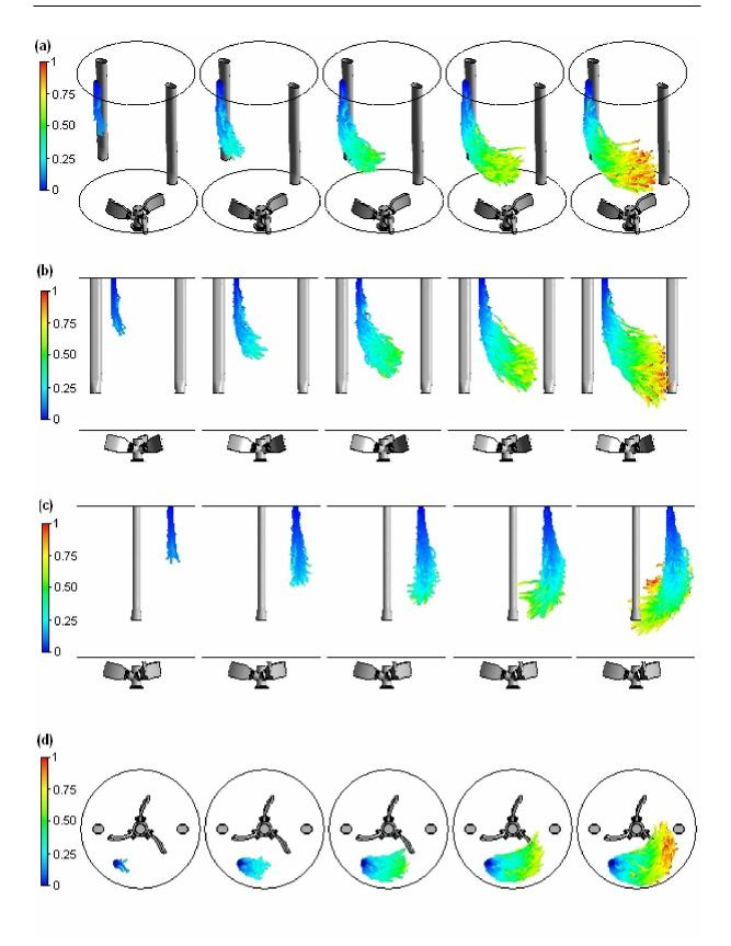
Figure D.4. Lagrangian jet trajectories coloured by the Lagrangian particle travel time normalized by  $T_{inj}$ , for d=0.1 m,  $V=20V_o=31$  m s<sup>-1</sup> and  $Re=5\times10^6$ , plotted at  $0.2T_{inj}$ ,  $0.4T_{inj}$ ,  $0.6T_{inj}$ ,  $0.8T_{inj}$  and  $T_{inj}$ . (a) 3D view; (b) XY lateral view; (c) YZ lateral view; (d) top view.
