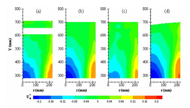
Figure 5.10. Contours plots of normalized axial velocity on the PIV plane for N = 100 RPM: (a) experimental PIV data; (b) single phase numerical data using the k- $\epsilon$  model; (c) single phase numerical data using the Reynolds Stress (SSG) model; (d) multiphase numerical data using the k- $\epsilon$  model.
