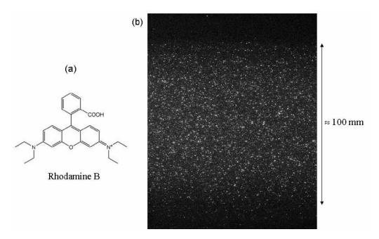
Figure 3.9. Molecular formula of the Rhodamine-B; (b) water and Rhodamine B exposed by the Nd-YAG
