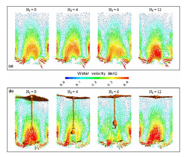
Figure 5.4. Axial-radial instantaneous velocity vectors on the vertical median plane of the two baffles obtained after steady-state ( $N_r = 0$ ) and at the end of  $N_r = 4$ , 6 and 12 agitator revolutions, N = 100 RPM: (a) single phase simulation; (b) two phase simulation.
