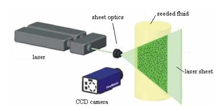
Figure 3.5. System components for PIV (inspired from <a href="www.piv.de">www.piv.de</a>).
