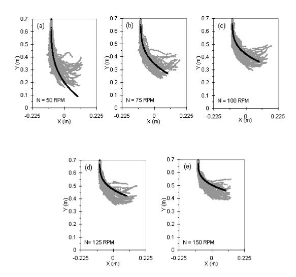
Figure 11.11. Comparison between the Lagrangian particle tracks from CFD (grey symbols) and the jet trajectory obtained by using Eq. (11.7) (black line) with d = 10 mm and V = 6 m s<sup>-1</sup> for different agitator rotation speeds (pilot reactor).
