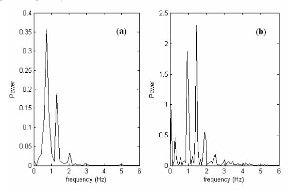
Figure 5.5. Fast Fourier Transform power spectrum of the velocity; Y = 200 mm, r = 75 mm, N = 100 RPM; (a)  $k-\varepsilon$  model, (b) SSG Reynolds Stress model.
