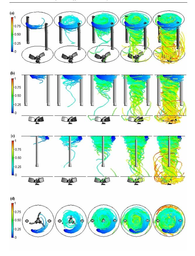
Figure 10.3. Lagrangian jet trajectories coloured by the Lagrangian particle travel time normalized by  $T_{inj}$ , for d = 0.1 m,  $V = V_o = 1.55$  m s<sup>-1</sup> (current injection conditions) and  $Re = 2.5 \times 10^6$ , plotted at  $0.2 T_{inj}$ ,  $0.4 T_{inj}$ ,  $0.6 T_{inj}$ ,  $0.8 T_{inj}$  and  $T_{inj}$ . (a) 3D view; (b) XY lateral view; (c) YZ lateral view; (d) top view.
