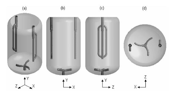
Figure 9.5. Geometry of the Beek reactor. (a) 3D view, (b) lateral XY view; (c) lateral YZ view; (d) top view
