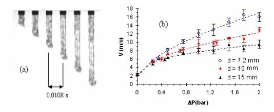
Figure 8.3. (a) Snapshots of a water jet released in air obtained with d=10 mm and V=2.1 m s<sup>-1</sup>  $\pm$  0.1 ( $\Delta P=0$  bar); (b) jet velocities versus the pressure measured in the sampling cylinder for three injection pipe diameters (7.2, 10 and 15 mm), symbols: arithmetic average of 5 experiments, error bars:  $\pm \sigma$ .
