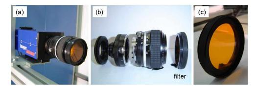
Figure 3.10. PIV camera: (a) camera equipped with the telephoto lens and the filter; (b) telephoto lens Nikkor 50 mm and its mounting rings; (c) high pass filter  $\lambda_{cut} = 550$  nm.
