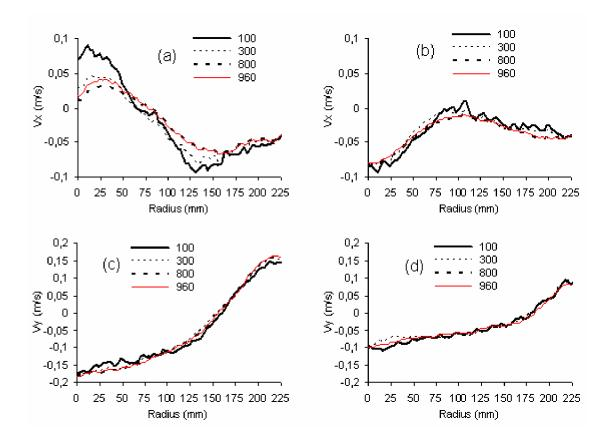
Figure 5.1. Experimental velocities for N = 100 RPM on the lines Y = 388 mm and Y = 528 mm for four different numbers of PIV images pairs: (a) radial velocity Vx at Y = 388 mm, (b) radial velocity Vx at Y = 528 mm, (c) axial velocity Vy at Y = 388 mm, (d) axial velocity Vy at Y = 528 mm.
