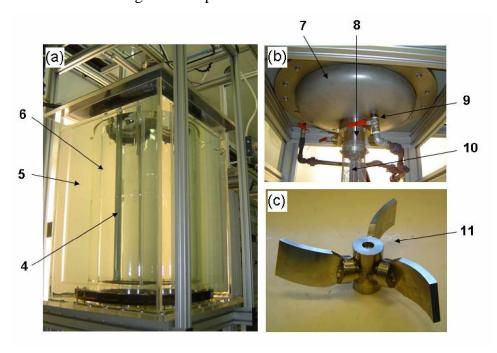
Figure 3.2. Pictures of the different elements of the mixing vessel: (a) vessel shell and jacket; (b) bottom dish; (c) agitator.
