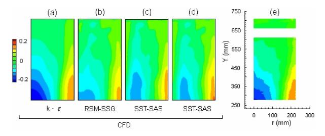
Figure 12.3. Contour plot of the averaged axial velocity obtained on the PIV plane and comparison with the experimental data. (a) k- $\varepsilon$  model, averaging over 15 agitator rotations.; (b) RSM-SSG, averaged over 15 agitator rotation; (c) SST-SAS,  $\Delta t = 0.3$  ms, averaged during 15 agitator rotations., (d) SST-SAS,  $\Delta t = 3$  ms, averaged over 30 agitator rotations; (e) experimental PIV data.
