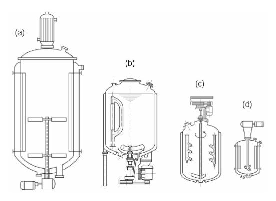
Figure 2.2. Changes of reactor shape for different reactor volumes. (a)  $60 \sim 200 \text{ m}^3$ ; (b)  $30 \sim 60 \text{ m}^3$ ; (c)  $10 \sim 30 \text{ m}^3$ ; (d)  $4 \text{ m}^3$  (from Saeki and Emura, 2002).
