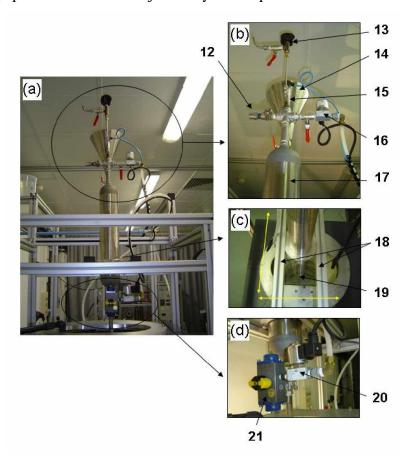
Figure 3.3. Pictures of the different elements of the injection system: (a) the top of the injection system; (b) the bottom of the injection system and sash; (c) the draining equipment.
