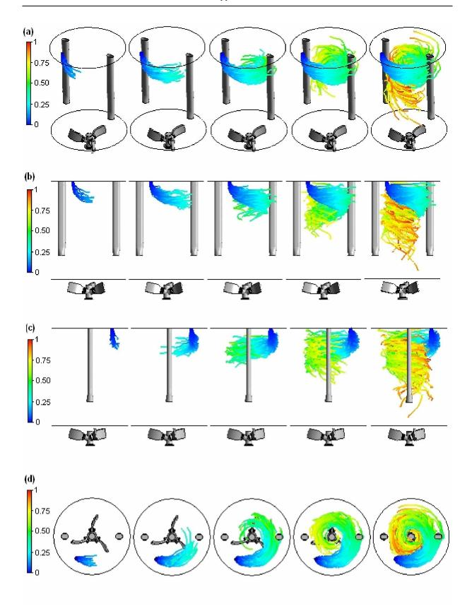
Figure D.2. Lagrangian jet trajectories coloured by the Lagrangian particle travel time normalized by  $T_{inj}$ , for d=0.1 m,  $V=20V_o=7.75$  m s<sup>-1</sup> and  $Re=5\times10^6$ , plotted at  $0.2T_{inj}$ ,  $0.4T_{inj}$ ,  $0.6T_{inj}$ ,  $0.8T_{inj}$  and  $T_{inj}$ . (a) 3D view; (b) XY lateral view; (c) YZ lateral view; (d) top view.
