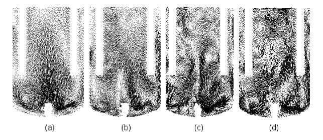
Figure 12.2. Axial-radial vector plots of the instantaneous velocity field obtained by CFD using different turbulence models (on the same grid): (a) k- $\epsilon$ ; (b) RSM-SSG; (c) SST-SAS,  $\Delta t = 0.3$  ms; SST-SAS,  $\Delta t = 3$  ms.
