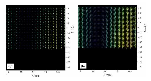
Figure 3.12. Multi-pass calculation and influence of the size of the interrogation area for an averaged velocity field (a) first step:  $64 \text{ pixels}^2$ ; (b) last step:  $32 \text{ pixels}^2$  with 50% overlap. Y = 0 corresponds to the centre of the laser sheet.
