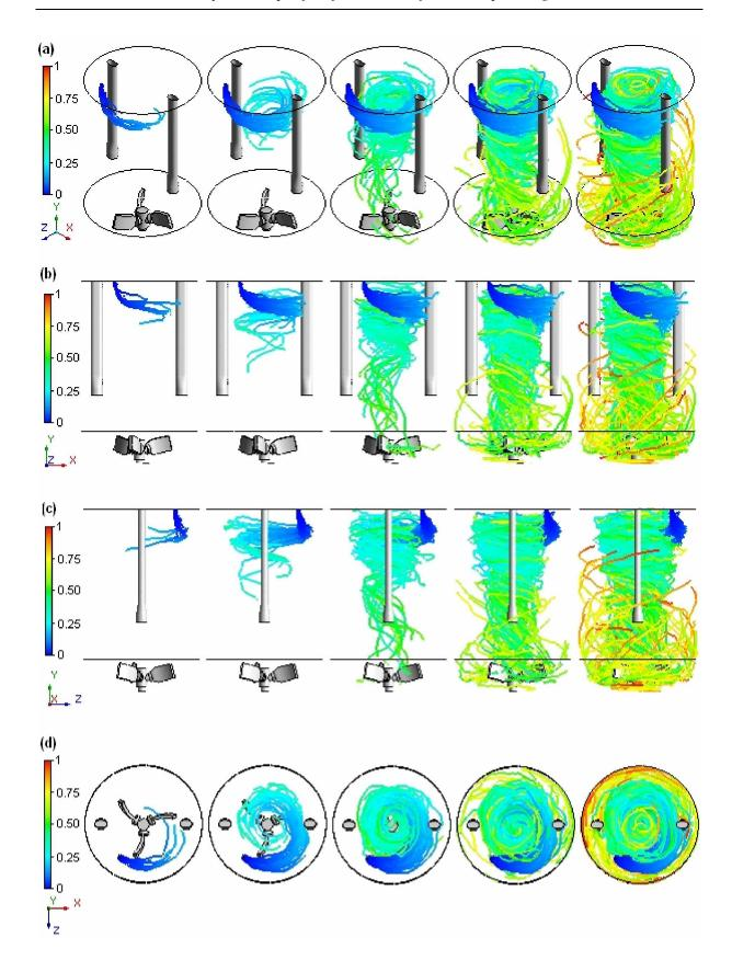
Figure 8.6. Lagrangian jet trajectories coloured by the Lagrangian particle travel time normalized by  $T_{inj}$ , for d=7.2 mm, V=2 m  $s^{-1}$  and N=100 RPM, plotted at  $0.2T_{inj}$ ,  $0.4T_{inj}$ ,  $0.6T_{inj}$ ,  $0.8T_{inj}$  and  $T_{inj}$ . (a) 3D view; (b) XY lateral view; (c) YZ lateral view; (d) top view.
