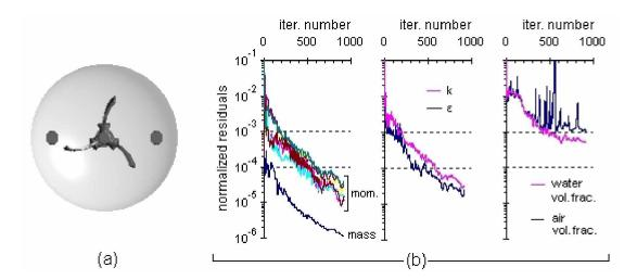
Figure 9.10. CFD simulation of the Mazingarbe reactor with the baffles providing the least perturbation ( $Re = 5.0 \times 10^6$ ): (a) geometry; (b) normalized residuals versus iteration number for the momentum and mass, turbulence quantities, and volume fraction equations.
