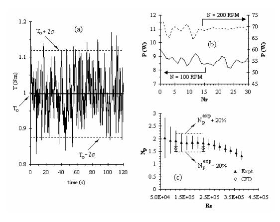
Figure 5.12. (a) Experimental measurement of the torque for N=100 RPM; (b) Simulated power consumption versus number of agitator revolutions for N=100 RPM and N=200 RPM. (c) Experimental and computed power number versus Reynolds number.
