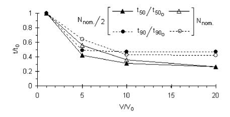
Figure 10.9. Influence of the jet velocity on  $t_{50}$  and  $t_{90}$ , for the two agitation speeds tested, and for jet velocities equal to  $V_o$ ,  $5V_o$ ,  $10V_o$  and  $20V_o$ .
