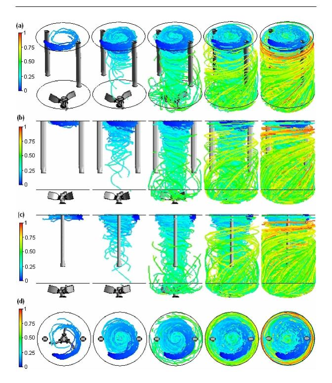
Figure D.1. Lagrangian jet trajectories coloured by the Lagrangian particle travel time normalized by  $T_{inj}$ , for d=0.1 m,  $V=20V_o=1.55$  m s<sup>-1</sup> and  $Re=5\times10^6$ , plotted at  $0.2T_{inj}$ ,  $0.4T_{inj}$ ,  $0.6T_{inj}$ ,  $0.8T_{inj}$  and  $T_{inj}$ . (a) 3D view; (b) XY lateral view; (c) YZ lateral view; (d) top view.
