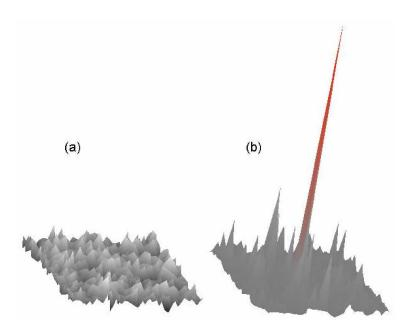
Figure 3.12. Three dimensional plot representing results of a cross correlation calculation: (a) only noise: (b) correlation peak
