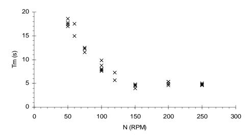
Figure 7.2. Experimental plot of mixing time versus agitator speed. The injection conditions were atmospheric pressure and an injection pipe diameter of 17.8 mm.
