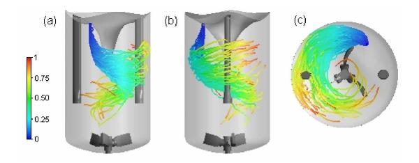
Figure 12.9. Jet injection on a deformed free-surface. Lagrangian jet trajectories coloured by the Lagrangian particle travel time normalized by  $T_{inj}$ , for d = 10 mm, V = 6 m s<sup>-1</sup> and N = 275 RPM, plotted at  $T_{inj}$  with 200 particles. (a) XY lateral; (b) YZ lateral view; (c) top view.
