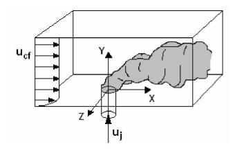
Figure 11.2. Schematic of a jet in a cross-flow.
