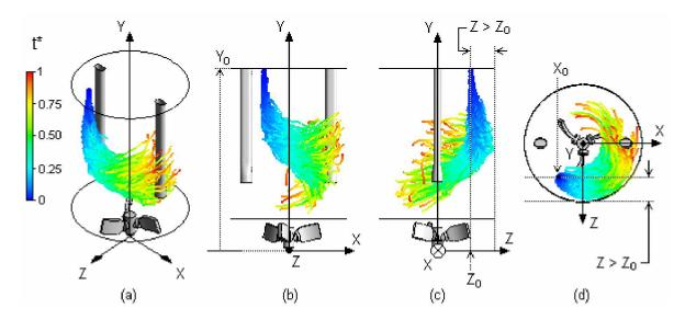
Figure 11.1. Details of the coordinate system: (a) 3D view; (b) XY lateral view; (c) YZ lateral view; (d) XZ top view.
