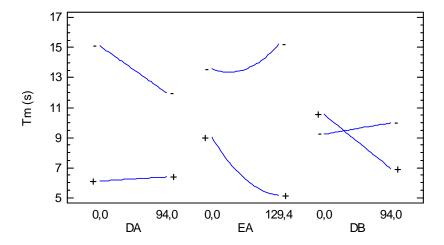
Figure 7.15. DA, EA and DB interaction plots. Abscissa shows the variation of the first letter of the plotted interaction. (+): higher level of the factor; (-): lower level of the factor.
