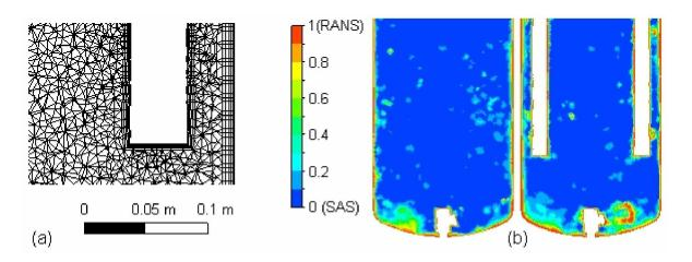
Figure 12.1. (a) details of the mesh used in the SAS simulations around the bottom tip of the right baffle; (b) RANS-SAS blending function on the vertical orthogonal baffle plane and on the baffle plane.
