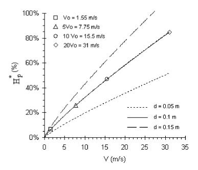
Figure 11.14. Variation of the dimensionless jet penetration depth with the jet velocity and the jet diameter for N =  $N_{\text{nom}}/2$  (industrial reactor).
