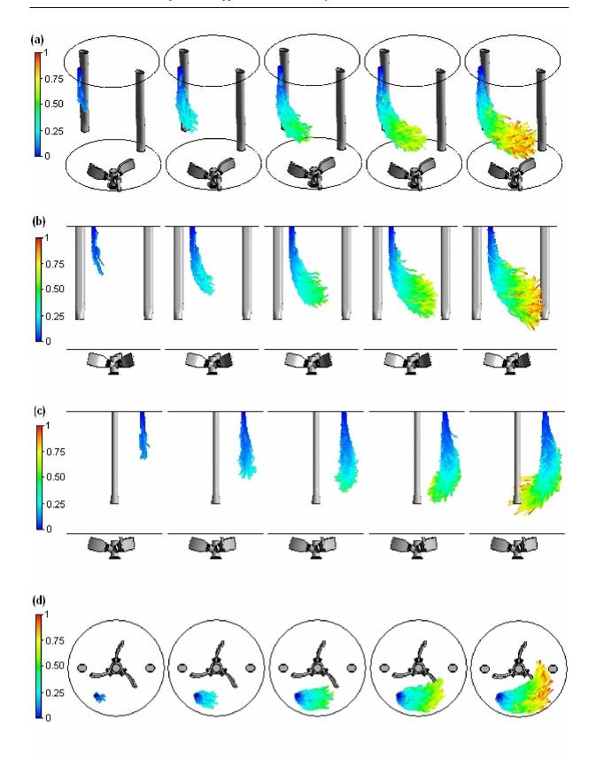
Figure 10.5. Lagrangian jet trajectories coloured by the Lagrangian particle travel time normalized by  $T_{inj}$ , for d = 0.1 m, V =  $10V_o$  = 15.5 m s<sup>-1</sup> and Re =  $2.5\times10^6$ , plotted at  $0.2T_{inj}$ ,  $0.4T_{inj}$ ,  $0.6T_{inj}$ ,  $0.8T_{inj}$  and  $T_{inj}$ . (a) 3D view; (b) XY lateral view; (c) YZ lateral view; (d) top view.
