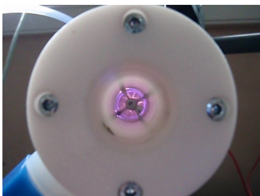
(e) U_{eff} = 5.5 \text{ kV} - f = 98 \text{ kHz}
