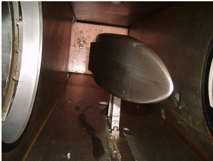
Figure 4.13: Installation of the forebody for oil-flow visualization.
