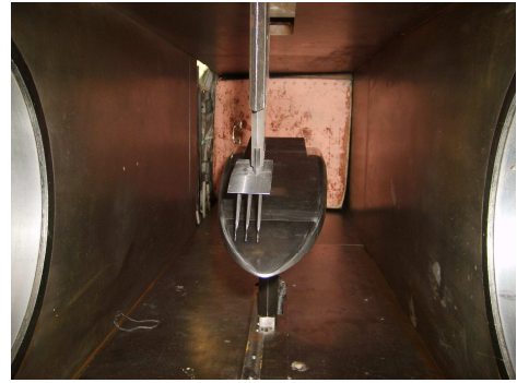
Figure 4.10: Installation of the forebody and the rake in T-313.
