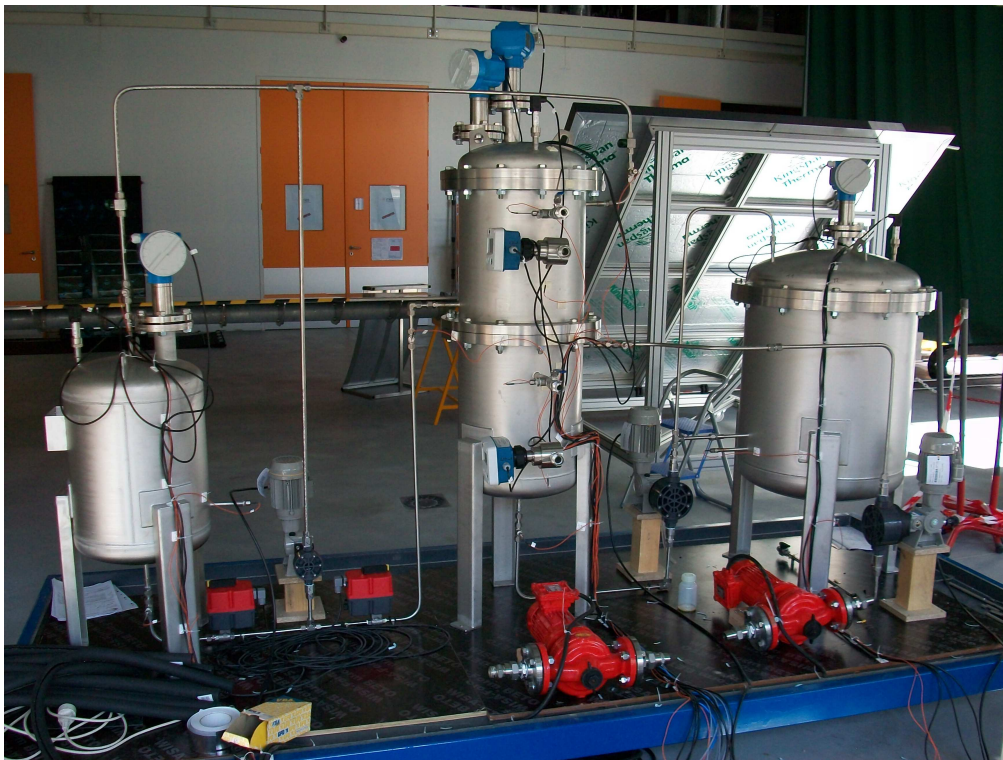
Figure 3-5 Experimental setup of the absorption storage system
