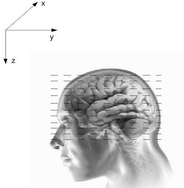
Figure 2.5: Slice by slice acquisition in MRI.
