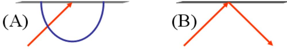
**Figure 3.3:** (A). Scattering at the totally rough surface ( $p = 0$ ). (B). Scattering at perfectly smooth surface ( $p = 1$ ).
