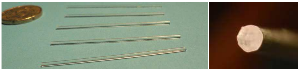
Figure 2.12 : fibres cristallines Nd :YAG [Fybercryst]
