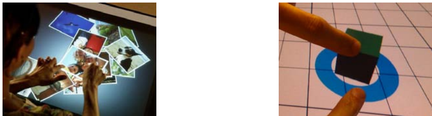
Fig. 2.9: RST technique for manipulation of photos on the Microsoft Surface ( left ). The same technique with a 3D visualization may cause occlusion problems ( right ).
