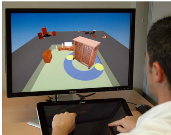
Fig. 2.12: Indirect control of the RST technique in a 3D furniture manipulation scenario.
