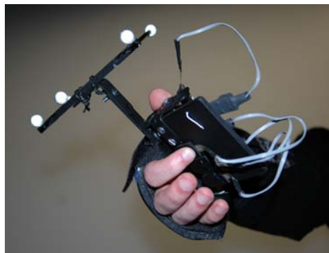
Fig. 3.3: The Piivert device. Tracking is operated by infrared vision. Force Sensitive Resistors allows fine excitation from finger gestures.
