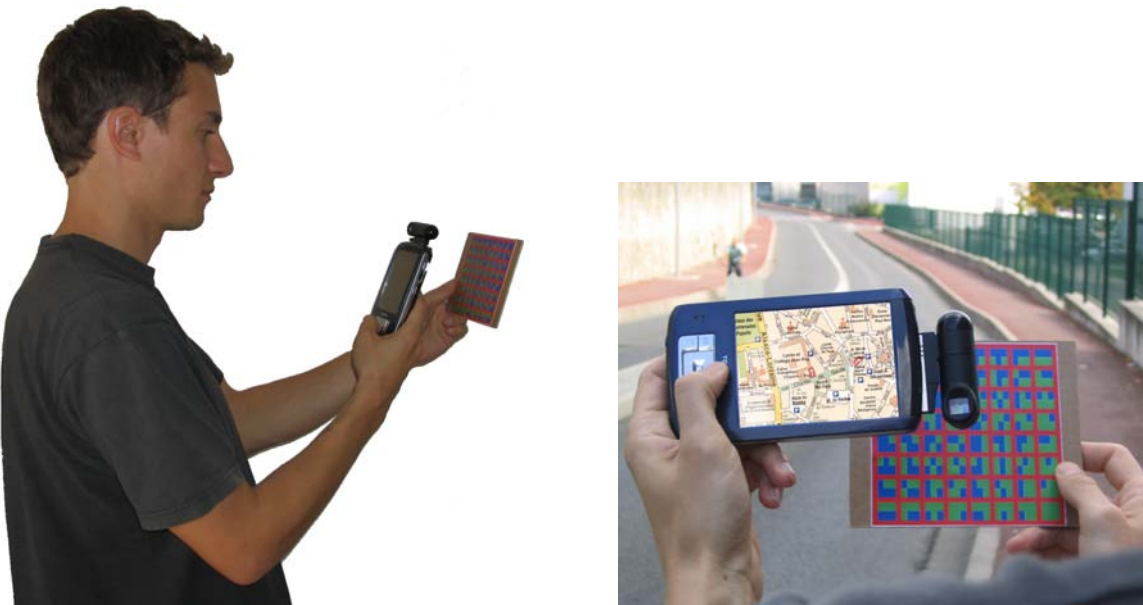
Fig. 1.10: Tangimap. By moving a target with his dominant hand, the user controls 3 DOFs for interaction with large documents or 3D environments.
