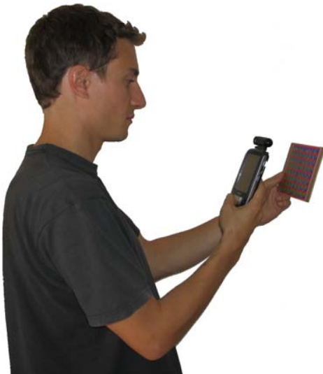
Figure 2: The camera of the handheld computer films the movements of a target behind the screen.
