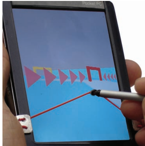
Fig. 1.5: A simple rubber band adds elastic feedback to pen input on a PDA.
