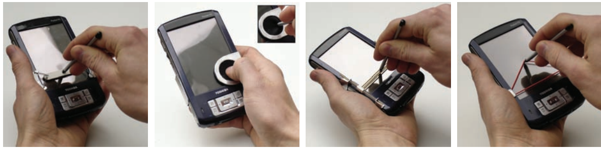
(a) Elastic pen insertion with small movement deviation. (b) Elastic feedback system made of elastic fabric to be used with pen or thumb. (c) Semi-elastic pen insertion, providing constrained isotonic input for one degree of freedom, while offering elastic feedback to the other. (d) Semi-elastic pen insertion as in (c), but providing constraints to the elastic degree of freedom in relation to induced input with isotonic movement.
