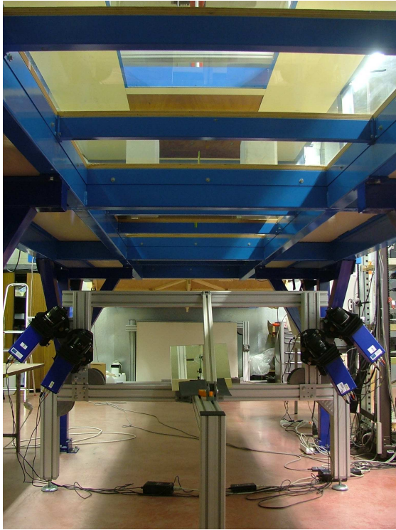
Figure 4.2: Side view of the stereo-PIV setup in the XY configuration (LML)
