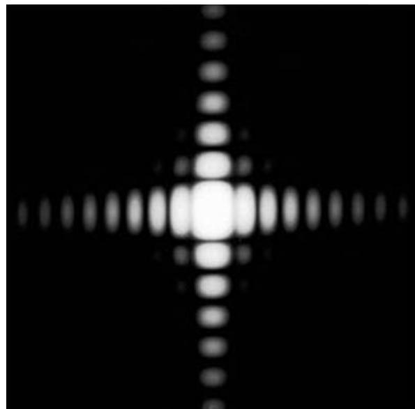
Figure 1.4: Diffraction pattern from a rectangular aperture.
