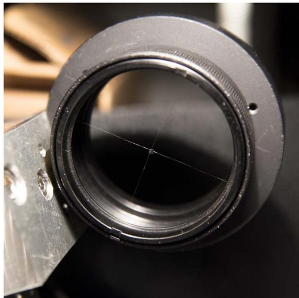
Figure 3.12: Order 0 mask used to eliminate order 0.
