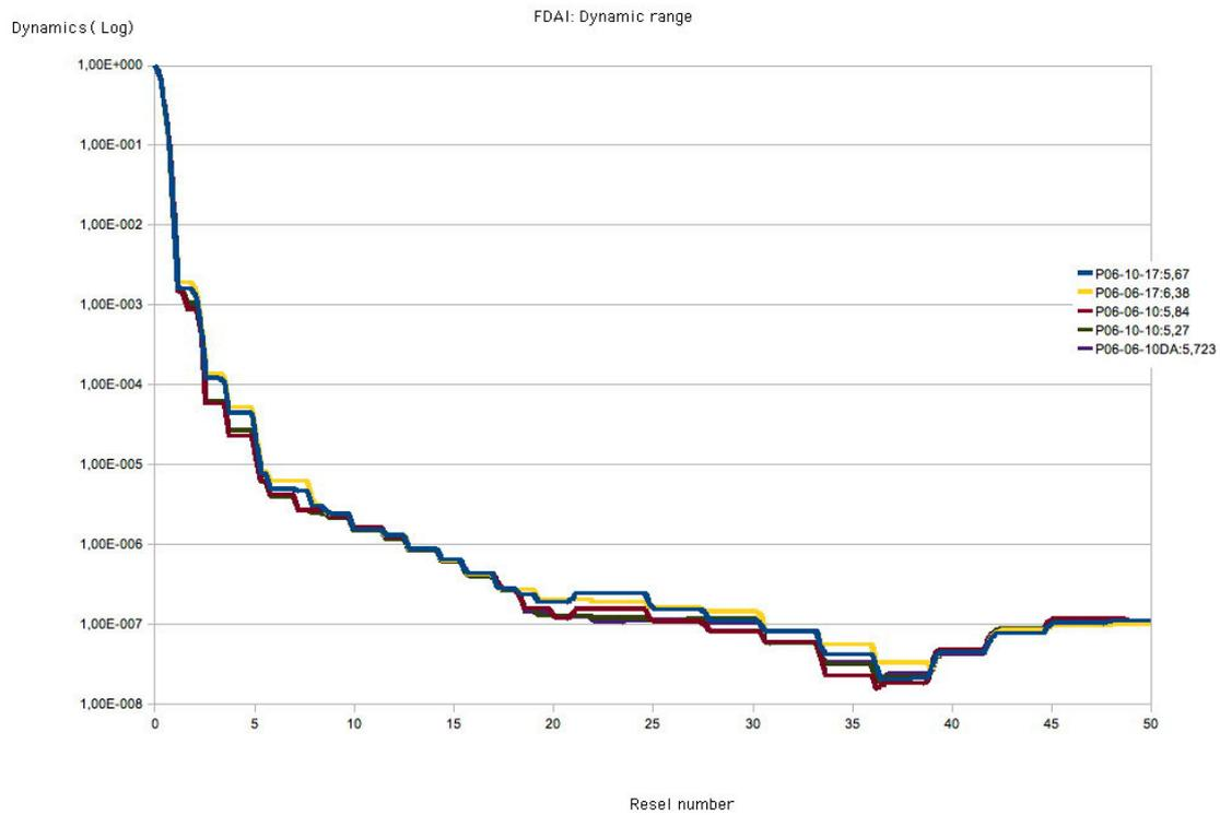
Figure 3.10: Dynamic range from arrays with different apodization parameters and different bar widths. The last numbers on the middle right of the figure correspond to the overall efficiency into order one(5.67, 6.38). The best curve is the red one at 6% bar width and  $a_0 = 0.10$ . The profile in the bottom is double cosine function.
