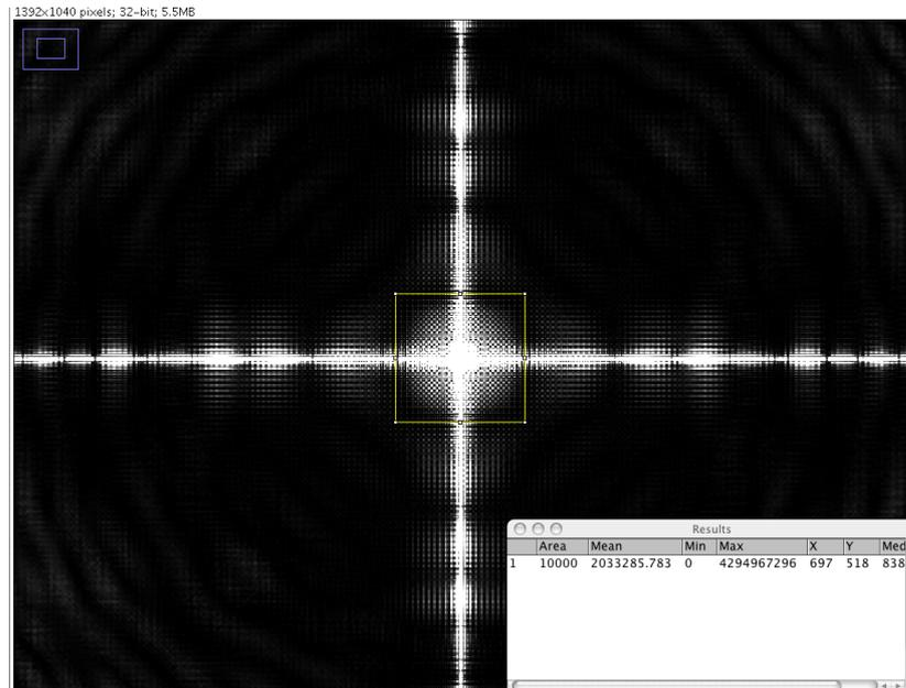
Figure 2.5: Central lobe measurement on the image obtained by Fresnel imager simulator for dynamic range determination. (Image contrast has been enhanced to display the faint levels of the PSF)
