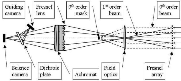
**Fig. 7** The optical scheme of the Generation 2 Fresnel imager (not to scale). The light beam from the zero order of diffraction is represented by dashed lines, whereas solid lines are used for the first order beam.
