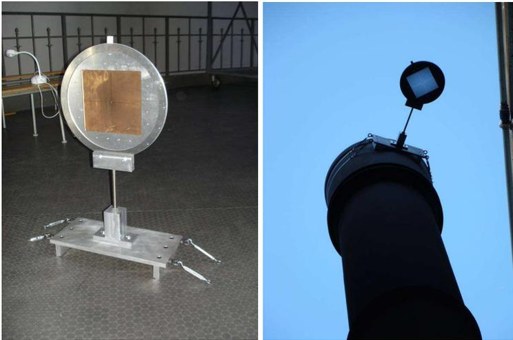
**Fig. 4** *Left: the Fresnel array module on its mechanical stand. Right: the same module, mounted on the refractor's tube. The orientation of the square aperture (hence of its PSF spikes) can be adjusted by rotating the cell holding it. The cell has been rotated by  $45^\circ$  between the two figures.*
