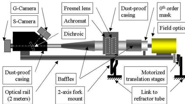
**Fig. 8** The setup of the Generation 2 Fresnel imager (not to scale). The 45 mm field stop (not represented) is located immediately upstream of the field optics (a Maksutov telescope).
