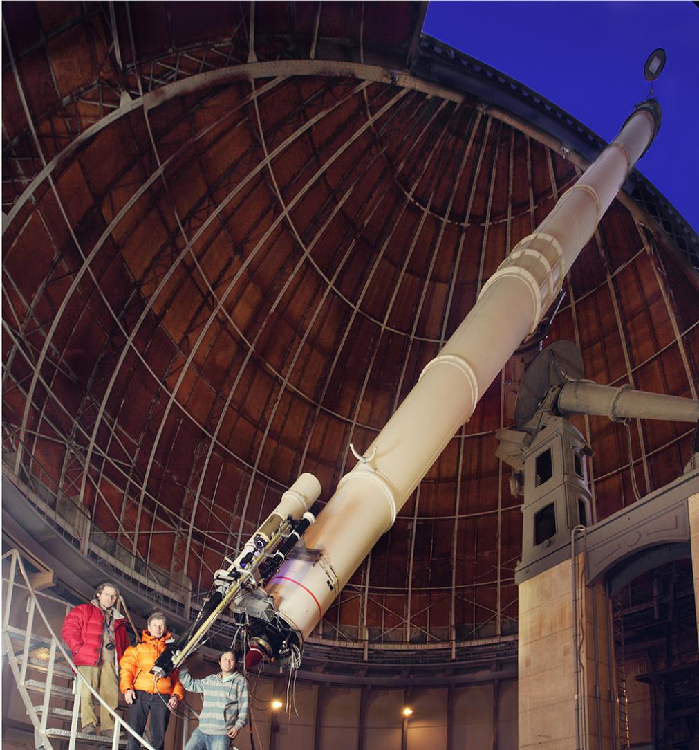
Figure 1. Fresnel generation II tested on the side of the 18 meter refractor at Observatoire de Nice. The 20 cm square Fresnel array is attached to the front end, the receptor module is the thin steerable optical bench at the rear end. The optical axis of the Fresnel imager runs in free air outside the refractor tube.
