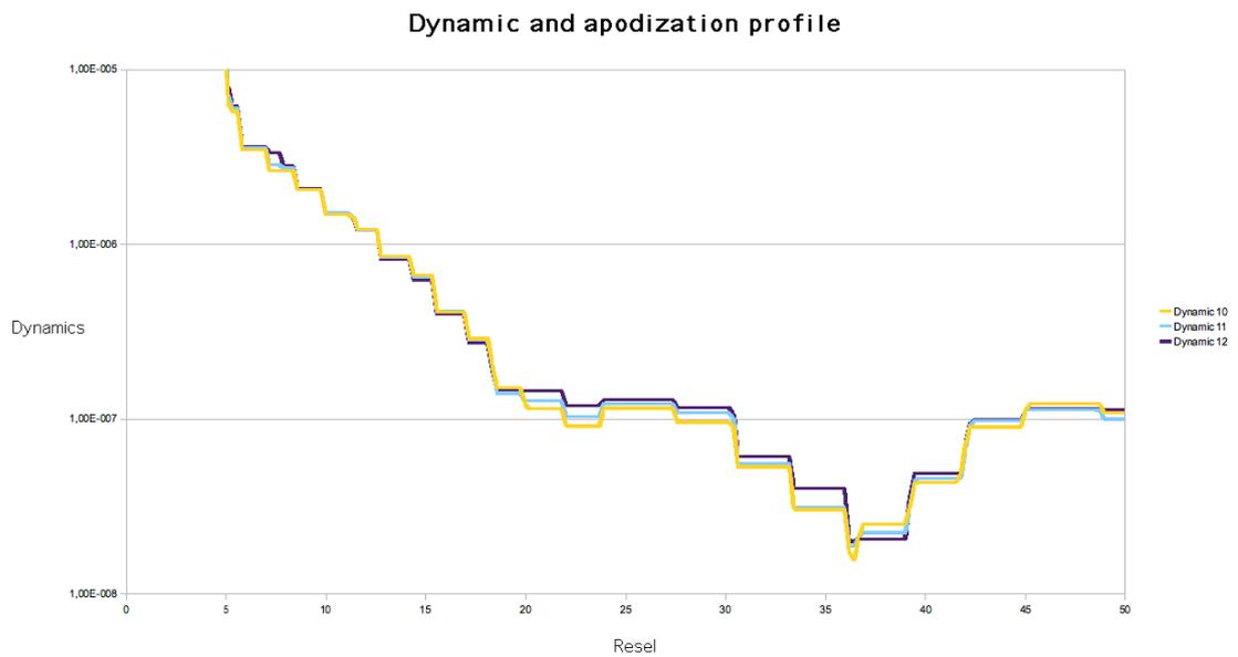
Figure 3.11: Comparison of dynamic range curves with different values of edge transmission( $a_0$ ).
