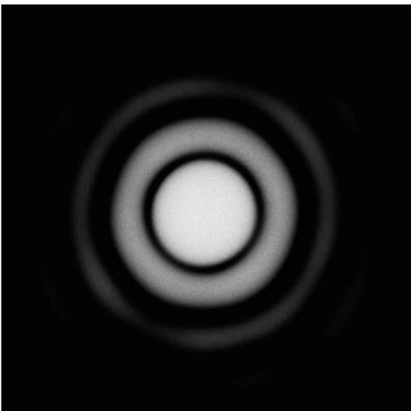
Figure 1.3: Diffraction pattern from a circular aperture
