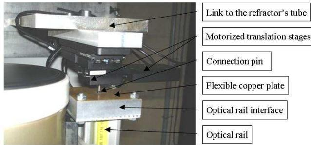
**Fig. 6** The crossed  $XY$  translator stages connecting the optical rail of the receiver module to the refractor's tube. Since the optical rail is on a fork mount, the  $XY$  translation stages acting on its upper end, modify the orientation of the whole receiver module with respect to the Fresnel array module. The fine tuning of the chromatic correction is obtained by electrically controlling these translation stages.
