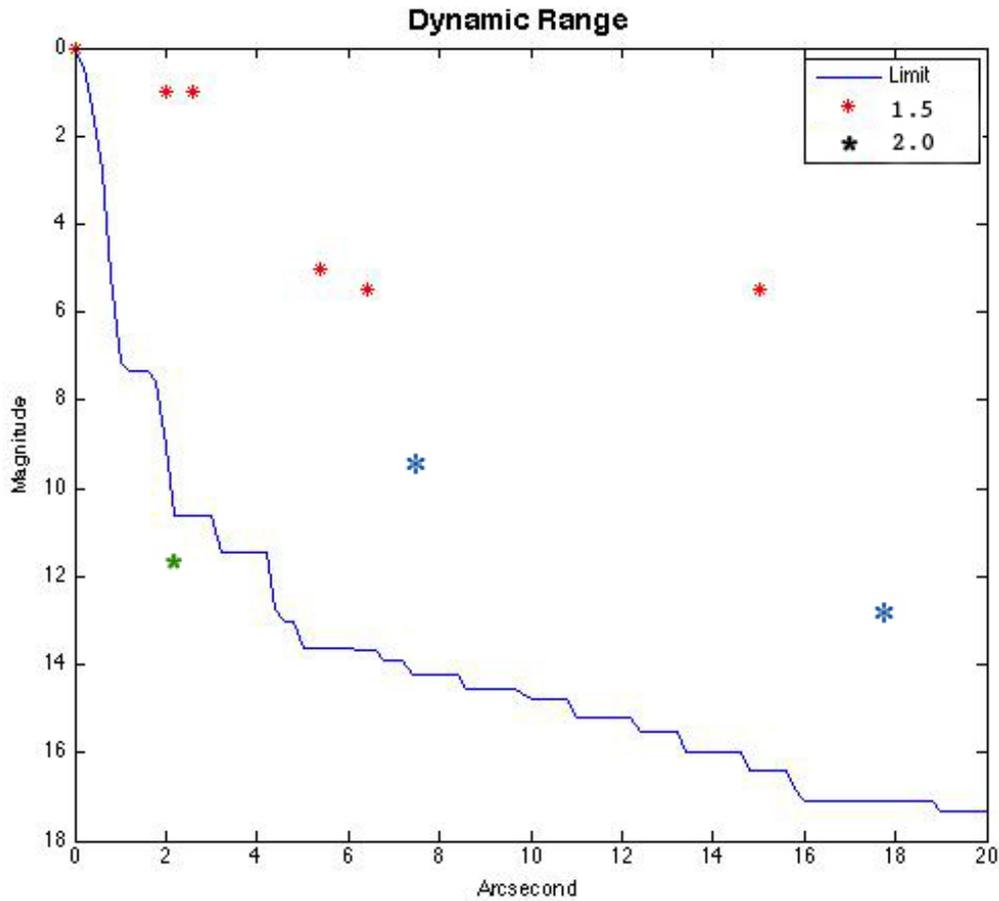
Figure 5.2: The curve corresponds to the limiting magnitude difference as a function of the angular separation. It is obtained from the PSF of the Fresnel Imager, compared to observed results from prototypes 1.5.1 and 1.5.2 and 2.0. The *red* stars are results from prototype generation 1.5.1 and 1.5.2. The results from a complete prototype generation 2 are shown as the *blue* stars. The green one below the curve is Procyon, for which the companion is not detected.
