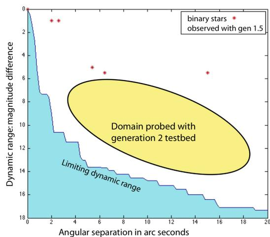
**Fig. 8** Separation versus contrast diagram. The star markers represent the couples actually studied with the Generation 1.5.1 and 1.5.2 testbeds. The continuous curve is the theoretical limit, and the ovale shaded shape sketches the expected region of action of the full generation 2 testbed.
