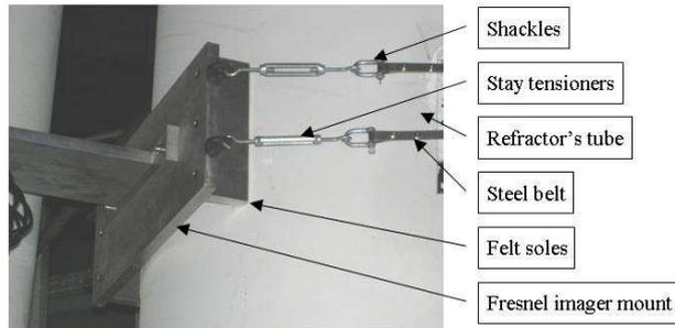
**Fig. 3** *Non-destructive mounting system. The mount is fastened to the refractor's tube by two stainless steel belts, the tension of which is adjusted with four stay tensioners. The felt soles prevent damage of the refractor's coating.*
