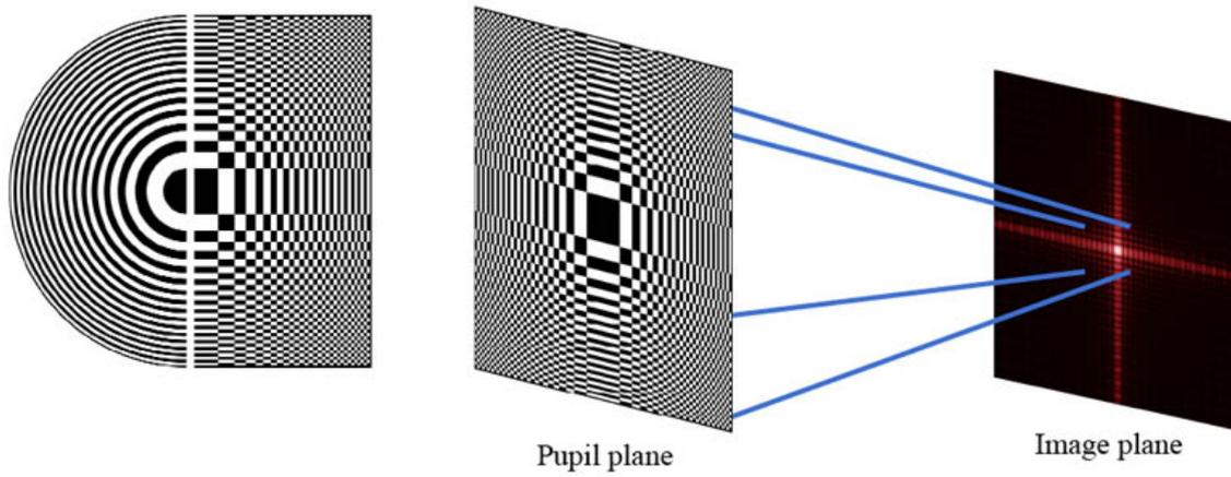
Figure 1.8: Left : circular-orthogonal comparative designs, Right : The image given from a point source, Point-Spread-Function (PSF)
