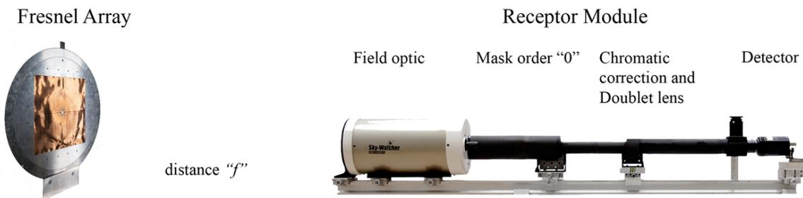
Figure 1.9: Fresnel Imager System contains Fresnel Array module and Receptor module.
