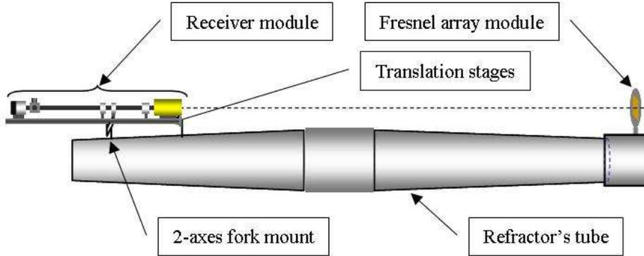
**Fig. 2** The global structure of the instrument (not to scale). The refractor's tube is 19 m long, and the optical rail is 2 m long. The optical axes of the refractor and of the Fresnel imager are parallel.
