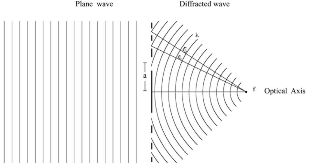
Figure 1.5: A plane wave propagates through the apertures in Fresnel zones. The optical paths ( $E_1$  and  $E_2$ ) difference between two Fresnel zones is  $\lambda$ . The diffracted light by arrays aperture converges to a focal point ( $f$ )
