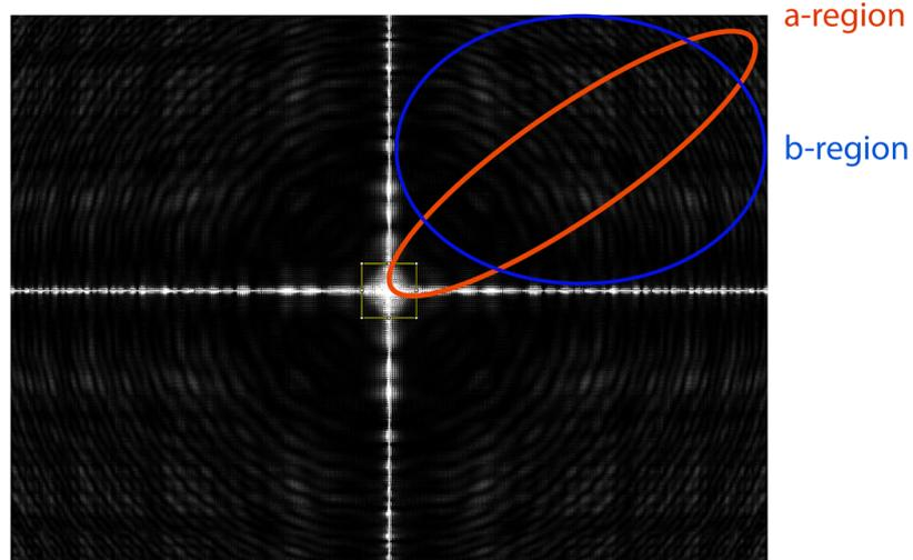
Figure 2.3: PSF obtained by numerical simulation. Our new Fresnel Design (Orthogonal transformation) extends the contrast between central lobe and background level in quadrants, as *b* region. The areas where the contrast is sampled for dynamic range assessment are in the *a* region.
