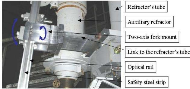
**Fig. 5** The two-axes fork mount connecting the receiver module to the refractor's tube. The foot of the fork mount is tightly bolted on an existing structure of the refractor (the sole of a former auxiliary finder).
