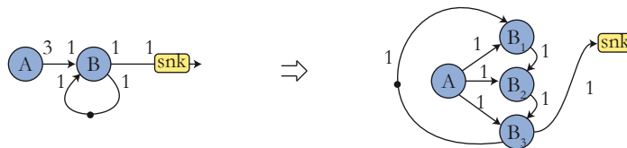
Figure 3.9: IBSDF Sub-Graph Example and Its Single Rate Equivalent
