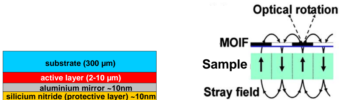
Fig. 2.22 (left): schematic diagram of the MOIF structure (not to scale); (right): scheme of magneto-optic imaging with a MOIF.
