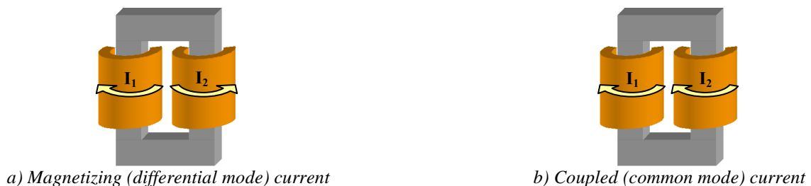
Figure III.4: Current directions when simulating coupled and magnetizing currents.
