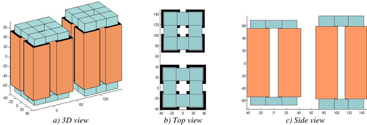
Figure IV.21: Final shape of optimized ICTs with different conductor material (scale in millimeters).
