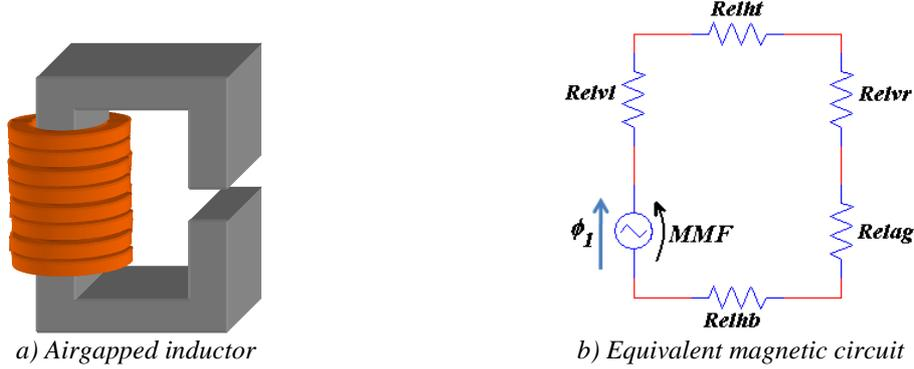
Figure I.10: Inductor and its magnetic circuit.
