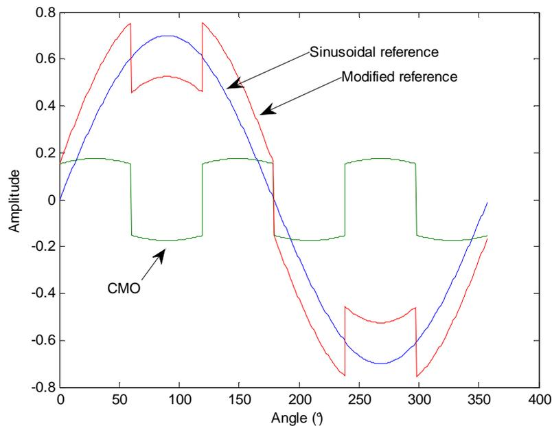
Figure V.36: Modulation waveforms of PWMBC method ( $M_i=0.7$ ).
