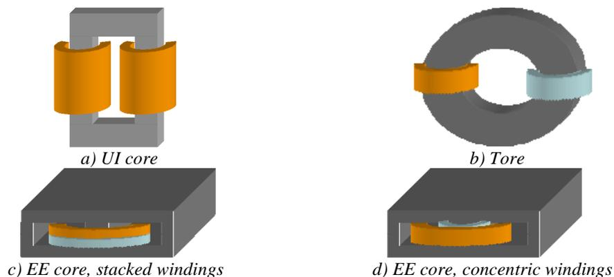
Figure III.2: Two-cell ICTs using different core shapes.
