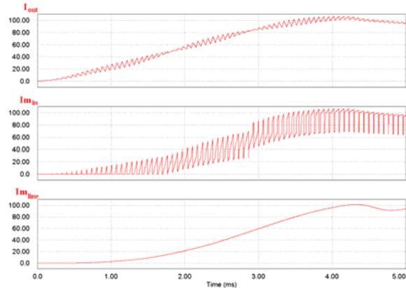
Figure I.4: Parallel multicell converter and filter waveforms ( $F_s=5\text{kHz}$ ).
