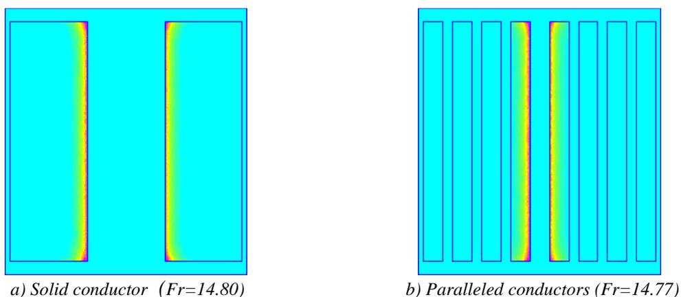
Figure II.29: Current density in solid and paralleled conductors.
