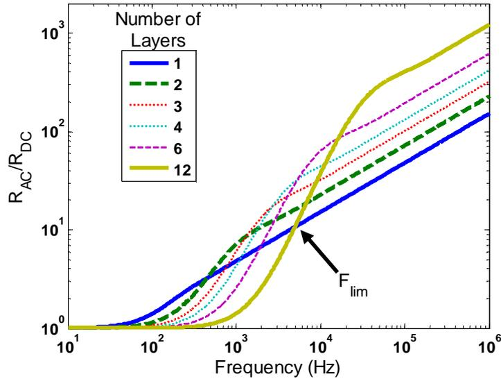
Figure II.33: Variation of the AC resistance with the frequency for each of the configurations of Figure II.32.
