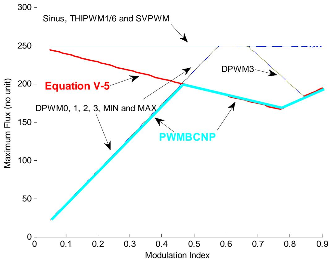
Figure V.24: Maximum flux ripple for different PWM methods.
