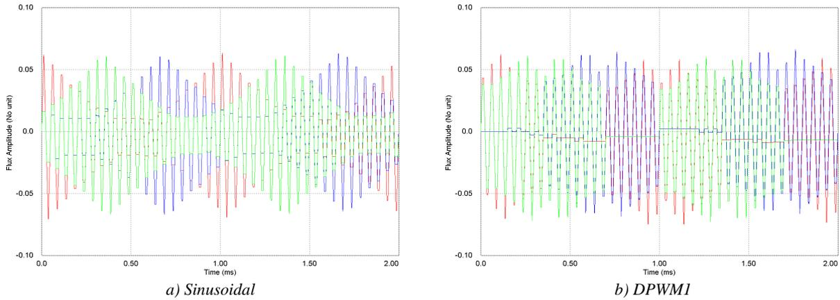
Figure V.12: ICT flux using DPWMI and SPWM techniques.
