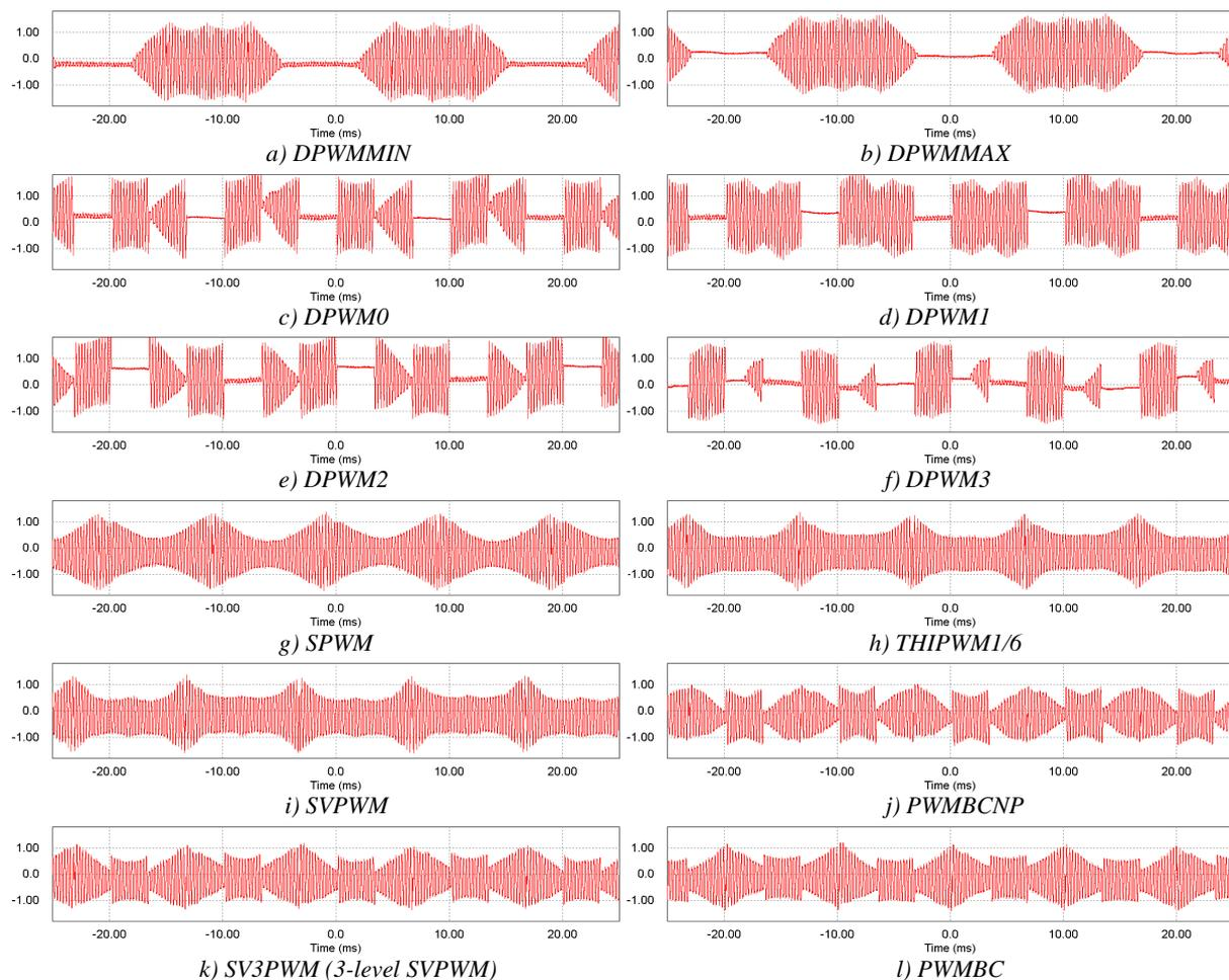
Figure V.49: Measured current differences for different methods.
