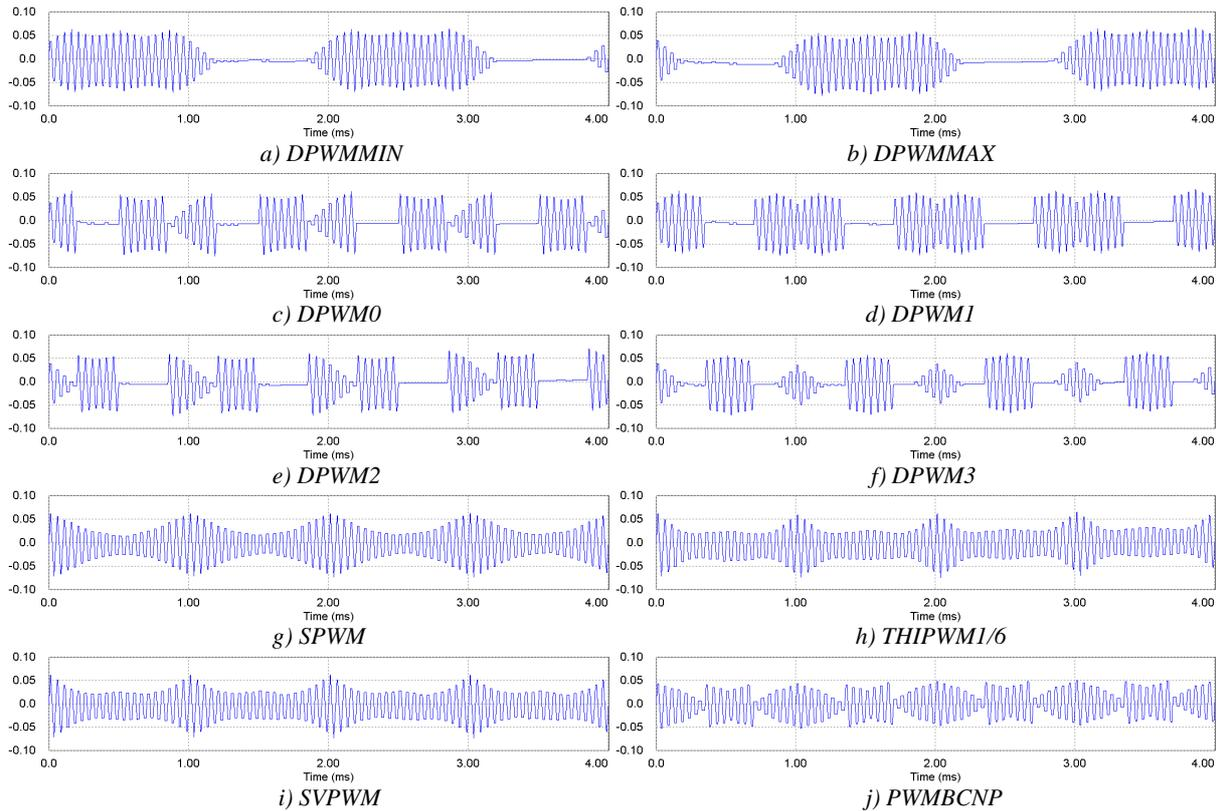
Figure V.25: ICT flux waveform for different PWM methods.
