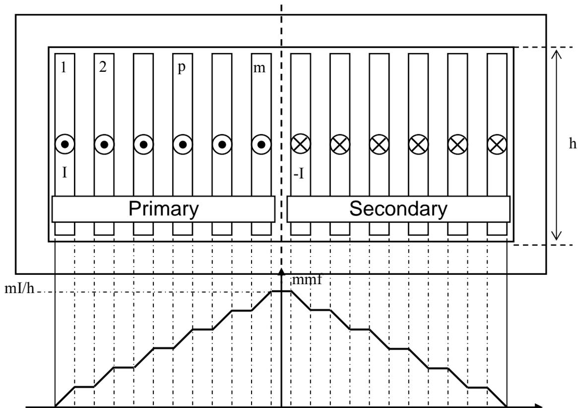
Figure II.8: Transformer parameters used to explain Dowell's formula.
