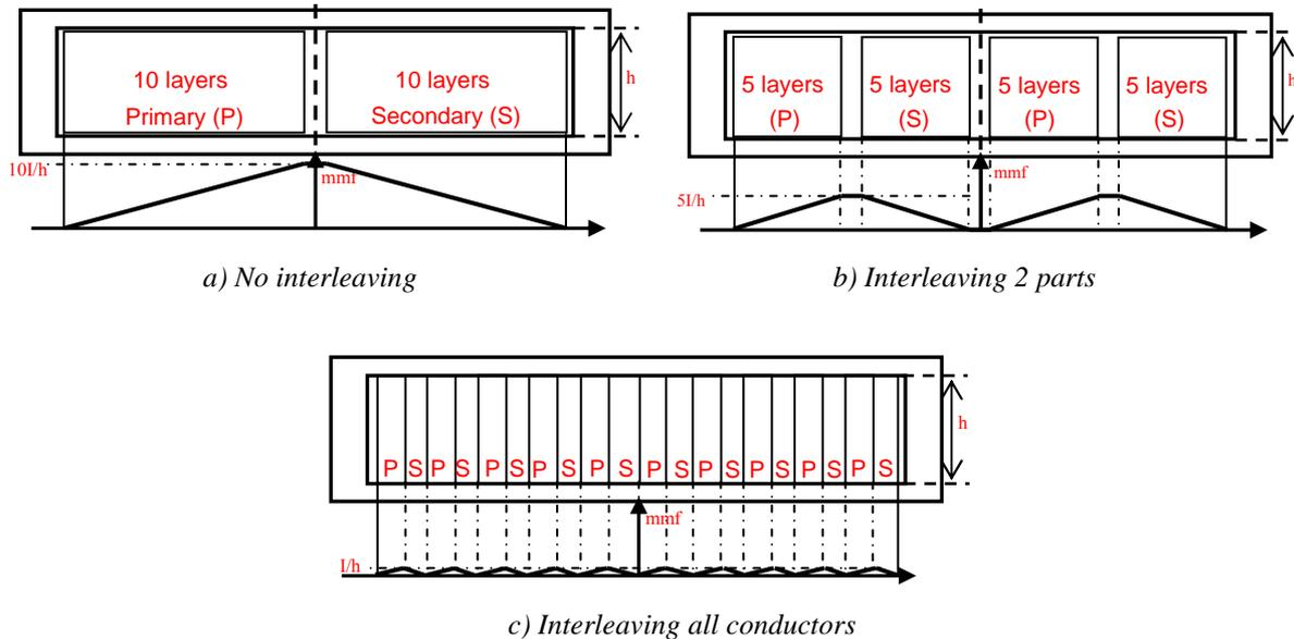
Figure II.26: Energy reduction by interleaving windings.
