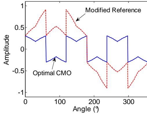
Figure V.17: Optimal CMO for high modulation indexes.
