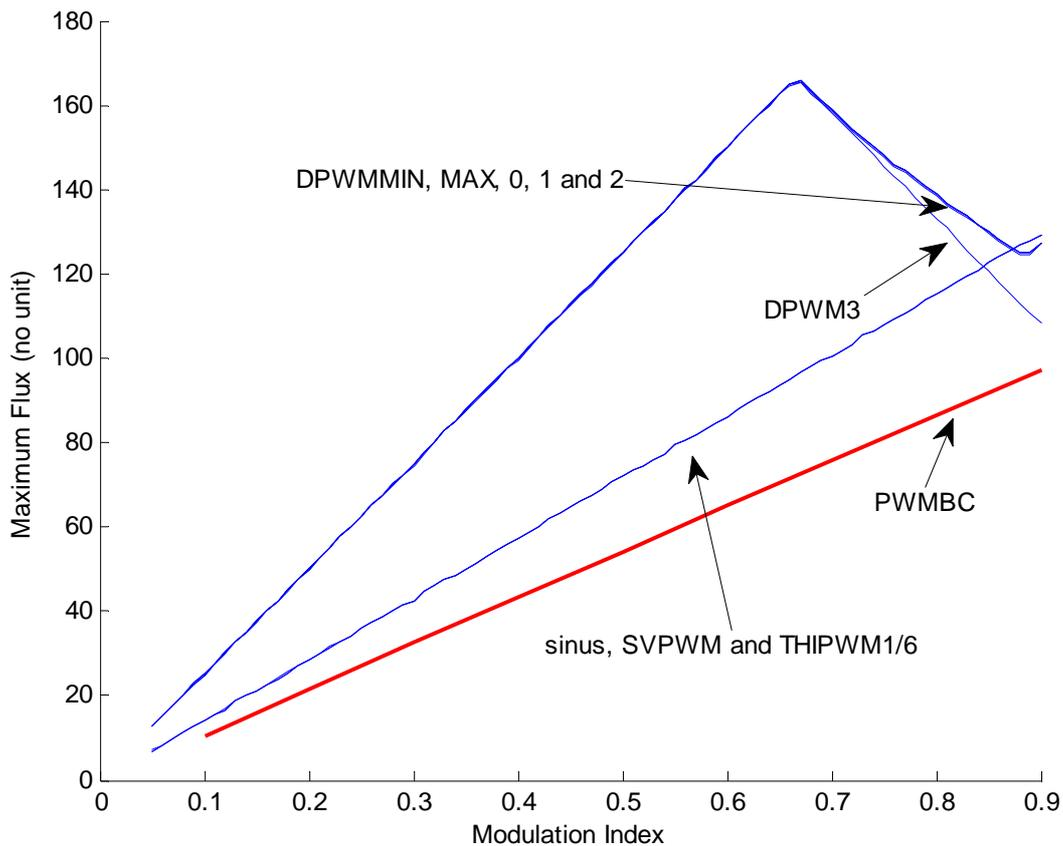
Figure V.40: Maximum flux ripple for different PWM methods.
