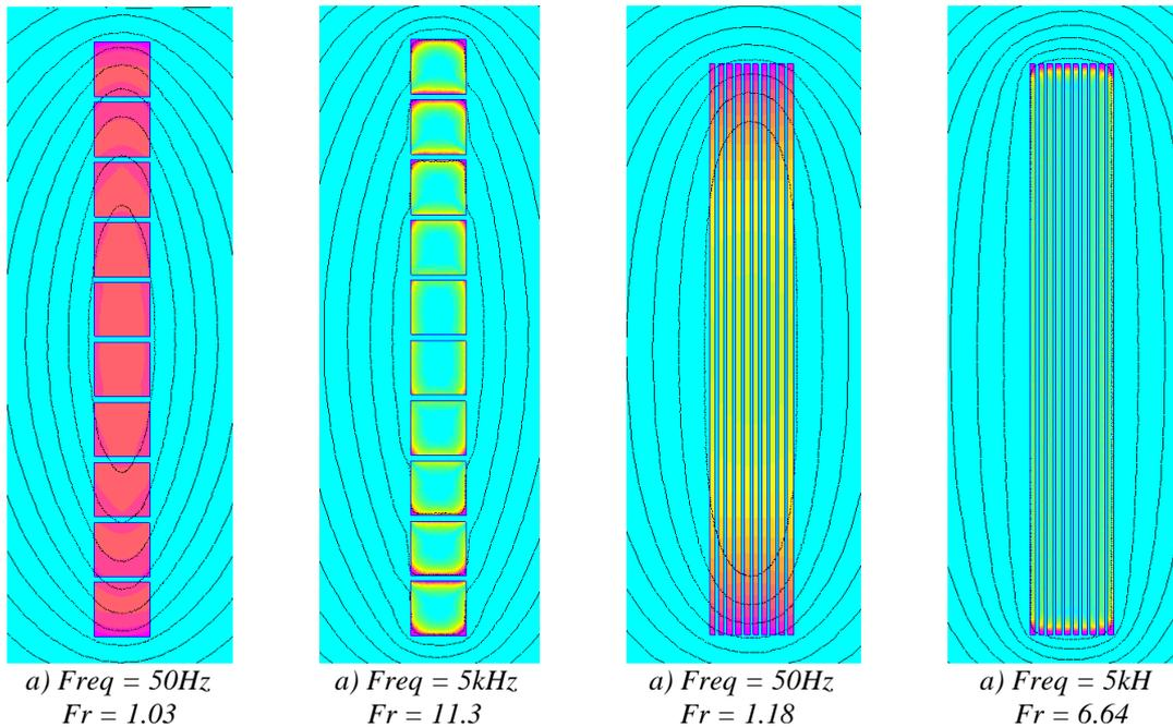
Figure III.7: FEMM simulation of conductors with different dimensions but with the same cross-section area, at two different frequencies (current density plot).
