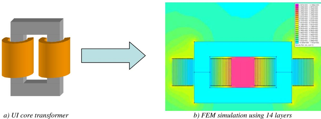
Figure II.17: Transformer and FEM simulation (magnetic field distribution).
