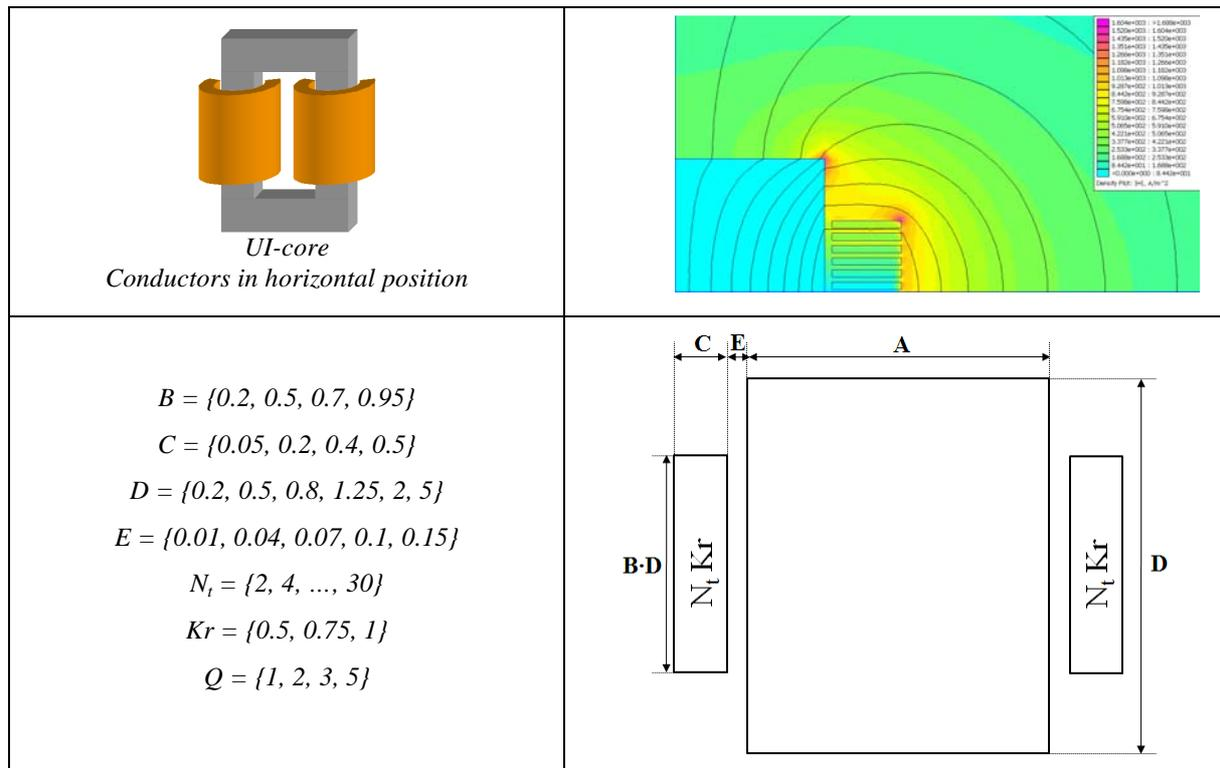
Figure IV.12: UI-core, conductors in horizontal position.
