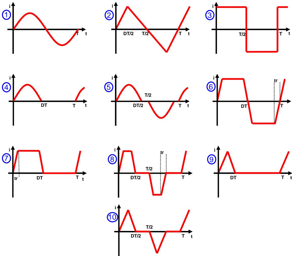
Figure II.42: Typical current waveforms found in switch-mode power supplies.
