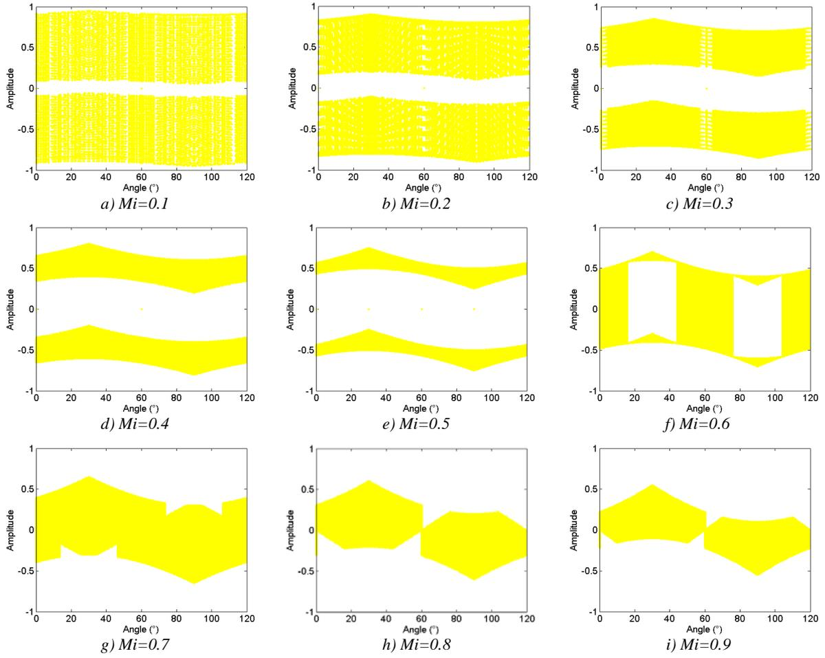
Figure V.42: Offsets where the maximum flux ripple is close to the minimum numerical solution (1%).
