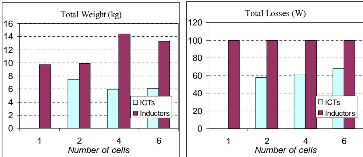
Figure IV.26: Comparison between ICTs and inductors for N-cell interleaved Buck converter.
