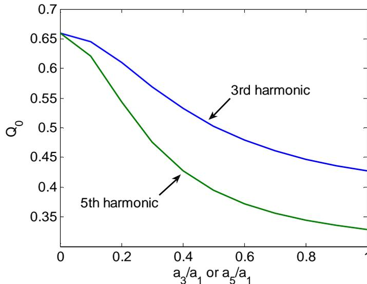
Figure II.39: Variation of  $Q_0$  with the amplitude of the 3<sup>rd</sup> and 5<sup>th</sup> harmonics.
