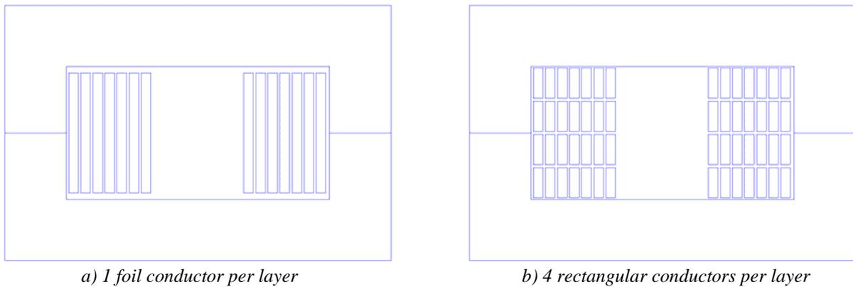
Figure II.11: Simulated structures.
