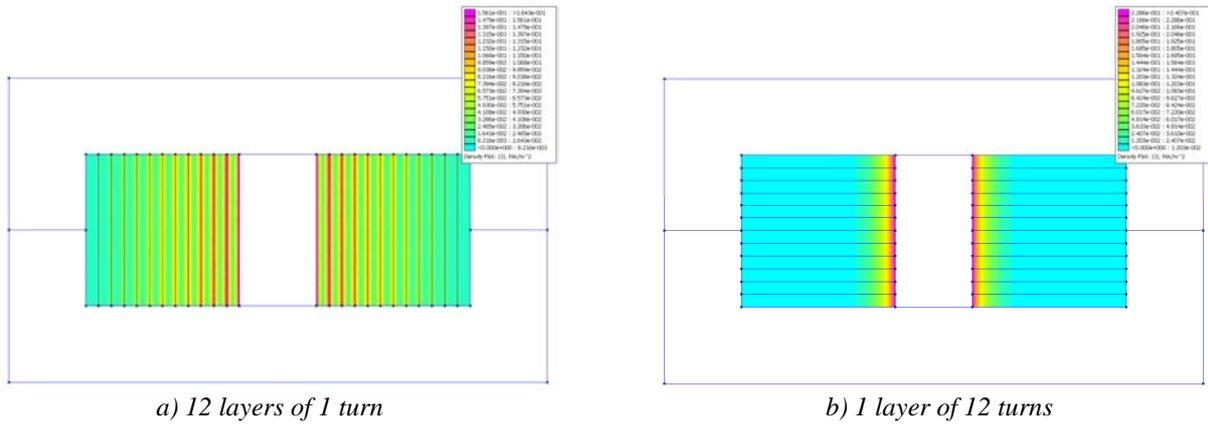
Figure II.37: Simulated transformers.
