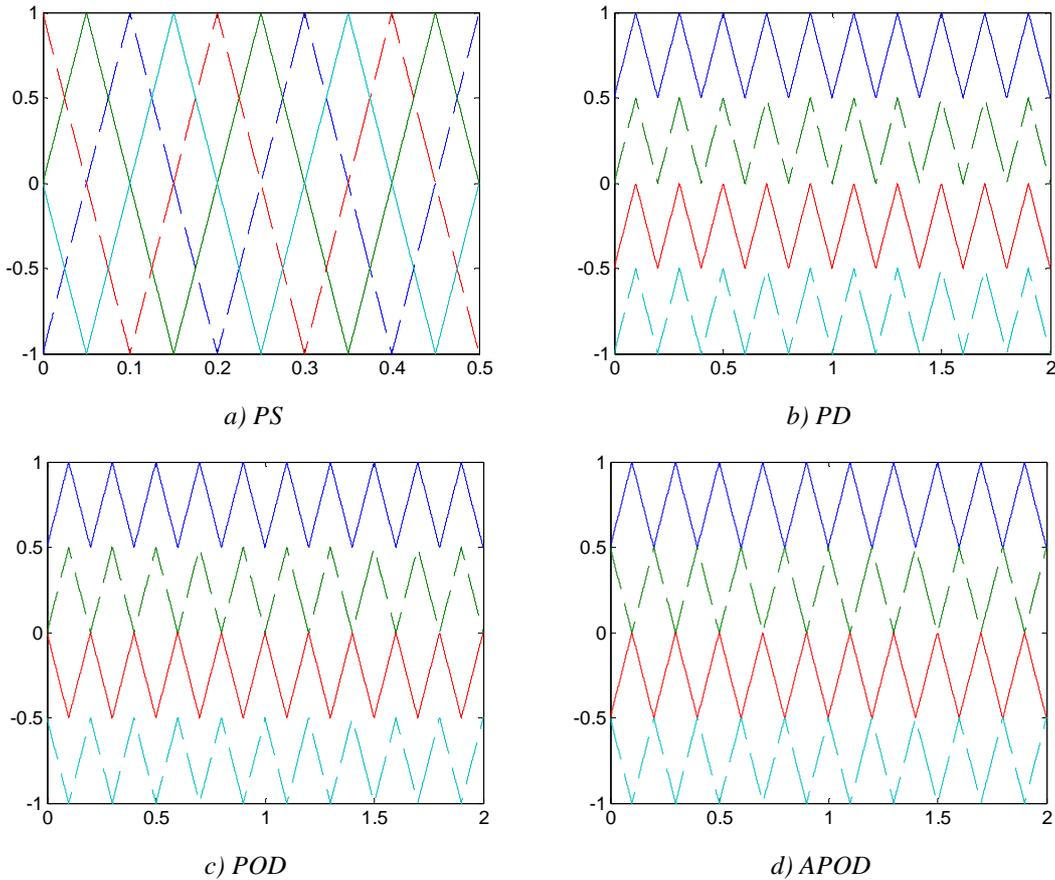
Figure V.4: Different carrier-based techniques for 5-level PWM.
