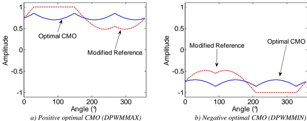
Figure V.15: Optimal CMOs for low modulation indexes.
