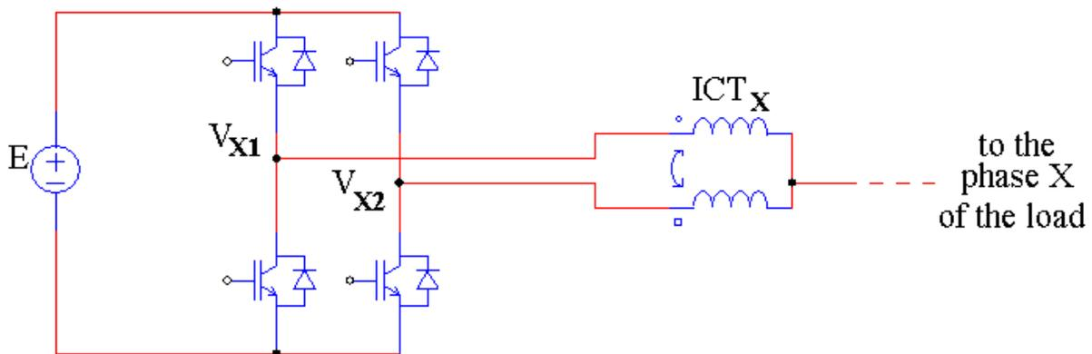
Figure V.5: One phase of the dual three-phase inverter coupled by one ICT.
