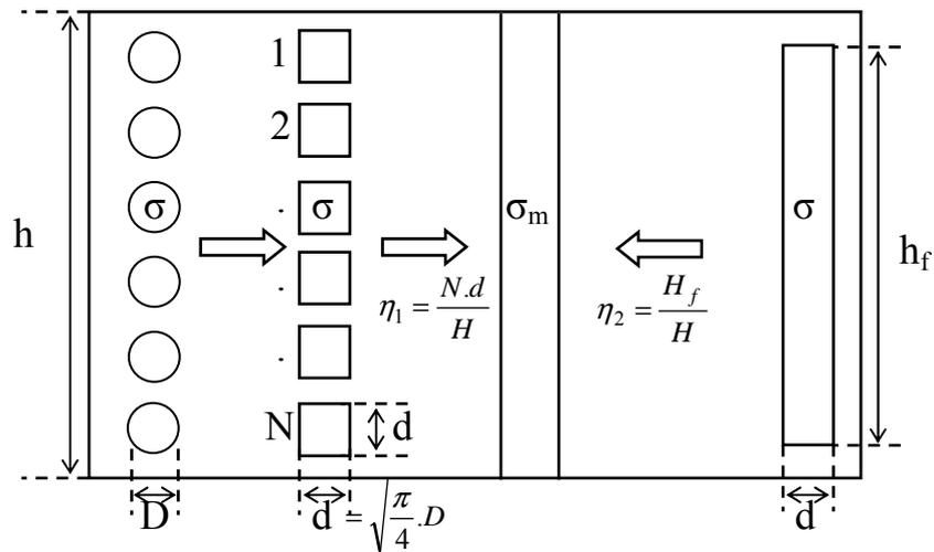
Figure II.10: Porosity factor definition for different conductor shapes.
