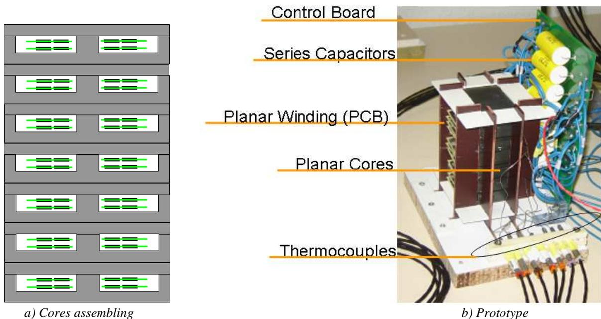
Figure III.32: “Basso Cambo” ICT built to evaluate core losses.
