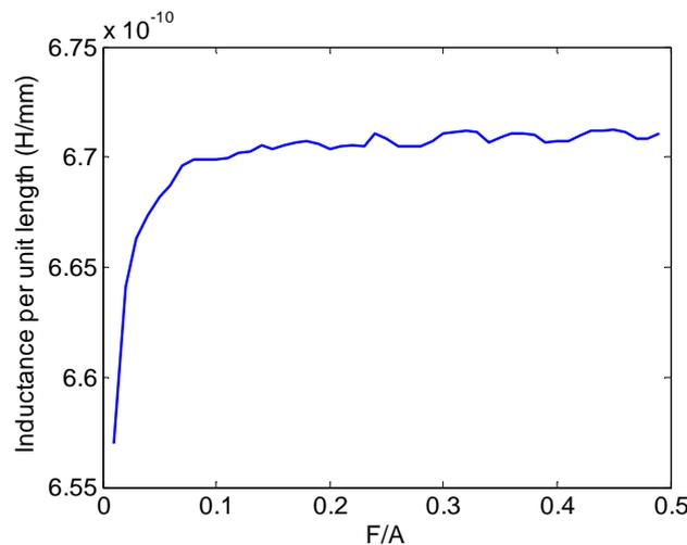
Figure IV.4: Variation of the leakage inductance per unit length with the core leg width.
