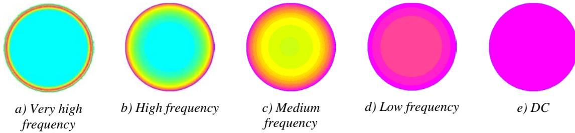
Figure II.2: Current distribution in conductors for different frequencies.
