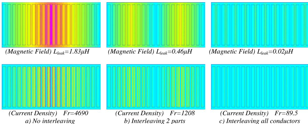
Figure II.27: Simulation of interleaved windings.
