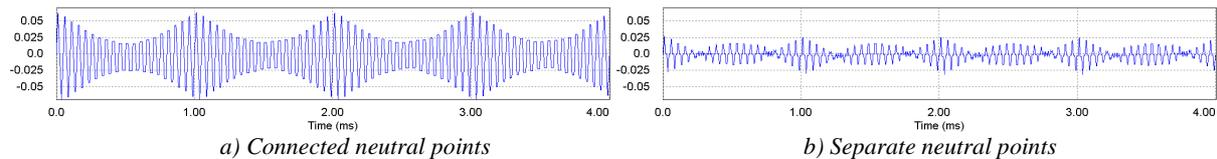
Figure V.29: Flux waveforms of the same circuit with and without neutral point connection ( $M_i=0.7$ ).
