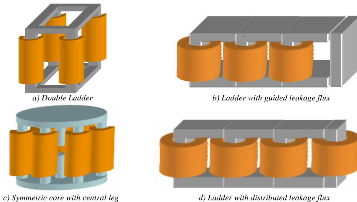
Figure III.26: Different topologies of monolithic InterCell Transformers.
