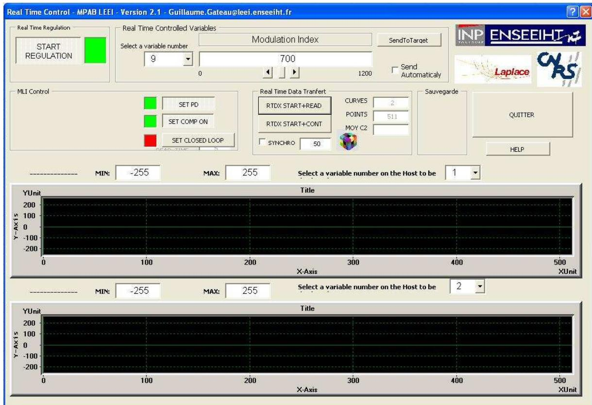
Figure V.48: User interface to control both three-phase inverters.
