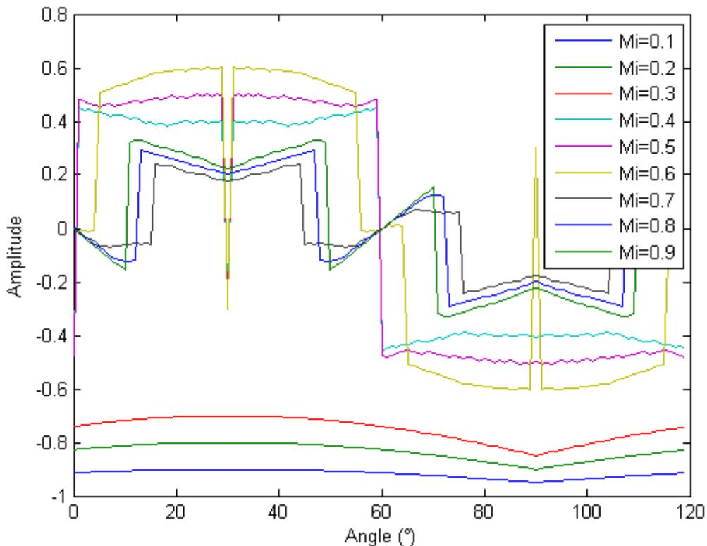
Figure V.22: Optimal CMO for 3 commutation cells per phase.
