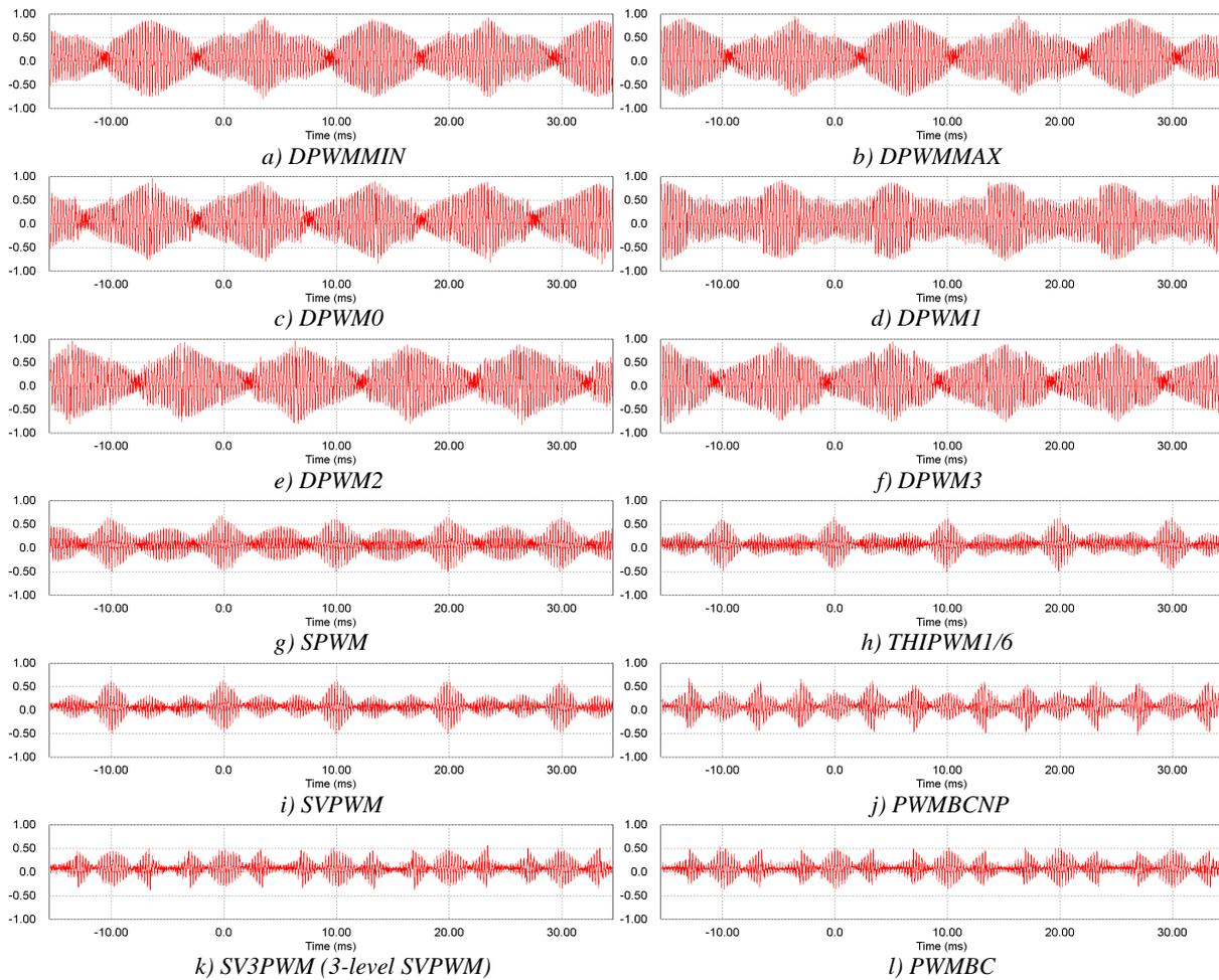
Figure V.51: Measured current differences for different PWM methods.
