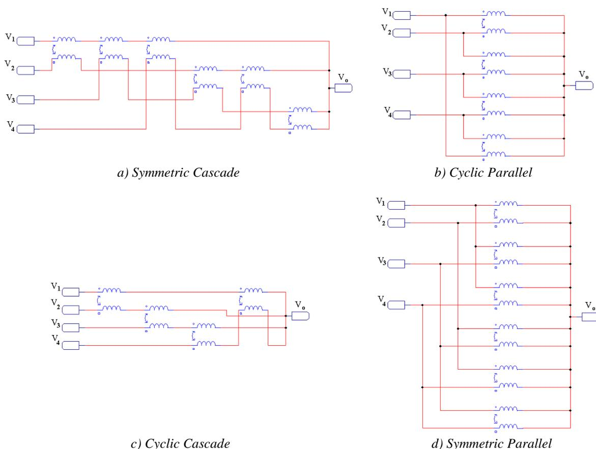
Figure I.17: 4-phase ICT topologies using separate 2-cell ICTs.
