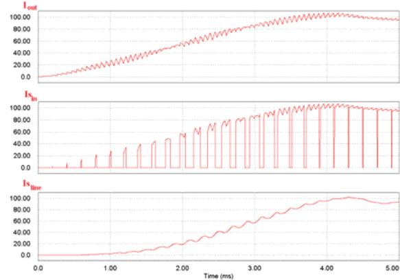
Figure I.3: Series multicell converter and filter waveforms ( $F_s=5\text{kHz}$ ).
