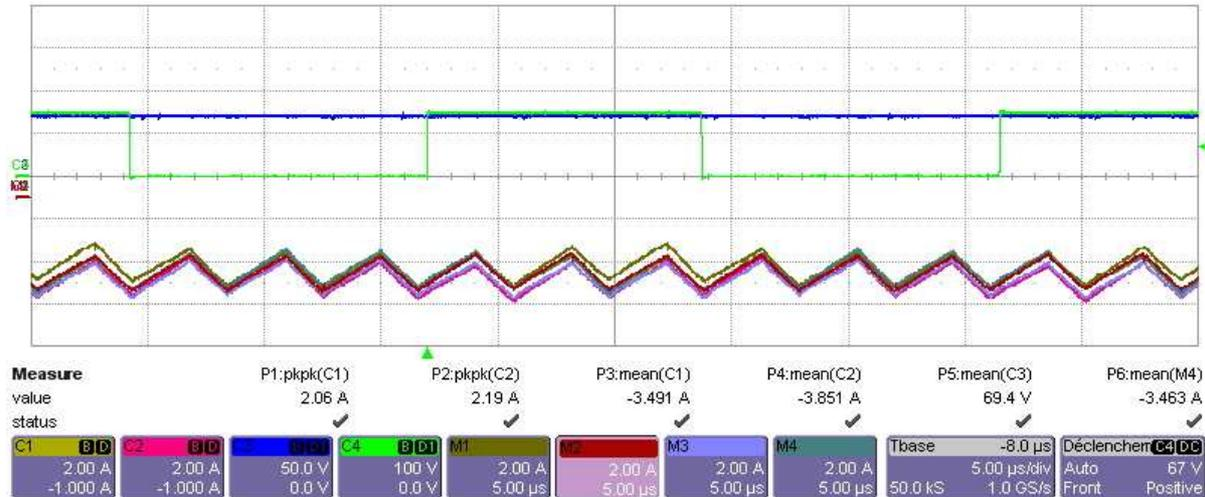
Figure III.35: Currents in the 6 commutation cells.
