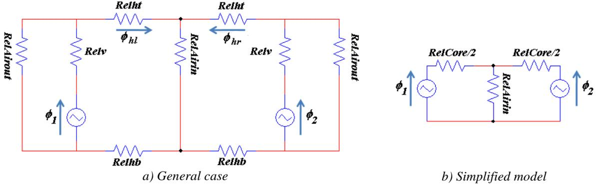
Figure III.16: Reluctance models of the ICT magnetic circuit.
