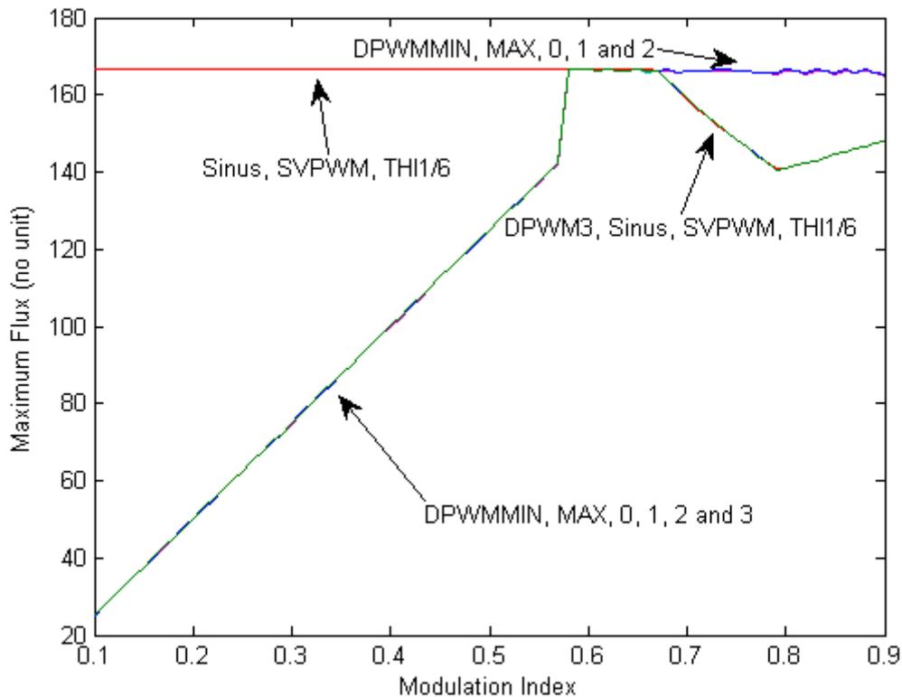
Figure V.44: Maximum flux ripple for different PWM methods.
