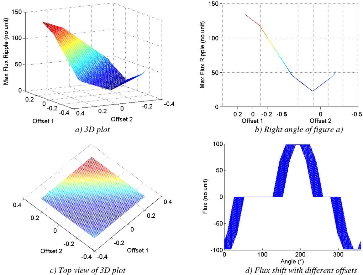
Figure V.39: Flux behavior when different offsets are applied to the dual three-phase converters. Angle =  $80^\circ$ ,  $M_i = 0.7$ , Offsets from  $-0.3$  to  $+0.3$ .
