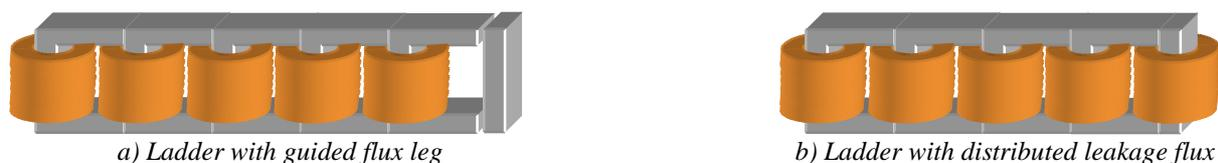
Figure I.13: Ladder InterCell Transformers.
