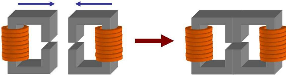
Figure IV.25: Joining two inductors to form an ICT.
