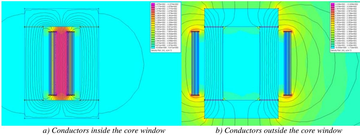
Figure III.14: FEMM simulation of the intercell transformer of Figure III.12 (magnetic field intensity).
