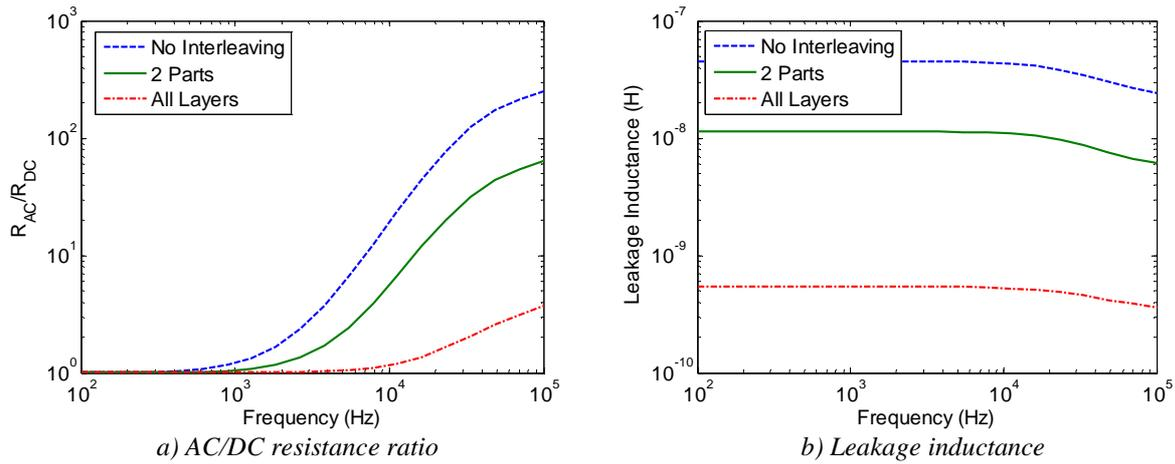
Figure II.28:  $Fr$  and leakage inductance reduction by interleaving windings.
