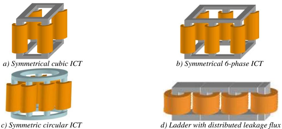
Figure IV.8: Different topologies of monolithic intercell transformer which may use the 4-dimensional matrix to speed up the optimization process.
