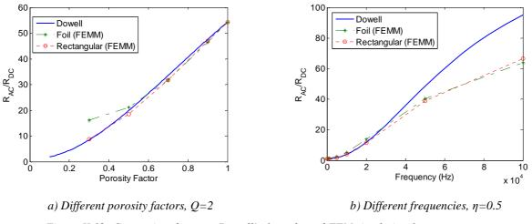
Figure II.12: Comparison between Dowell's formula and FEM simulation for two structures.
