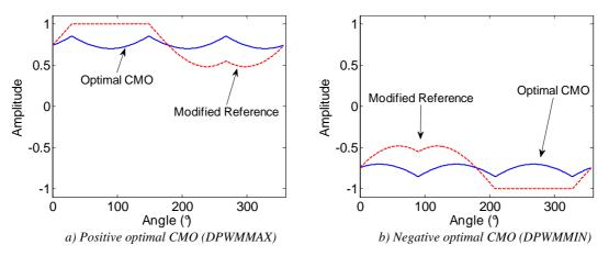
Figure V.15: Optimal CMOs for low modulation indexes.
