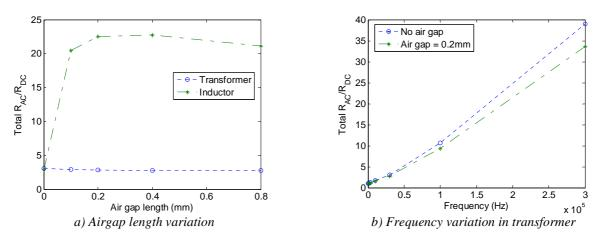
*Figure II.20: Influence of airgap in the AC/DC resistance ratio.*
