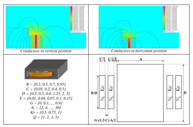
Figure IV.13: EE-core, concentric windings, conductors in horizontal and vertical positions.
