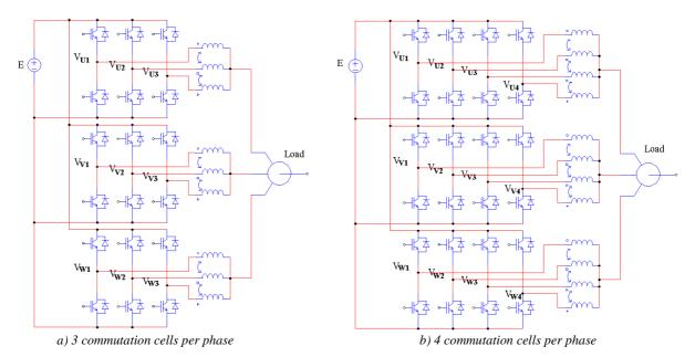
Figure V.20: System topologies with 3 and 4 commutation cells per phase.
