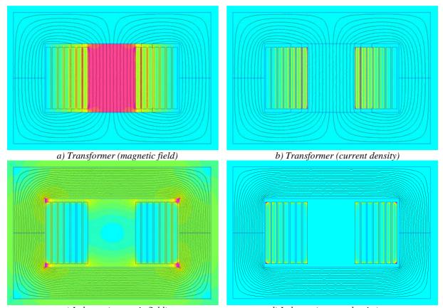
c) Inductor (magnetic field) Figure II.21: Current density and magnetic field distribution for transformer and inductor (same color scale for inductor and transformer).
