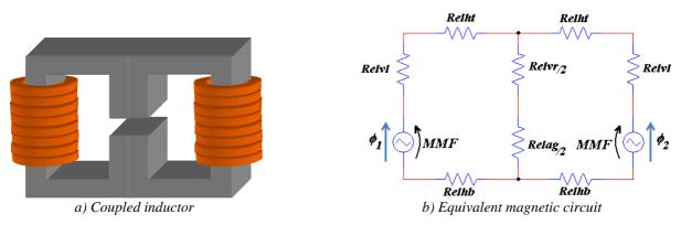
Figure I.11: ICT and its magnetic circuit.
