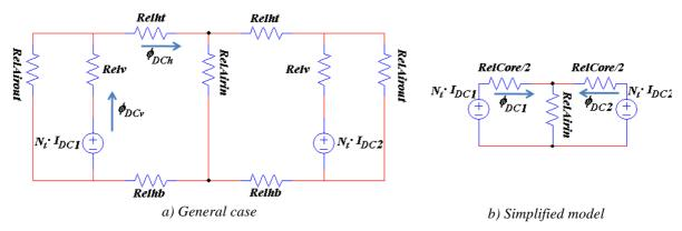
Figure III.17: Simplified model of the ICT magnetic circuit for DC or low frequency current.
