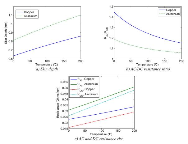
Figure II.5: Skin depth and AC resistance for different temperatures.
