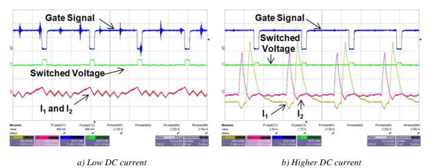
Figure III.36: High differential mode current and core saturation.
