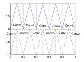
Figure V.7: Carriers for PD technique for 3-level converters.
