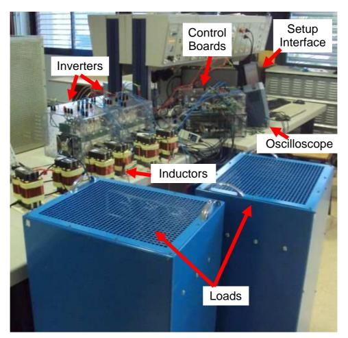
Figure V.47: Experimental setup.
