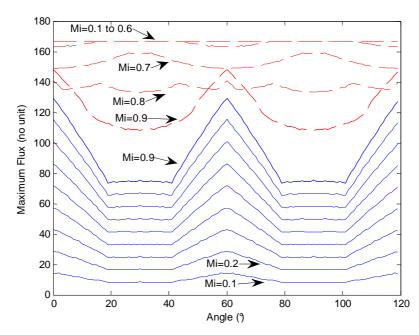
Figure V.32: Comparison of maximum flux ripples using POD (blue lines) and PD (red dashed lines) techniques.
