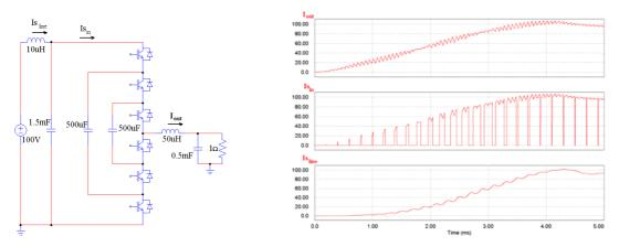
*Figure I.3: Series multicell converter and filter waveforms (F<sub>s</sub>=5kHz).*
