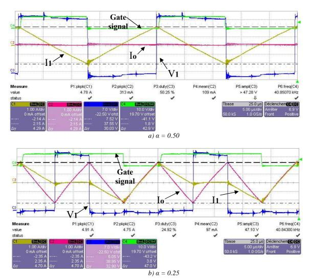
Figure III.13: Experimental waveforms at different duty cycles.
