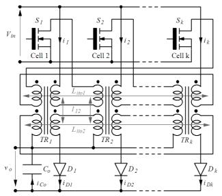
Figure I.19: ICT flyback converter with separate transformers [7].
