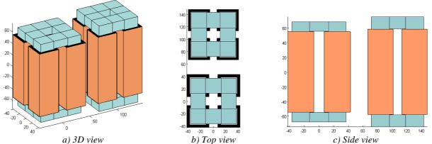
Figure IV.21: Final shape of optimized ICTs with different conductor material (scale in millimeters). Left ICT: made with aluminium. Right ICT: made with copper.
