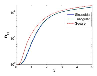
Figure II.15: Fr<sub>eq</sub> for different current waveforms.
