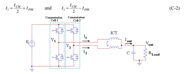
Figure C.1: Two-cell intercell transformer used in an interleaved converter.
