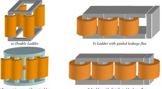
c) Symmetric core with central leg d) Ladder with distributed leakage flux Figure III.26: Different topologies of monolithic InterCell Transformers.
