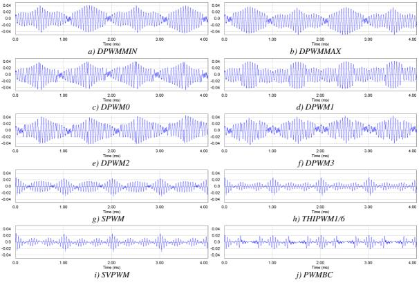
Figure V.41: ICT flux waveform for different PWM methods.
