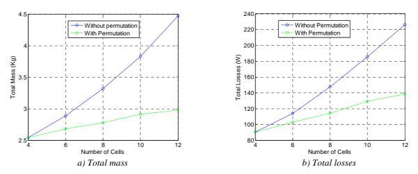
Figure IV.24: Comparison of ICT designs with and without permutation of commutation cells.
