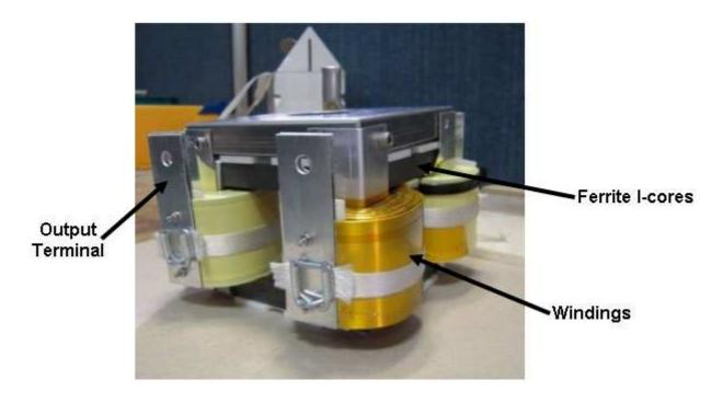
Figure III.38: CUBE ICT designed and constructed by CIRTEM.
