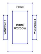
Figure IV.2: Simple model for the simulation of the energy outside the window of an intercell transformer.
