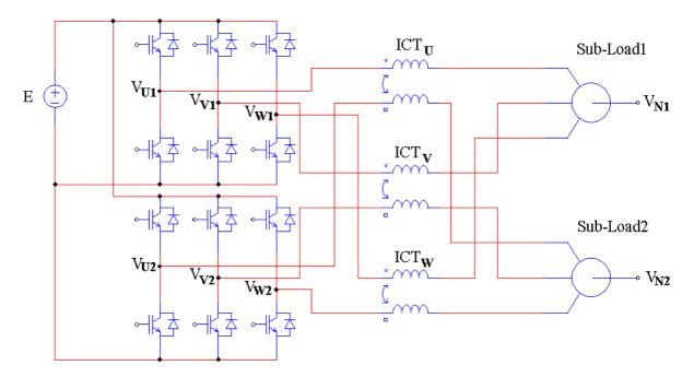
Figure V.3: Double three-phase inverter connected to double three-phase load by two-cell ICTs.
