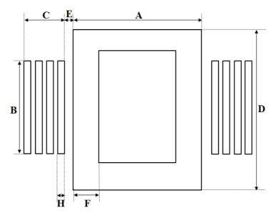
Figure IV.9: ICT geometrical parameters taking turns into account.
