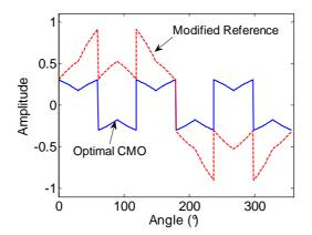
Figure V.17: Optimal CMO for high modulation indexes.
