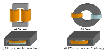
Figure III.2: Two-cell ICTs using different core shapes.
