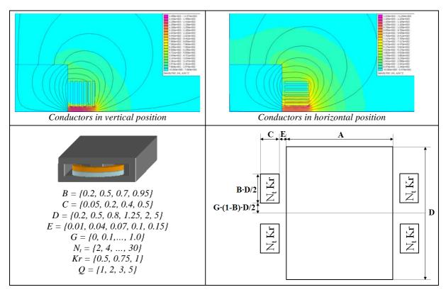
Figure IV.14: EE-core stacked windings, conductors in horizontal and vertical positions.
