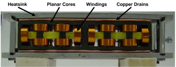
b) Prototype Figure III.34: "MONOBOBINE" ICT.
