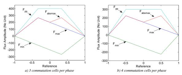
Figure V.21: Flux values for all possible reference values in 3- and 4-cell ICTs.
