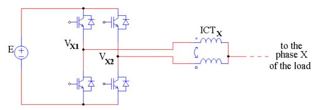
Figure V.5: One phase of the dual three-phase inverter coupled by one ICT.
