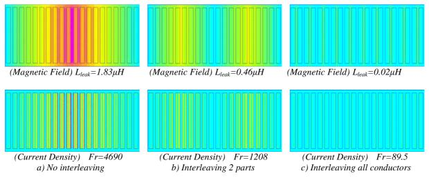
Figure II.27: Simulation of interleaved windings.
