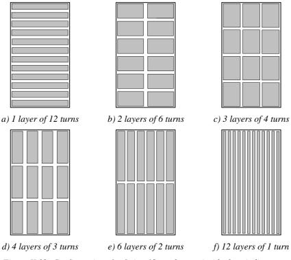
Figure II.32: Configurations for fitting 12 conductors inside the winding area.
