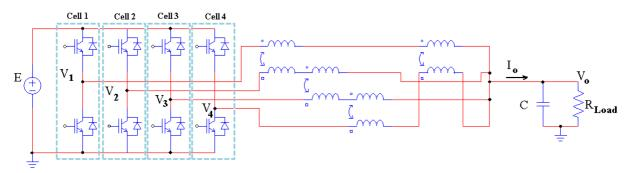
Figure III.21: 4-cell interleaved converter coupled by 4 x 2-cell ICTs (cyclic cascade topology).
