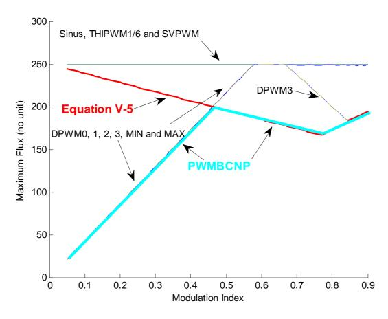
Figure V.24: Maximum flux ripple for different PWM methods.
