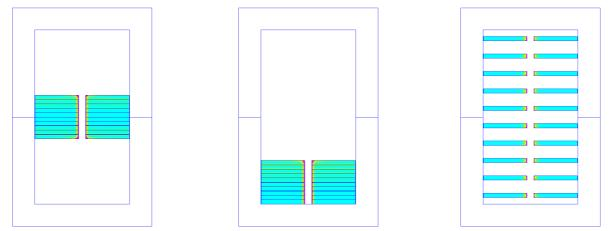
a) Centered in the window b) Close to the bottom c) Spread in the window Figure II.25: Current density of a 10-turn transformer when conductors are placed in different locations inside the core window.
