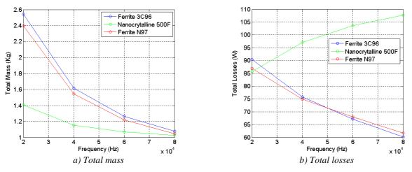
Figure IV.22: Comparison of optimized ICTs with different core materials.
