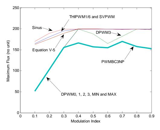
Figure V.26: Maximum flux ripple for different PWM methods for the 3-cell case.
