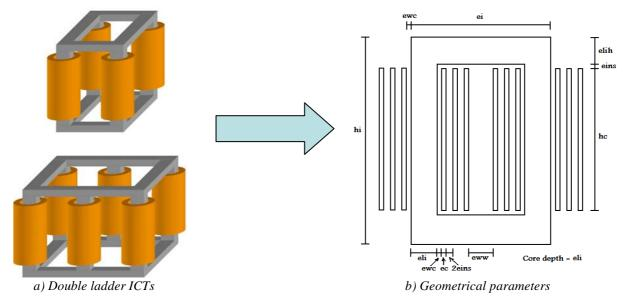
Figure IV.19: Geometrical parameters of N-cell ICT.
