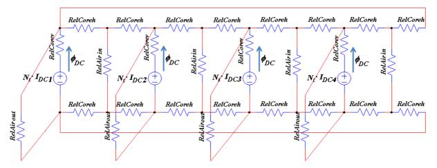
Figure III.31: Magnetic circuit of the CUBE ICT for DC or low frequency current.
