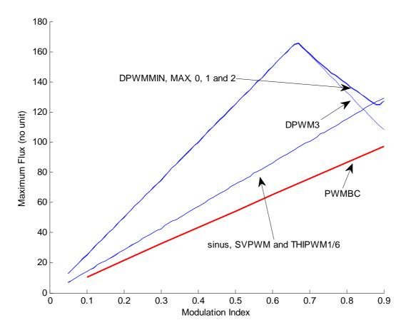
Figure V.40: Maximum flux ripple for different PWM methods.
