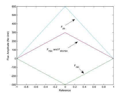
Figure V.13: ICT flux for all possible values of the reference.
