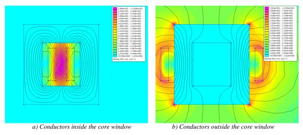
Figure III.11: FEM simulation of intercell transformer (absolute value of the magnetic field intensity).
