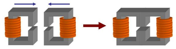
Figure IV.25: Joining two inductors to form an ICT.
