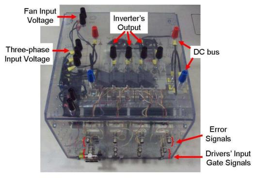
Figure V.46: Three-phase inverter used in the experimental setup (from SEMIKRON).
