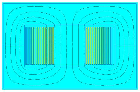
Figure II.14: Simulated ICT (current density plot).
