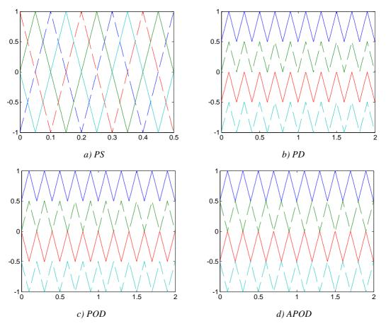
Figure V.4: Different carrier-based techniques for 5-level PWM.
