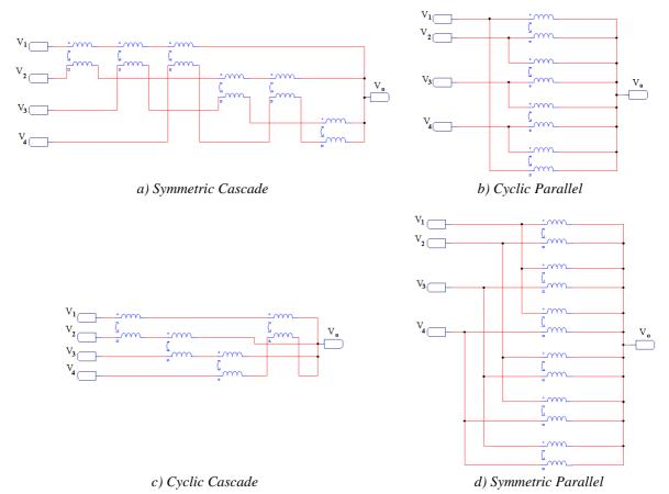
Figure 1.17: 4-phase ICT topologies using separate 2-cell ICTs.
