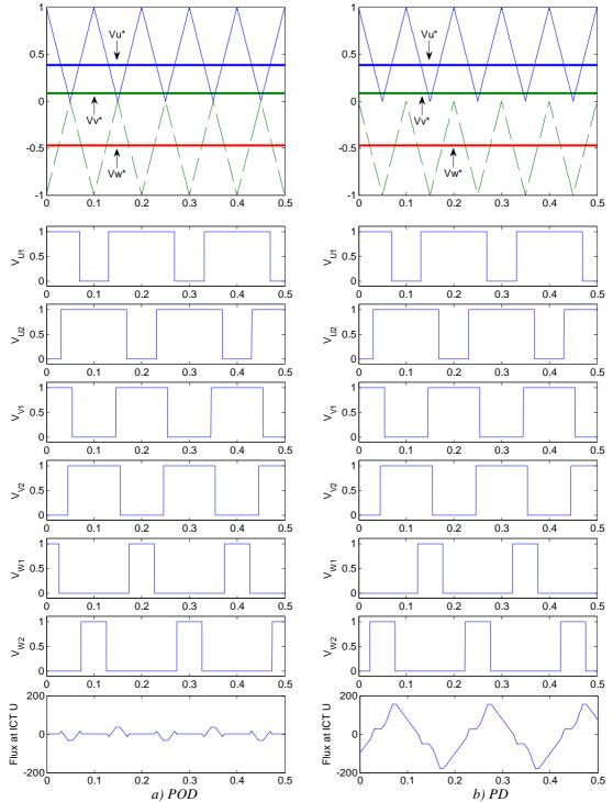
Figure V.31: Voltage reference, switching voltages and ICT flux for PD and POD techniques when Mi=0.5 and angle of the fundamental references is equal to 50°.
