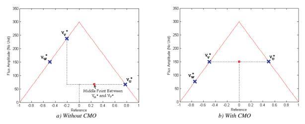
Figure V.16: Example of maximum flux oscillation with and without optimal CMO for high modulation indexes.
