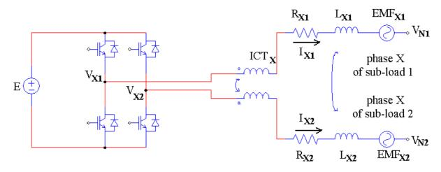
Figure V.28: One phase of the dual three-phase inverter feeding a dual three-phase load, coupled by one ICT.
