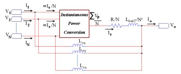
Figure III.23: Equivalent model of a symmetric ICT composed by N cells.
