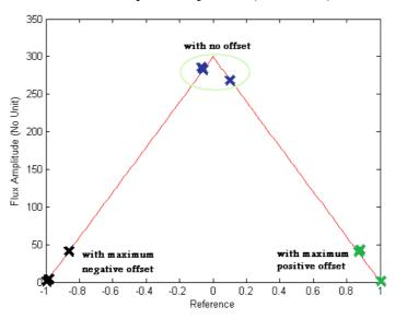
Figure V.14: Example of maximum flux oscillation with and without optimal CMO for low modulation indexes.
