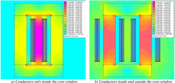
b) Conductors inside and outside the core window
