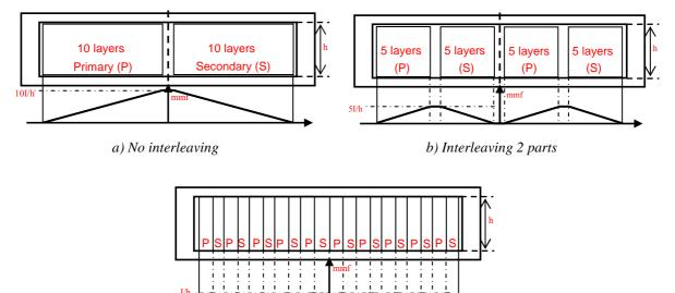
c) Interleaving all conductors
