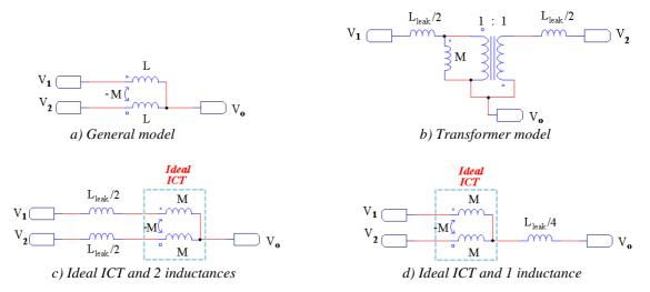
Figure III.9: ICT electrical models.
