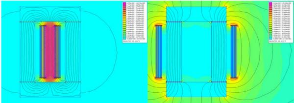
a) Conductors inside the core window b) Conductors outside the core window
