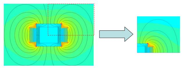
Figure IV.11: Simulation of one fourth of the total structure.
