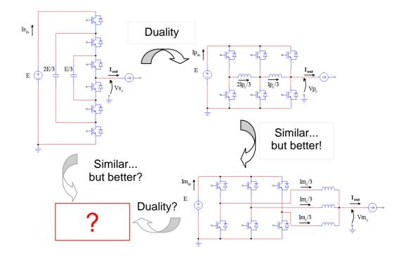
Figure I.5: Duality and similarity between series and parallel multilevel converters.
