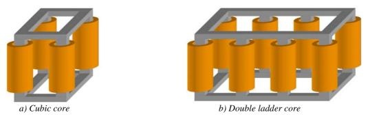
Figure 1.15: Double Ladder InterCell Transformers.
