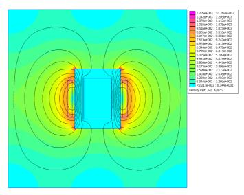
Figure IV.6: FEMM simulation of intercell transformer with rectangular boundaries (magnetic field intensity).
