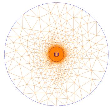
Figure IV.7: Mesh density of the FEMM simulation for good trade-off between precision and fast results.
