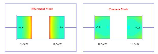
Figure C.2: Current distribution of transformer with real currents and also with corresponding differential and common mode currents.
