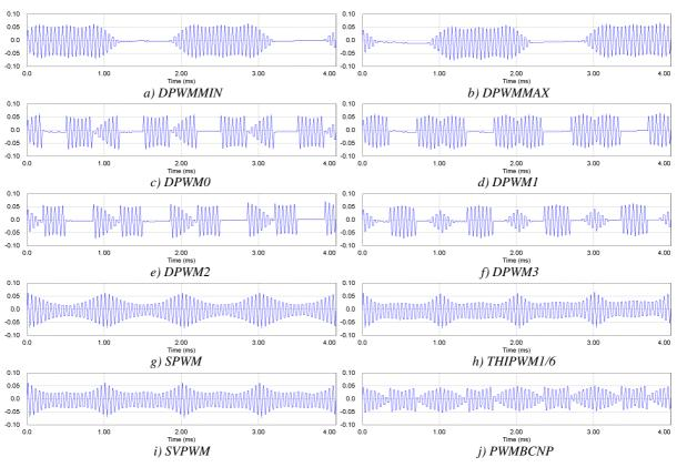
Figure V.25: ICT flux waveform for different PWM methods.
