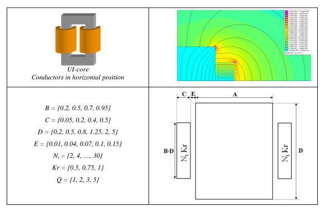
Figure IV.12: UI-core, conductors in horizontal position.
