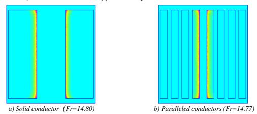
Figure II.29: Current density in solid and paralleled conductors.
