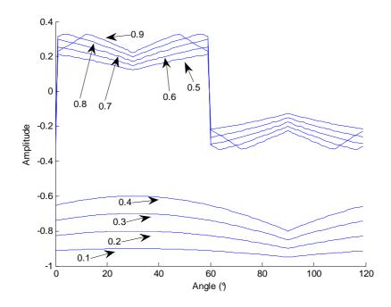
Figure V.19: Optimal CMO for all modulation indexes.
