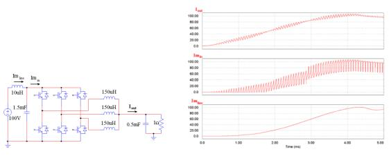
Figure I.4: Parallel multicell converter and filter waveforms ( $F_s=5kHz$ ).
