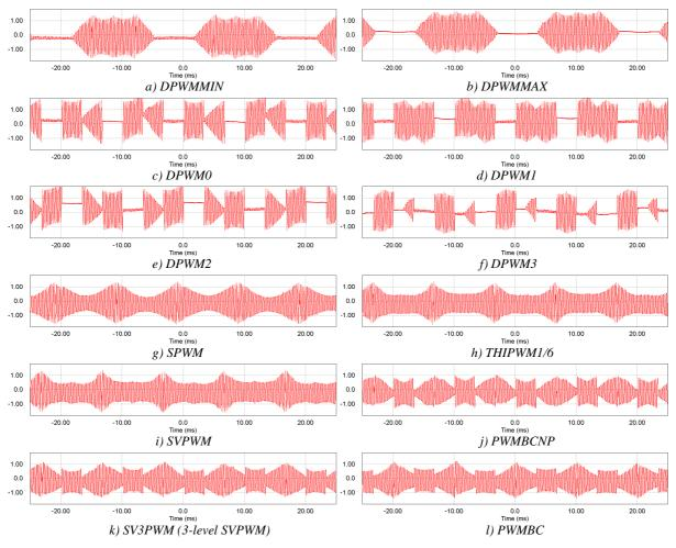
Figure V.49: Measured current differences for different methods.
