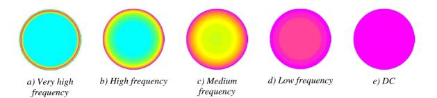
Figure II.2: Current distribution in conductors for different frequencies.
