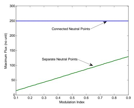
*Figure V.30: Comparison of the maximum flux ripple for the same circuit with and without neutral point connection.*
