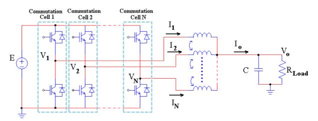
Figure III.20: N-phase intercell transformer used in an N-cell interleaved converter.
