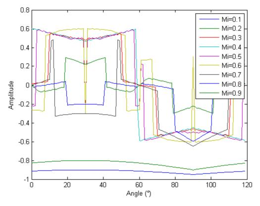
Figure V.23: Optimal CMO for 4 commutation cells per phase.
