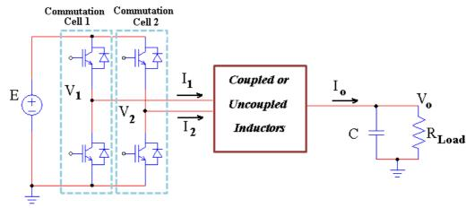
Figure I.9: 2-cell Buck converter using coupled or uncoupled inductors.
