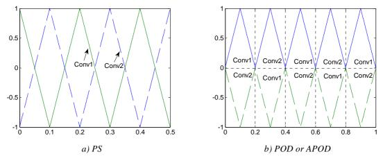
Figure V.6: Equivalence between PS, POD and APOD for the 3-level parallel converters.
