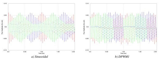
Figure V.12: ICT flux using DPWM1 and SPWM techniques.
