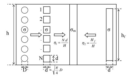
Figure II.10: Porosity factor definition for different conductor shapes.
