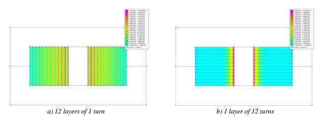
Figure II.37: Simulated transformers.
