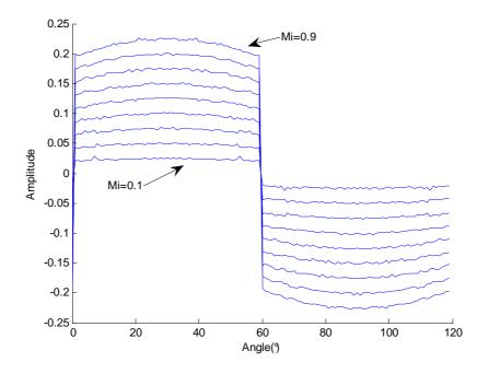
Figure V.34: Optimal CMO found by offset sweeping.
