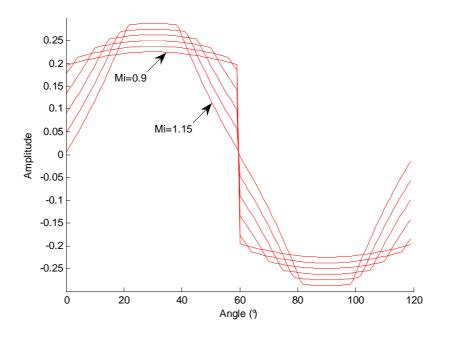
Figure V.38: PWMBC offsets in high modulation index and overmodulation regions.
