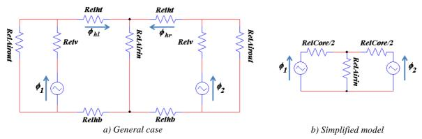
Figure III.16: Reluctance models of the ICT magnetic circuit.
