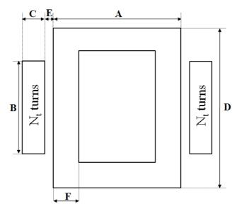
Figure IV.3: Transformer parameters.
