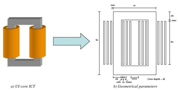
Figure IV.1: Two-cell ICT and geometrical parameters.
