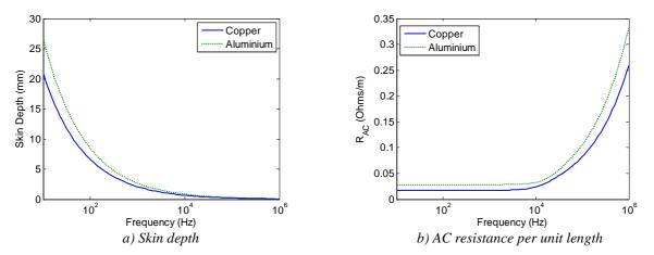
Figure II.4: Skin depth and AC resistance for different materials.
