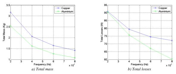
Figure IV.20: Comparison of optimized ICTs with different conductor materials.
