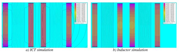
Figure III.8: Current density distribution simulation of ICT and inductor at low frequency current (50Hz).
