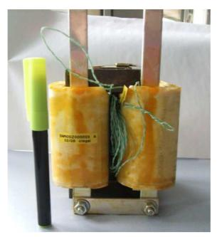
Figure III.12: Intercell transformer.
