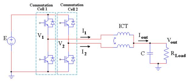
Figure III.1: Two-cell intercell transformer used in an interleaved converter.
