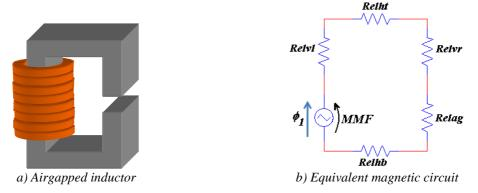
Figure I.10: Inductor and its magnetic circuit.
