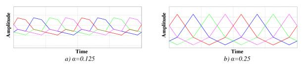
Figure III.24: Flux density waveforms in a 2-cell ICT inserted in a 4-cell Buck converter.
