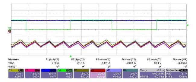
Figure III.35: Currents in the 6 commutation cells.
