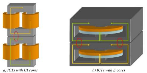
Figure III.29: Compensating magnetizing flux by joining transformers together.
