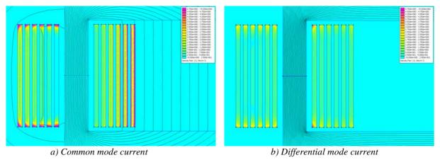
Figure III.5: FEMM simulation of a simple ICT (Current density plot), using "vertical" conductors.
