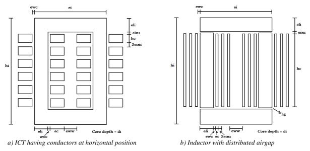
Figure IV.18: Geometrical parameters of ICT and inductor.
