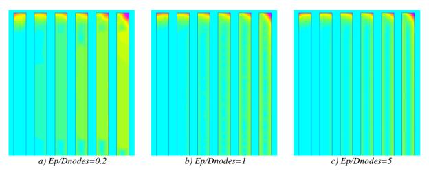
Figure IV.10: Comparison between FEMM simulations of the current density for different mesh density.
