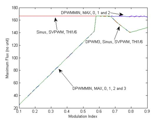
Figure V.44: Maximum flux ripple for different PWM methods.
