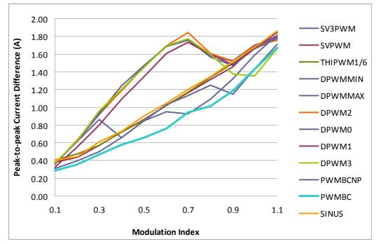
Figure V.52: Comparison of PWM methods: maximum peak-to-peak current difference obtained by experimental results.
