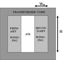
Figure II.31: Core window and winding area.
