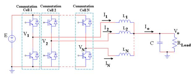
Figure I.7: Parallel Multicell Buck.
