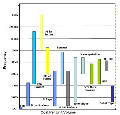
*Figure III.19: Comparison between core materials with regard to operation frequency and relative cost per unit volume.*
