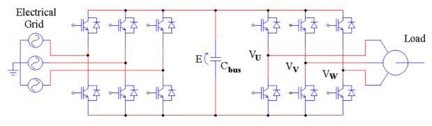
Figure V.1: Three-phase system feeding three-phase load.
