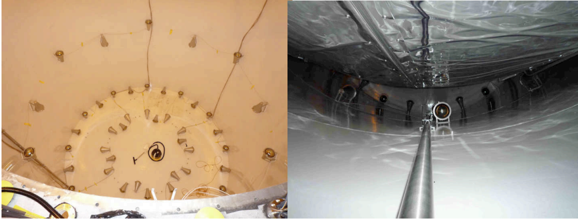
Figure 5.14: Left plot: Inner veto tank with its PMTs. Right plot: Reflective white paint on the inner veto tank wall and foils on the buffer tank outer wall.
