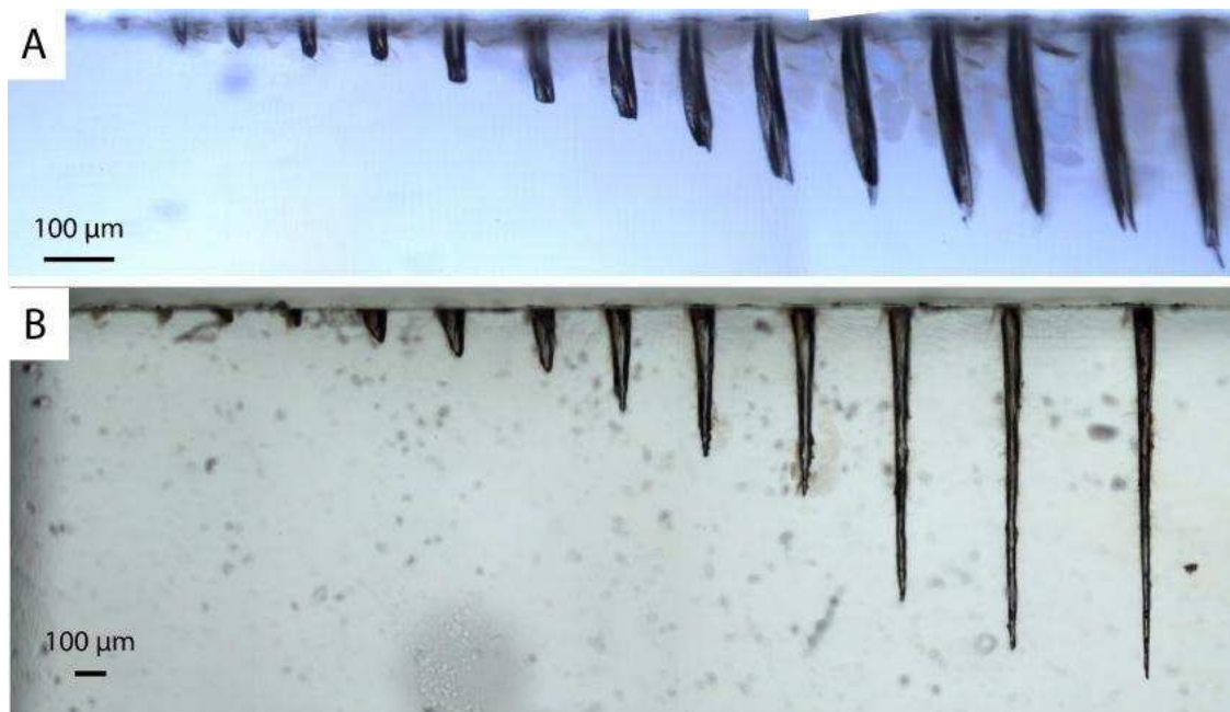
Fig 2: A. side view of an ablation serie from N=100 to N=3000 using the long focal lens. B. Side view from an ablation serie produced by the short focal objective ( N=100 to N=3000 )
