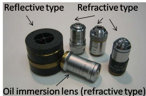
Figure 3.20 Refractive and reflective type objective lenses with various NA
