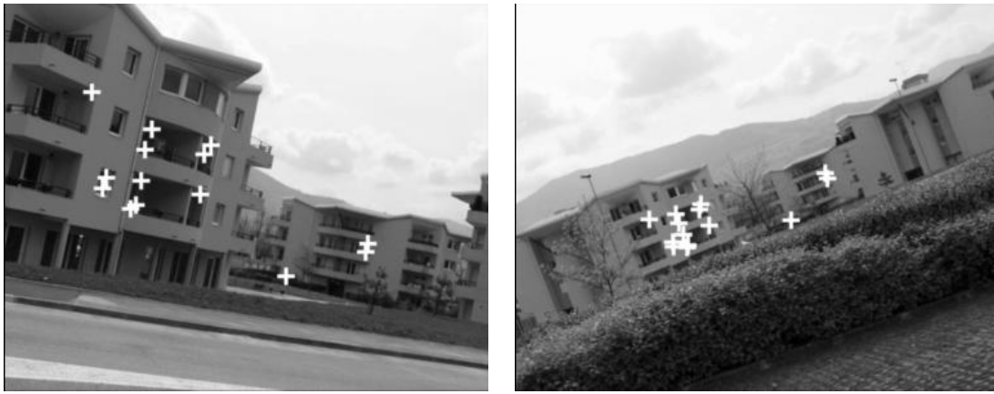
FIG. 6.2: Example of images taken from different viewpoints. There are 14 inliers to a robustly estimated fundamental matrix, all of them are correct. The estimated scale factor is 2.7.
