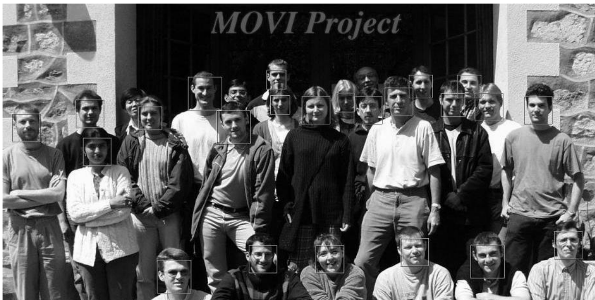
FIG. 7.9: Detection results for the frontal face detector. Note that the faces are correctly detected despite shadows and occlusions.
