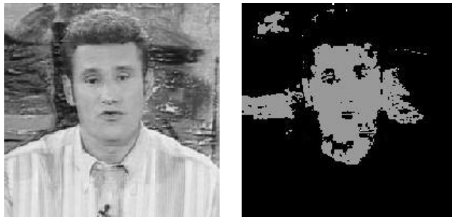
FIG. 7.6: Skin color detected with a model build in rg color space. The image displays thresholded probabilities of corresponding pixel colors.
