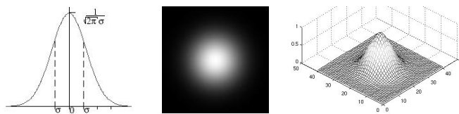
FIG. 3.1: Uniform Gaussian kernel.
