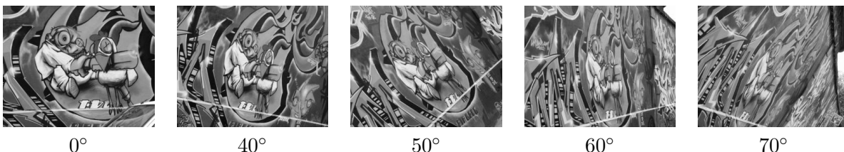
FIG. 4.10: Images of one test sequence with perspective deformations. The corresponding viewpoint angles are indicated below the images.
