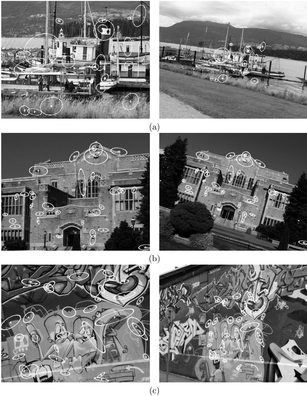
FIG. 6.8: Correctly retrieved images. The displayed matches are the inliers to a robustly estimated fundamental matrix or homography between the query image (on the left) and the most similar image in the database (on the right). There are (a) 22 matches, (b) 34 matches, (c) 22 matches and (d) 33 matches. All of them are correct.
