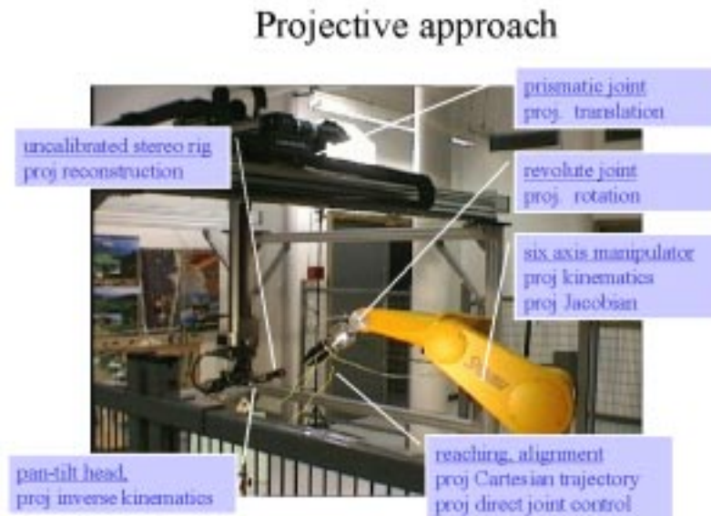
Figure 1.3: Modelling of a robotic work-cell using a stereo camera pair.
