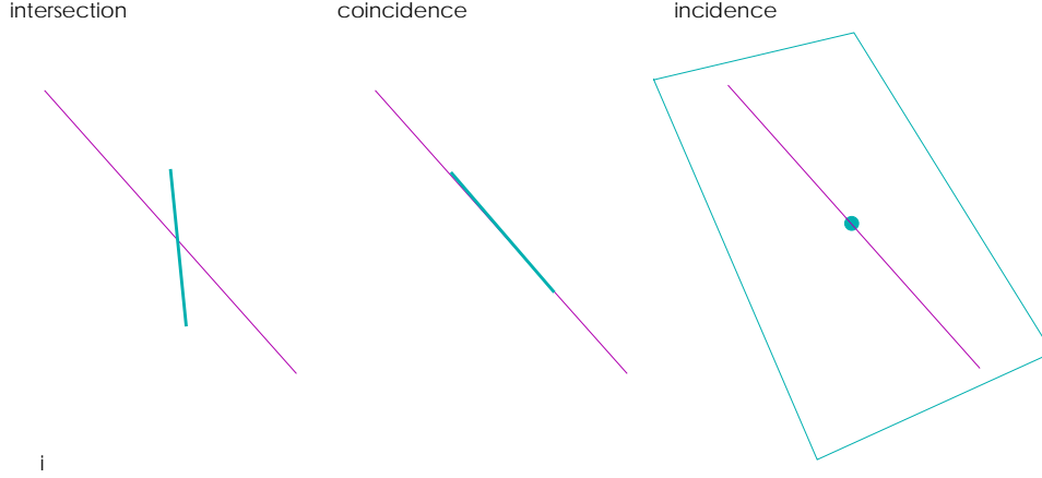
Figure 2.15: Intersection, incidence, and coincidence relation between linear geometric features, i.e. points, lines, planes, . . .
