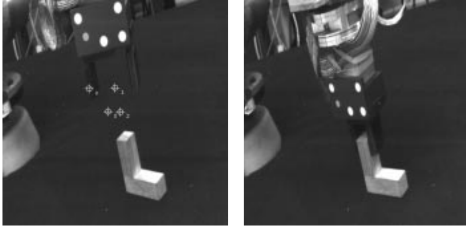
Figure 7.1: Alignment task encoded by means of a projective displacement, expressed relative to a basis of five points on the L-shaped object.
