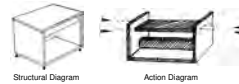
Figure 2: Hand-drawn assembly diagrams for the TV stand. The action diagram is preferable to the structural diagram because it depicts the operations required to attach each part. In this case the action diagram shows how the shelf is fastened to the stand.
