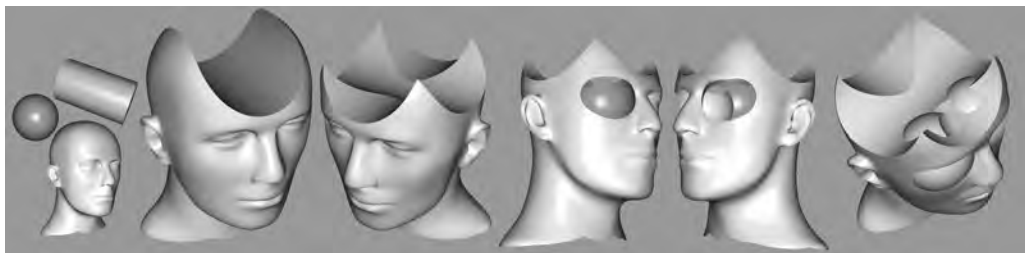
Figure 11: Subtracting 2 cylinders (230k surfels each, octree depth 4) and 2 spheres (46k surfels each, octree depth 4) from the mannequin head (350k surfels, octree depth 5). Average interaction rate is 4.4 FPS. Left: original solids. Middle: the four boolean operations. Right: resulting geometry.
