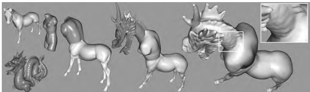
Figure 12: Mythical centaur constructed from the horse model (340k surfels), the Venus model (250k surfels) and the dragon model (650k surfels) all with octree depth 5. Average interaction time of union between horse model and Venus model was 2.5 FPS, between dragon head and centaur body was 3.3 FPS. Local smoothing is performed in the neighborhood of the surface-surface intersections.
