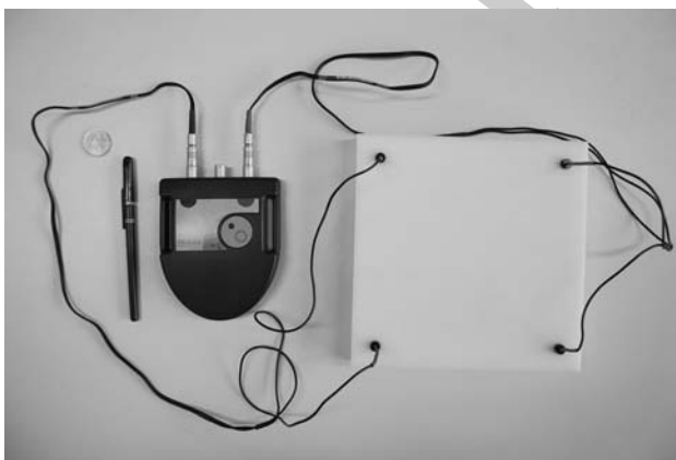
Fig. 5 The new device (a center frame and two pairs of electromagnetic coils secured: 2 transmitters, and 2 receivers) and the calibration square
