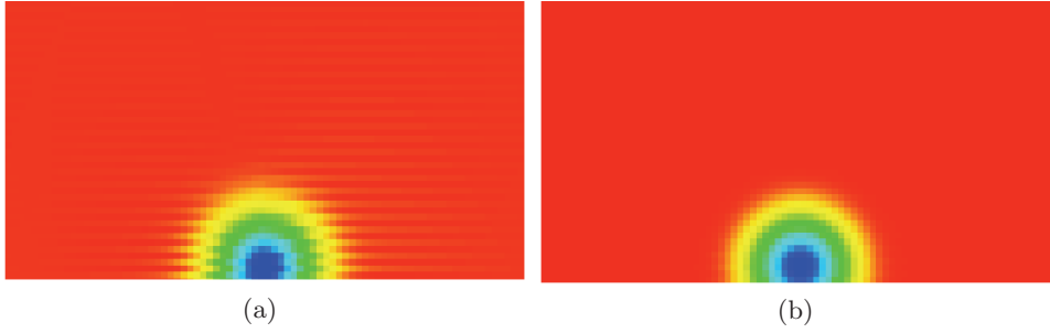
Figure 3.4: Normalized pressure map of a convected single-vortex at the instant it goes through a subsonic non-reflecting outflow without specific treatment of the artificial dissipation at the boundary (a) and with zeroth-order extrapolation of the net artificial dissipation flux (b).
