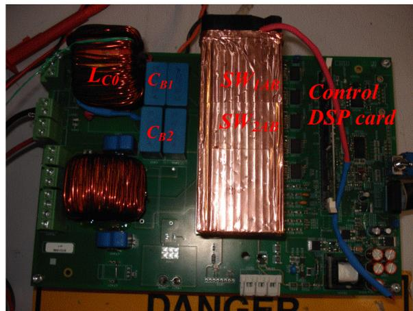
Fig. 4.8 Prototype of 5.5kW three-level dc-dc converter.
