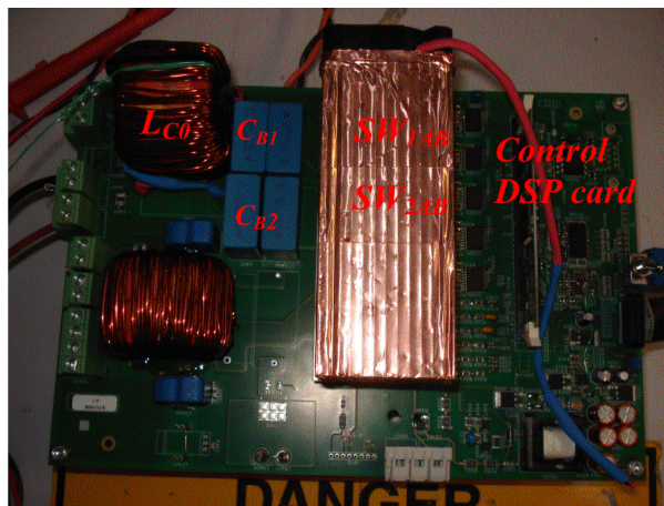
Fig. 4.8 Prototype of 5.5kW three-level dc-dc converter.
