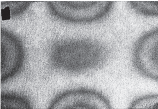
Figure 2: Time-averaged hologram of plate vibrating at 1733 Hz
