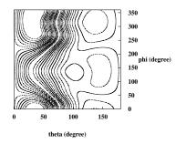
Figure 2.4: Potential for single CO adsorbed on Ar(100). The dependence of the potential on the molecular orientation angles  $\theta$  and  $\varphi$  is plotted (data from Parneix [61]).
