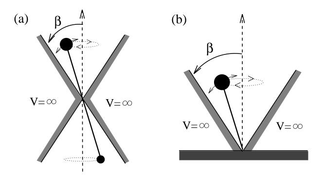
Figure 1.9: Hindered rotor model of U.Landman [137].
