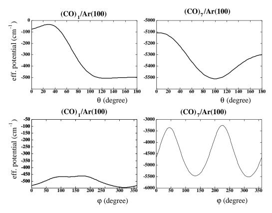
Figure 2.8: Cut of the two-dimensional potential surface (see Fig.2.4–2.7) at the global minimum. (CO)<sub>1</sub> in the left column and the central CO in the (CO)<sub>7</sub> cluster in the right column adsorbed on Ar(100). First row: Potential cut as function of  $\theta$  at  $\varphi$ =-44° and -46°, resp. Second row: Potential cut as function of  $\varphi$  at  $\theta$ =134° and 100° (data from Parneix [21]).
