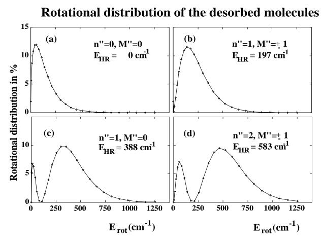
Figure 3.9: Rotational distribution of CO desorbed from Cu(111) by calculation of the Franck–Condon overlap between the hindered rotation and free rotation wave functions. CO adsorbed on–top at z = 2.41 and R = 1.167 Å.
