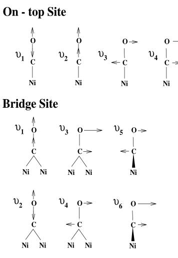
Figure 1.5: Normal modes of on-top and bridge-bonded CO (from Richardson and Bradshaw [47]).
