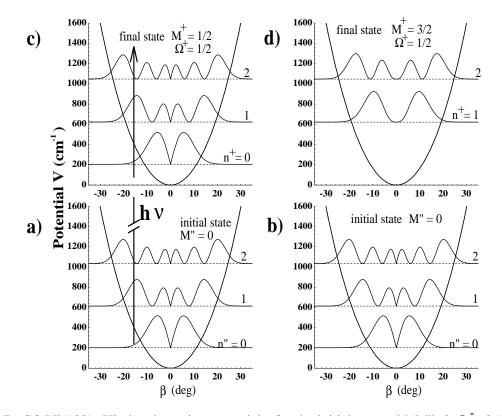
Figure 3.7: CO/Ni(100): Hindered rotation potentials, for the initial state with M''=0  $\Omega''=0$  (fig.a), b)) and two final states with  $M^+=1/2$ ,  $\Omega^+=1/2$  (fig.c)) and  $M^+=3/2$ ,  $\Omega^+=1/2$  (fig.d)). For each potential the rotational energy levels and the corresponding density functions (square of the wave function multiplied by sin  $\beta$ ) are represented (from Büchner and Raseev [11]).
