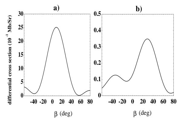
Figure 3.12: Angular distribution of electrons emitted from CO/Ni(100). Same set–up as in Fig.3.11. a)  $M^+=1/2$ ,  $\Omega^+=1/2$ ,  $n^+=0$ ,  $\leftarrow M^{"}=0$ ,  $\Omega^{"}=0$ ,  $n^{"}=0$  b)  $M^+=3/2$ ,  $\Omega^+=1/2$ ,  $n^+=2 \leftarrow M^{"}=0$ ,  $\Omega^{"}=0$ ,  $n^{"}=2$  (from Büchner and Raşeev [11]).
