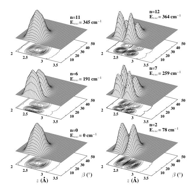
Figure 3.4: Wave function density for the coupled hindered rotation — *z*–stretch motion. (square of the wave function multiplied by  $\sin \beta$ ).
