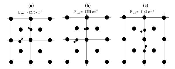
Figure 2.3: The energetically lowest adsorption geometries of two CO molecules adsorbed on Ar(100) (fcc). The adsorption energy  $E_{bind}$  is -1276, -1251 and -1164 cm<sup>-1</sup>, respectively (from Parneix [61]).
