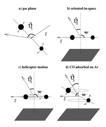
Figure 3.8: Pictural representation of models which simulate the physisorbed CO molecule: a) gas phase, b) 'oriented–in–space', c) "helicopter motion', d) hindered rotation model (from Büchner and Raşeev [11]).
