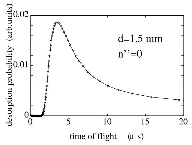
Figure 3.11: Time of flight spectrum of CO desorbed from Cu(111) in  $\mu s$ . The distance surface–probe laser is d=1.5 mm. Before desorption The CO molecules are assumed to be adsorbed in their ground vibrational state ( $n_{"}=0$ ). The hindered rotation and translation, but not the CO–surface and internal vibration are frozen (upright on–top adsorption site).  $E_{kin}^{max} = \frac{1}{2m_{CO}} (E_{kin}^{max})^2 = 220 \text{ cm}^{-1}$ .
