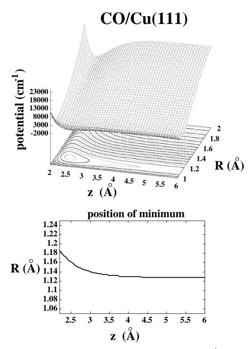
Figure 3.5: CO/Cu(111): potential for CO–surface and internal vibration in cm<sup>-1</sup>. The adsorbate is kept in upright position ( $\alpha$ ,  $\beta$ =0°) with R=1.167 Å. Upper figure: Potential respect to the intranuclear distance R and the CO–centre–of–mass surface distance z. Lower figure: position of potential minimum. The position of the minimum is only slightly varying in R.
