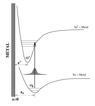
Figure 1.6: Model of Gadzuk for vibrational excitation after photoionization. Due to the attractive ion – image ion interaction, the potential of the final ionic state is deeper and shifted towards the surface, causing Franck–Condon type excitation of the final xenon–surface vibrational state (from Gadzuk [52]).
