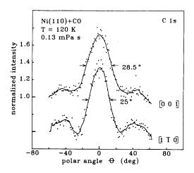
Figure 1.7: 1253.6 eV photoelectrons ionize CO/Ni(110). The polar dependence of the photoelectrons coming from the carbon 1s shell are plotted for electron emission in [001] and [110] directions and for a sample temperature 120 K, (from Wesner et al. [14]).
