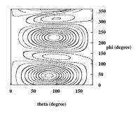
Figure 2.7: Contour plot representation of Fig.2.6. The minimum is at  $\theta$ =100°,  $\varphi$ =314° and *V* = -5509.6 cm<sup>-1</sup>. Each line indicates a difference of 100 cm<sup>-1</sup> starting at -5600 cm<sup>-1</sup>.
