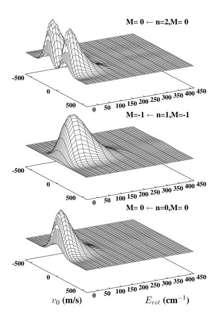
Figure 3.12: Rotational and translation distribution of CO desorbed from Cu(111) in arb.units. The particles have a velocity  $v_{speed} = v_0 + \Delta v$  in z direction. Their rotational energy is  $E_{rot} = B_{CO} * J(J+1)$  with  $B_{CO} = 1.93$  cm<sup>-1</sup>.
