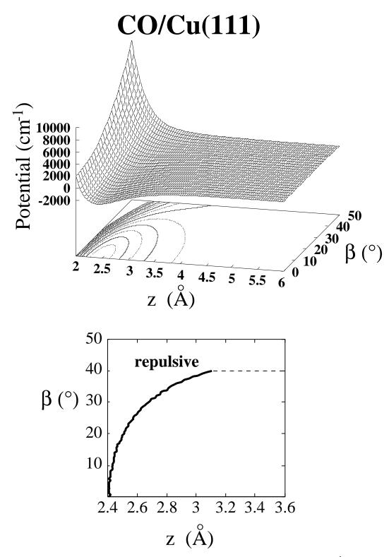
Figure 3.2: CO/Cu(111): potential for hindered rotation and CO–surface stretch in cm<sup>-1</sup>. Upper figure: Potential with respect to the tilt angle  $\beta$  and the CO–centre–of–mass surface distance z. The molecule is adsorbed on–top site with the intramolecular distance fixed at R=1.167 Å. Lower figure: position of potential minimum. Note, that for  $\beta>40^\circ$ , the potential in z is purely repulsive.
