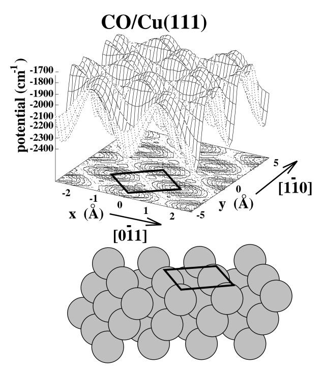
Figure 3.6: Potential for hindered translation motion of the CO adsorbate parallel to the (111) surface of the fcc copper crystal in cm<sup>-1</sup>. The molecule is kept in upright position to the surface with R=1.167 Å. The x axis is defined by [011] direction one the surface and the y axis by [111]. The potential in xy is varies by about 500 cm<sup>-1</sup>.
