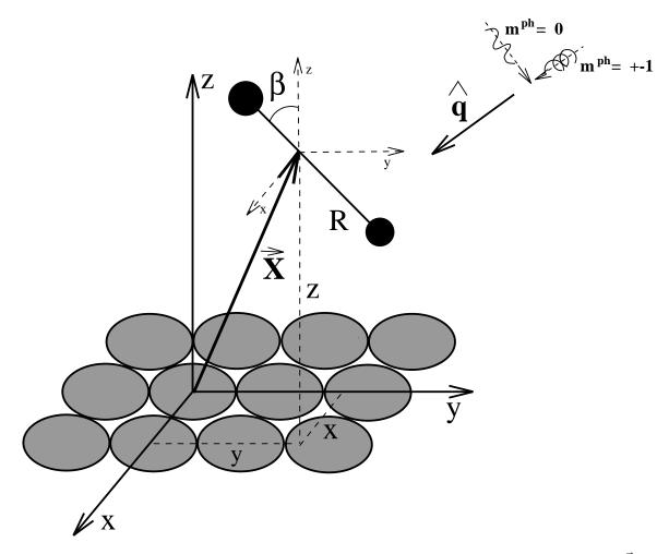
Figure 2.1: Coordinate system for structured surface allowing hindered translation and rotation.  $\vec{X} = (x, y, z)$  is the position of the centre of mass of the molecular adsorbate,  $\beta$  is the tilt angle of the molecular axis and defines together with  $\alpha$  and  $\gamma$  (not shown here) the molecular orientation. R is the intranuclear distance of the the adsorbate.
