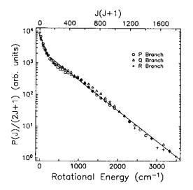
Figure 1.4: Experimental rotational populations of CO desorbed from oxidised Ni(111), normalised to the degeneracy. 3.3 mJ/cm<sup>2</sup> fluence/pulse, same set–up as in Fig.1.3 The two straight lines correspond to rotational temperature population with  $T_{rot}$ =200 and 634 K, resp. (from M.Asscher et al. [32]).
