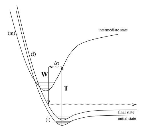
Figure 2.2: Present two step model. The photon excites the molecule–surface system from the initial (i) to the upper state (m) (photon operator T). The excited state is coupled by non-adiabatic interactions W to the final state (f). These interactions determines a decay time  $\Delta \tau$ .
