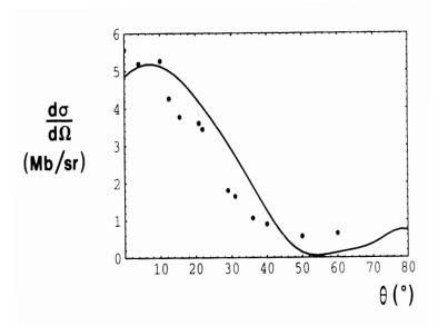
Figure 3.3: Angular photoelectron distribution of the  $(4\sigma)^{-1}$  ionization. The light (35 eV) is linear polarized, while  $\Theta$  is the photoelectron ejection angle in the photon – surface normal plane ( $\varphi=0^\circ$ ). The full line is the theoretical calculation. The dots are experimental results from Allyn et al. [4], normalised to the theoretical curve (from Budău et al. [13]).
