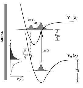
Figure 1.8: Centre–of–mass translational motion of the adsorbate. The photon excites the ground state wave packet to the negative  $2\pi^*$ resonance state with its associated potential curve (V<sub>-</sub>(z)). The wave packet propagates in time on V<sub>-</sub>(z) during a characteristic decay time  $\tau_r$ . Then it decays to the ground state and desorbs. (from Gadzuk et al. [130].
