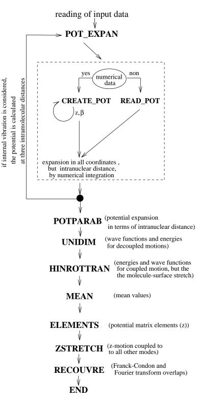
Figure E.1: Flowchart of the program, calculating the Franck–Condon and Fourier transform overlap between the coupled hindered rotation, translation, internal vibration, molecule–surface stretch of the adsorbed molecule and those of the gas phase. rotation.
