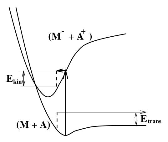
Figure 1.6: Desorption mechanism in the Antoniewicz model [126]. Here A is the adsorbate and M is the metallic surface.
