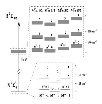
Figure 3.4: Rotational energy levels of CO/Ar for the initial  $(X^{1}\Sigma_{0}^{+})$  and the final  $(B^{2}\Sigma_{1/2})$  electronic states. Note, that the energy scales for the initial and final states are different (from Büchner and Raşeev [11]).
