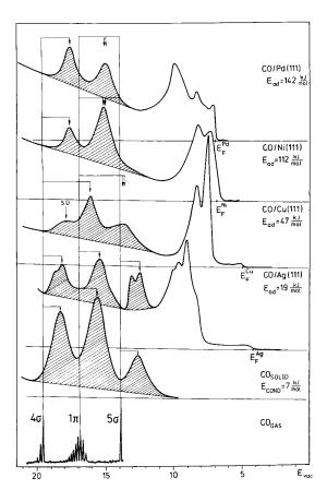
Figure 1.1: Different adsorbate systems in normal emission, the binding energy  $E_B = h\nu - E_{kinetic}$  is given with respect to the vacuum level  $E_{vac}$  (from [41]). One can see a shifting of ionization potentials and a broadening depending on the substrates.
