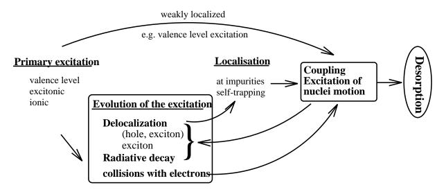
Figure 1.1: Elementary processes in electronically stimulated desorption (adapted from P.Feulner and D.Menzel [118]).
