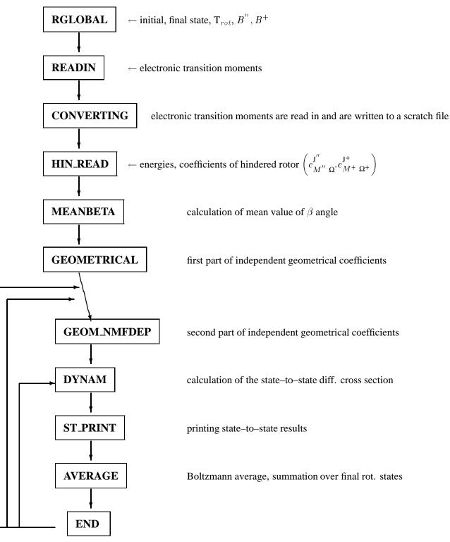
Figure C.1: Flowchart of the program, calculating the photoionization cross section for molecular adsorbates, including hindered rotation.
