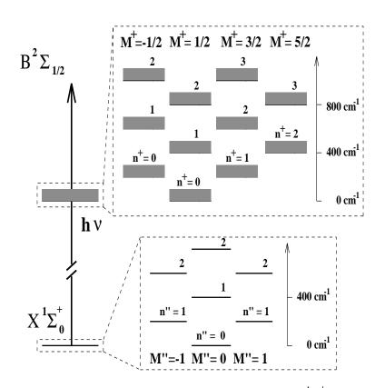
Figure 3.6: Rotational energy levels of CO/Ni(100) for the initial  $(X \ ^1\Sigma_0^+)$  and the final  $(B \ ^2\Sigma_{1/2})$  electronic states (from Büchner and Raşeev [11]).
