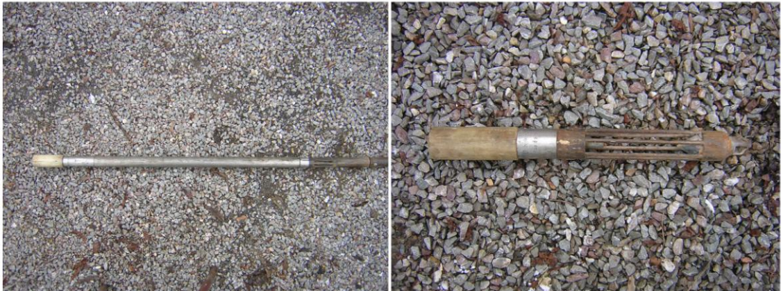
Fig. 12. Photograph of high sensitive probes for temperature measurements.
