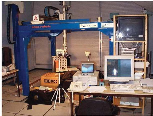
Figure 3.8 – Experimental system: Cartesian robot
