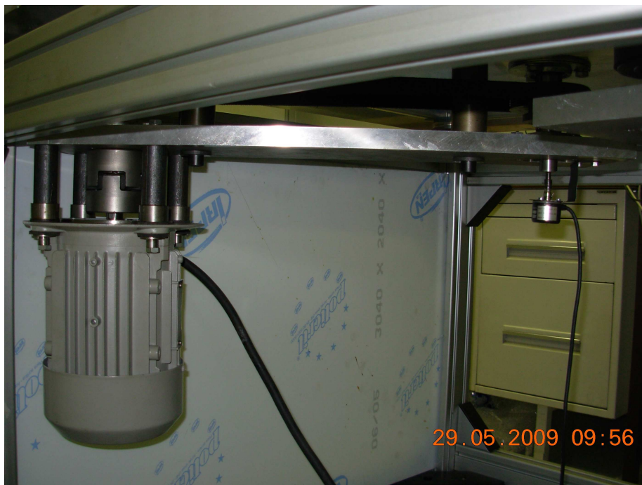
Figure 3.3: Electric motor placed underneath the disk assembly, on the right side there is a sensor placed for the measurement of disk rotation rate.
