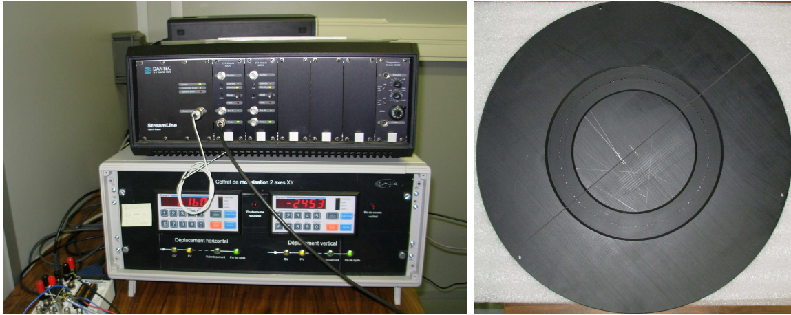
Figure 3.10: Left top: Dantec Dynamics StreamLine constant temperature anemometer, left bottom: digital controller for the hot-wire positioning above the disk surface, right: PVC light weight disk used for the radial alignment of the hot wire.
