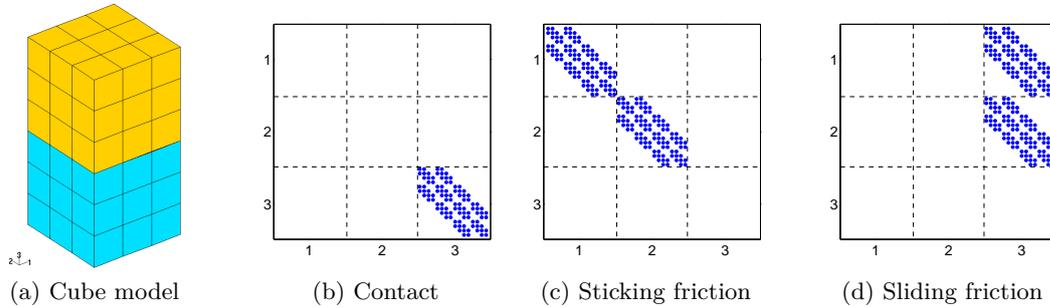
Figure 3.14: Tangent contact-friction matrix topologies on a simple case. Direction 1,2 are horizontal (friction plane). Direction 3 is vertical (contact direction).
