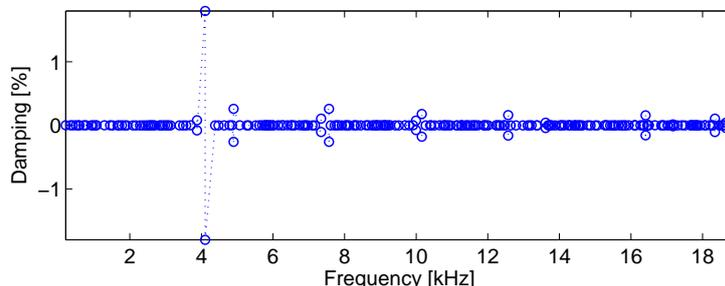
Figure 3.16: Brake stability diagram at 12 Bar
