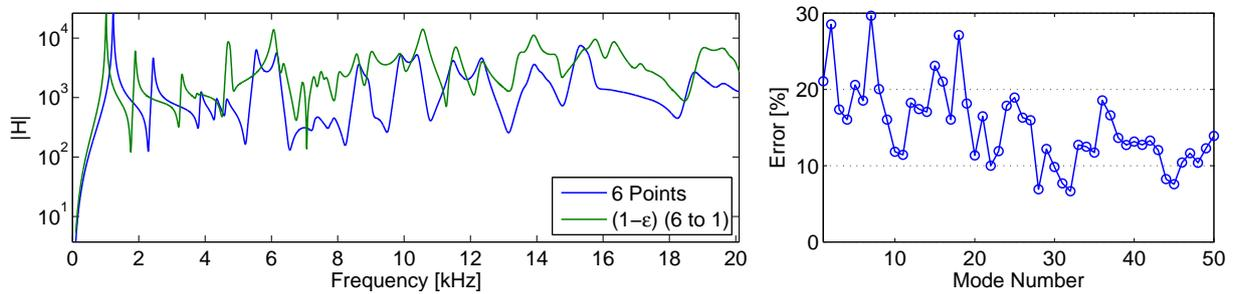
Figure 2.54: Left: Dynamic behavior differences between the use of a 6 point integration rule contact integration law, and the regularization strategy based on a 1 point integration rule for  $\epsilon = 10^{-3}$  (42% of quasi-compatible shapes kept). Right: Frequency differences observed at peaks
