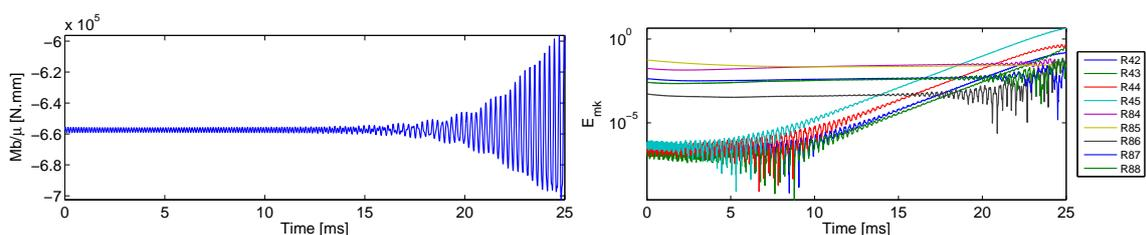
Figure 4.43: Targeting unstable mode C84, braking torque and main modal mechanical energies
