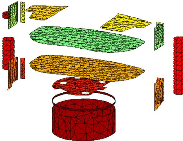
Figure 1.7: Contact elements of the brake system
