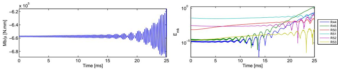
Figure 4.41: Targeting unstable mode C51, braking torque and main modal mechanical energies
