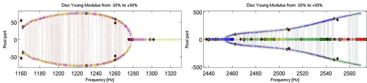
Figure 2.31: Full stability diagram as function of the disc Young modulus, green diamond at the nominal point, red diamonds for the ABAQUS recomputed solution and yellow diamonds for the corresponding prediction
