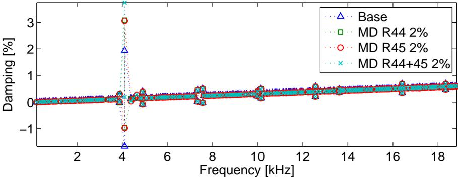
Figure 5.33: Industrial brake stability diagram at 12 Bar as function of real modes R44 and R45 modal damping
