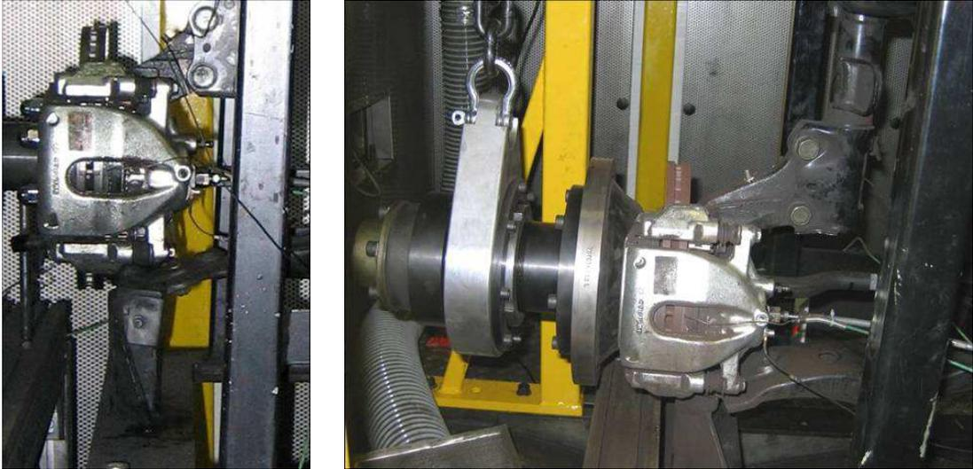
Figure 1.11: A squeal test bench at Bosch facilities
