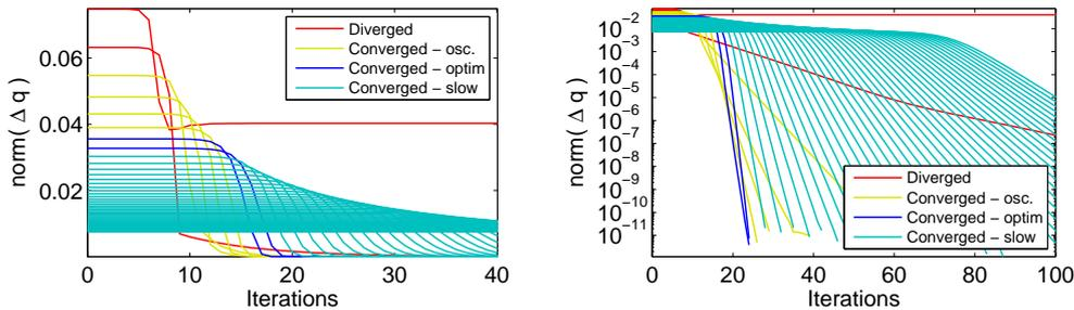
Figure 4.11: Convergence pattern plotting the correction increment quadratic norm as function of the iterations in the Newton-Raphson resolution and as function of the Jacobian parameter  $k_c$ . Left: linear y scale. Right: logarithmic y scale
