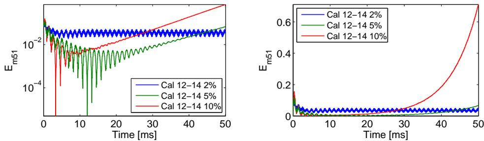
Figure 5.60: Effect of damping caliper mode 12 to 14 on the limit cycle obtained at 12 Bar, modal mechanical energies associated to mode C51
