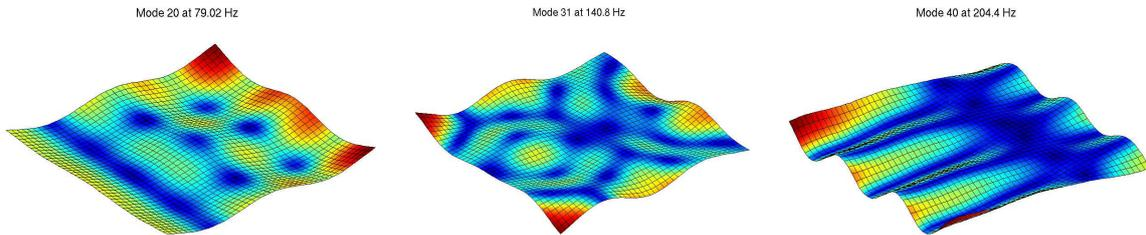
Figure 2.22: Plate mode shape variation for an increase by 20% of half-plate #1 Young modulus
