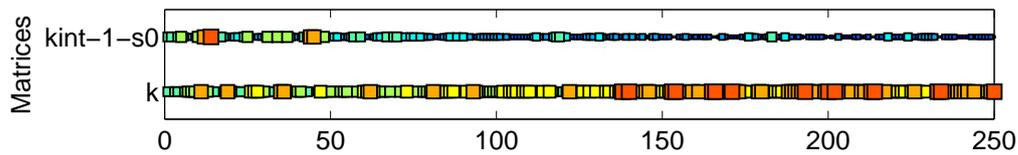
Figure 3.21: System complex mode distribution by matrix, from top to bottom, elastic interaction matrix  $k_{int\_s0}$  (contact and sticking friction) and elastic stiffness  $k$  (components). The hotter the color and the larger the marker, the higher the energy fraction
