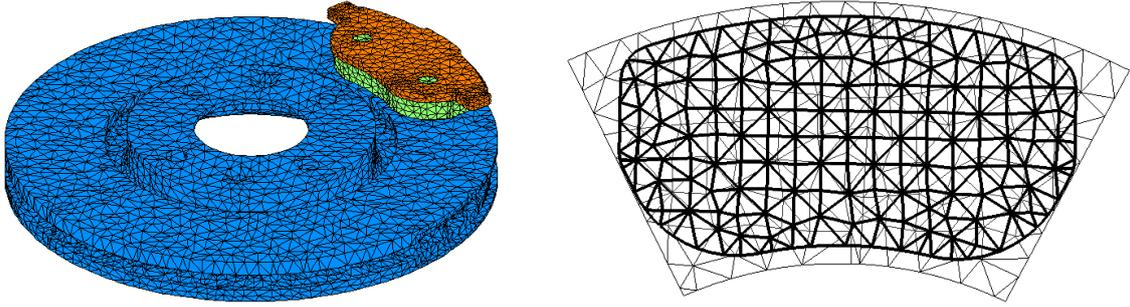
Figure 2.50: Pad/Disc model and superimposed interface discretization
