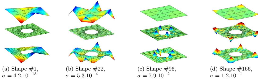
Figure 2.46: Shapes resulting from the SVD of  $[A]$  plotted on  $\Gamma_1$  and  $\Gamma_2$ . The gap is computed and plotted on the Gauss points of  $\Gamma$
