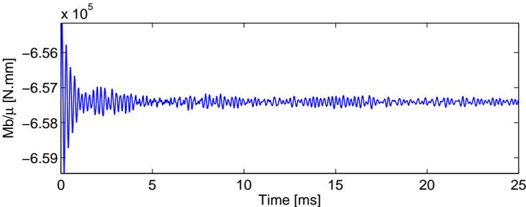
Figure 4.39: Braking torque for a 10% modal damping of modes R42 to R48
