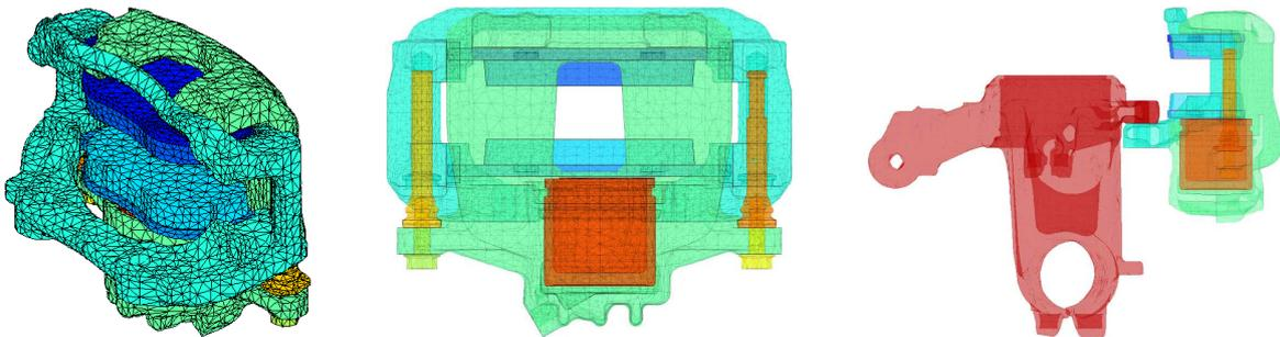
Figure 1.5: Stator part of the brake system
