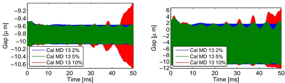
Figure 5.55: Effect of damping caliper mode 13 on the limit cycle obtained at 12 Bar, slip-separation pattern evolution through sample gap measurements
