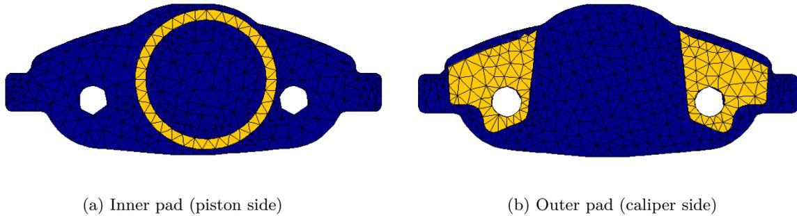
Figure 1.6: Braking pressure transmission areas on the pads
