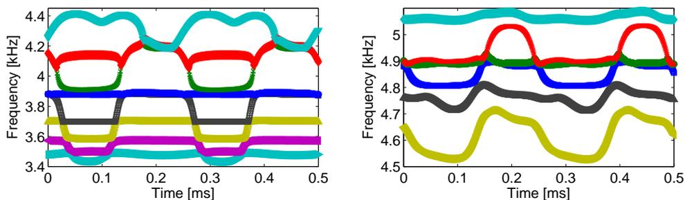
Figure 5.7: Frequency variation of the brake complex modes in the squeal limit cycle at 4 and 5 kHz
