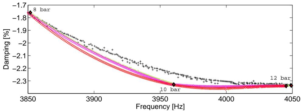
Figure C.5: Various interpolation strategies between 8 and 12 bar. + Linear interpolation between 8 and 12 bar. + Piecewise interpolation between 8 and 10 bars then 10 and 12 bar.  $\diamond$  Piecewise interpolation between 8 and 12 bar using 3 reduction bases at 8, 10 and 12 bar.  $\diamond$  3 points quadratic interpolation using 8,10 and 12 bar
