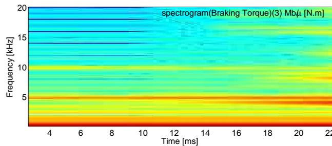
Figure 4.42: Targeting unstable mode C51, braking torque spectrogram
