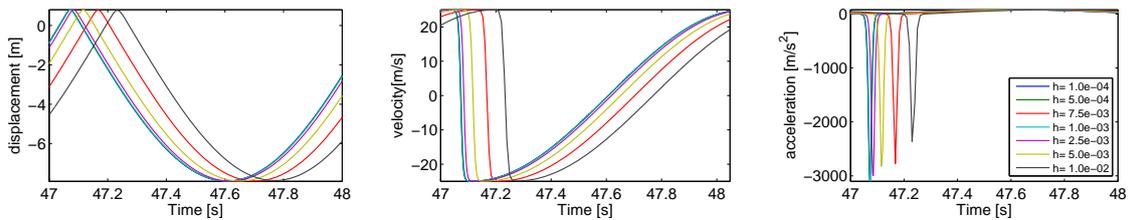
Figure 4.8: Displacement, velocity and acceleration signals for a 50s time simulation of the mass-exponential spring system
