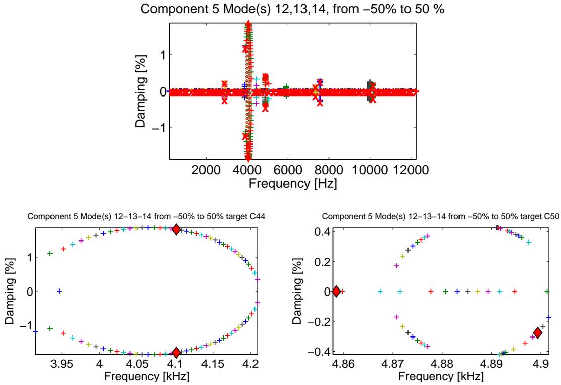
Figure 5.42: Effect of caliper modes 12, 13 and 14 frequency tuning from -50 to +50 % on the global system stability at 12 Bar. Red diamond stands for the nominal state
