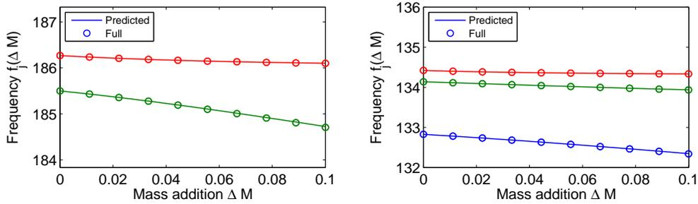
Figure 2.24: Plate frequency variation as function of the added mass on half-plate #2, predictions from the CMT (-) and recomputations (o)
