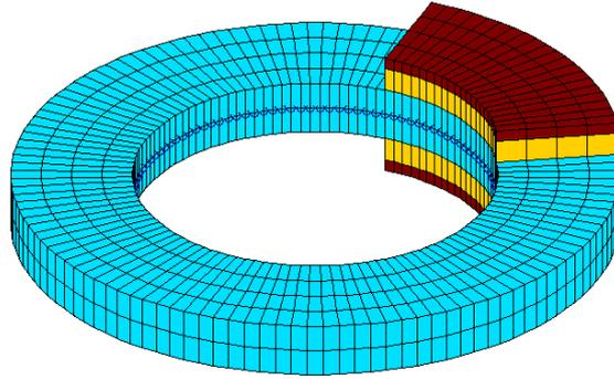
Figure 1.13: Simplified brake model used for code validations
