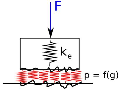
Figure 3.6: Representation of contact between two bodies, body stiffness and asperities
