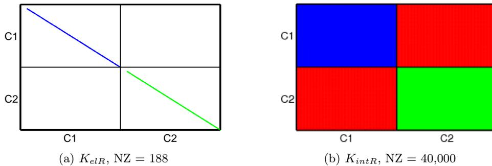
Figure 2.9: Reduced matrix topologies for the CMT formulation. The use of rigid body modes yields zero diagonal terms on the elastic matrix. The mass matrix is reduced to the identity
