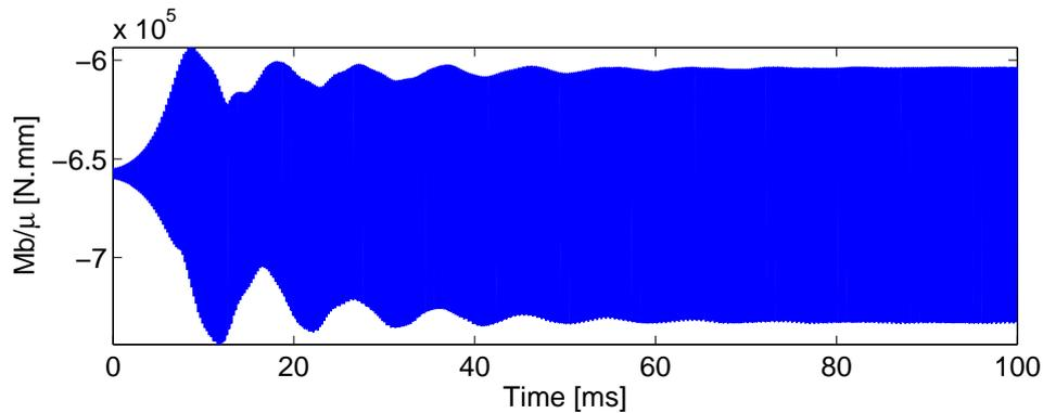
Figure 4.50: 100ms of the real brake squeal simulation at 12 Bar, initialized by excitation of mode C44
