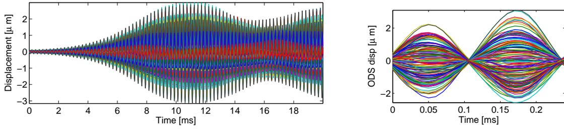
Figure 4.29: Limit cycle installation at 12 Bar triggered by mode C44 target, displacement measured on the disc ODS mesh, and zoom in on a cycle at the simulation end
