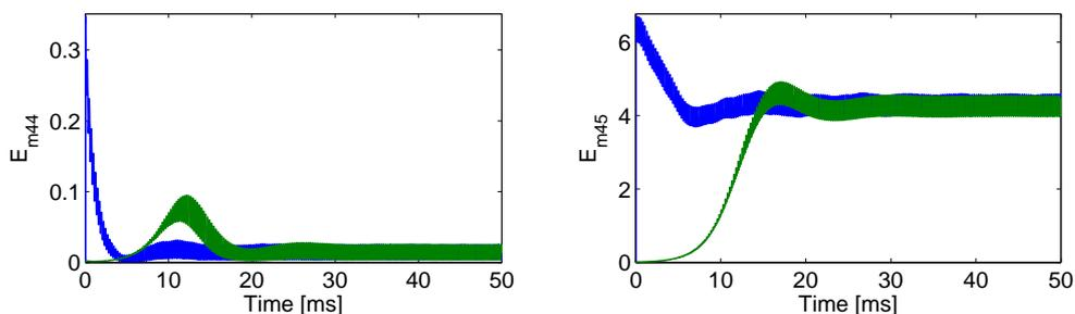
Figure 5.15: Difference evaluation between a limit cycle obtained from a restarted analysis with a 2% mode R44 damping or restarted from time 0. Modal sensor R44 and R45 results
