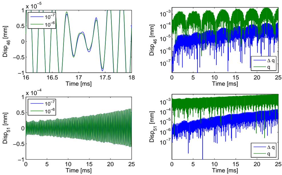
Figure 4.22: Relative displacement error between a  $10^{-7}$  s and  $10^{-6}$  s simulations featuring modal damping on the main instability. Left: displacement signals. Right: nominal signal at  $10^{-7}$  s  $q$  and error between the  $10^{-6}$  s and  $10^{-7}$  s simulations  $\Delta q$
