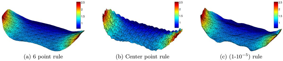
Figure 2.53: Basic contact pressure solution [MPa] for rich rule (6 point), poor rule (1 point), and regularized 1 point observation using shapes computed with the 6 points rule
