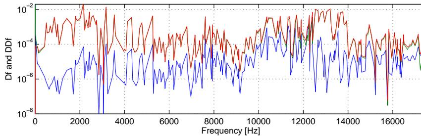
Figure 2.34: Relative error between the 250 first real modes of the ABAQUS recomputed solution and the SDT prediction. [—] Relative error on the frequencies. [—] Relative frequency shift computed with SDT. [—] Related frequency shift computed with ABAQUS
