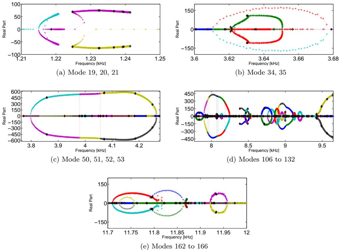
Figure C.4: Stability diagrams as function of the pressure, from 3 to 24 bars. Black edged yellow  $\diamond$  (*resp.* black edged red  $\diamond$ ) stand for the first (*resp.* last) design points of a sub-job
