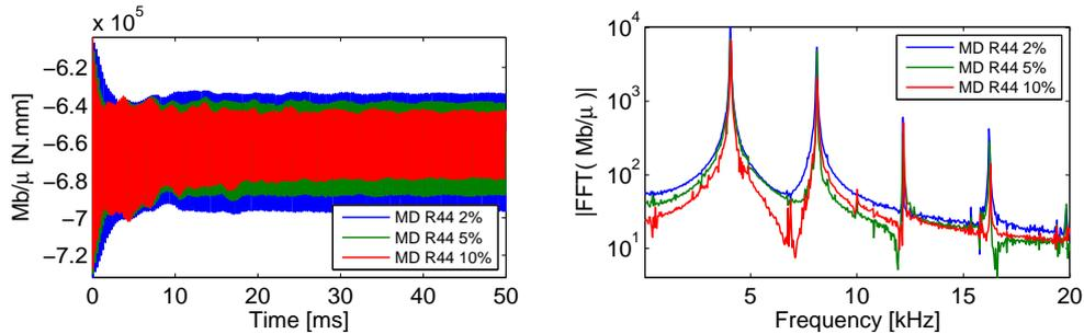
Figure 5.21: Braking torque and its FFT for a limit cycle continuation with mode R44 damping, as function of the ratio
