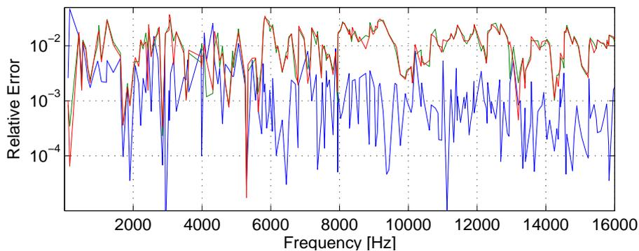
Figure 2.29: Relative error on the real modes predicted by the reduced model and a full ABAQUS recomputation for a 10% increase of the disc Young modulus. [—] Relative error on the frequencies. [—] Relative frequency shift computed with SDT. [—] Relative frequency shift computed with ABAQUS
