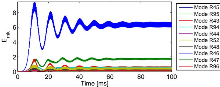
Figure 4.53: Modal sensors results for the 100ms simulation at 12 Bar, initialized by excitation of mode C44
