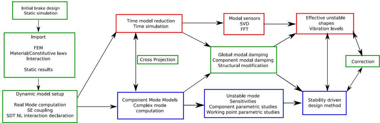
Figure 6.1: A suggestion of brake squeal simulation integrated in an NVH procedure
