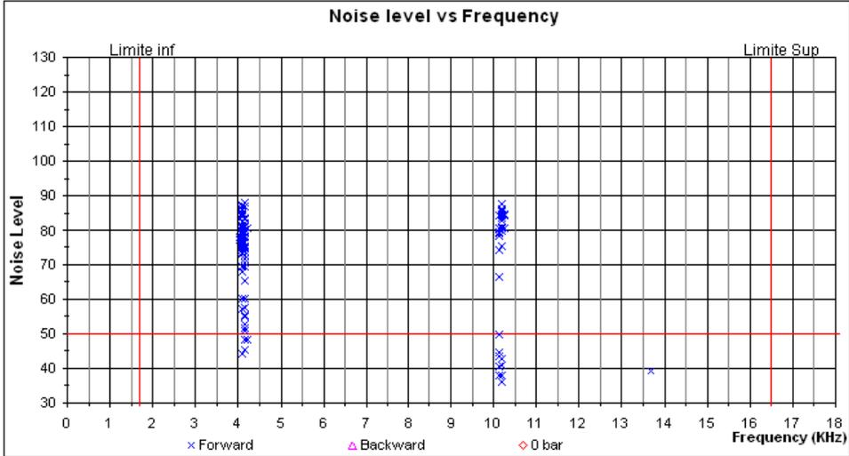
Figure 1.12: Experimental squeal results for the modeled brake
