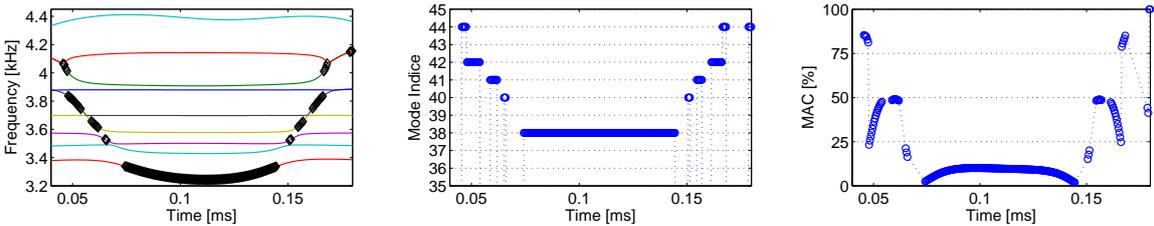
Figure 5.10: Identification of the moving shape in the frequency diagram, mode tracking indices and MAC against the nominal unstable mode
