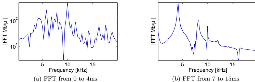
Figure 4.25: Braking torque FFT during the simulation
