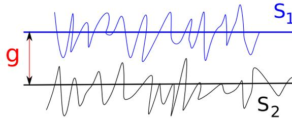
Figure 3.4: Illustration of roughness against nominal surfaces
