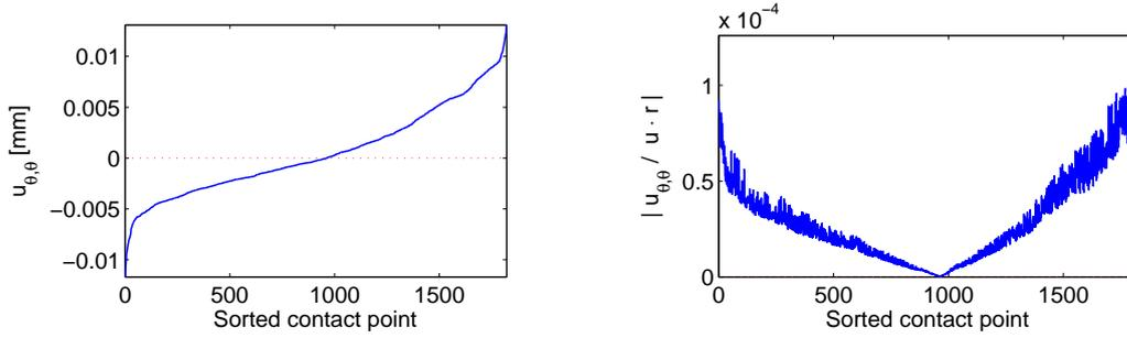
Figure 3.12: Convection term  $J(x_i) \frac{\partial u_\theta}{\partial \theta}_i$  [mm] sorted in increasing order (left) for both pads and comparison (right) to the disc rigid rotation term at 12 Bar, for a disc rotation velocity of  $5 \text{ rad/s}$
