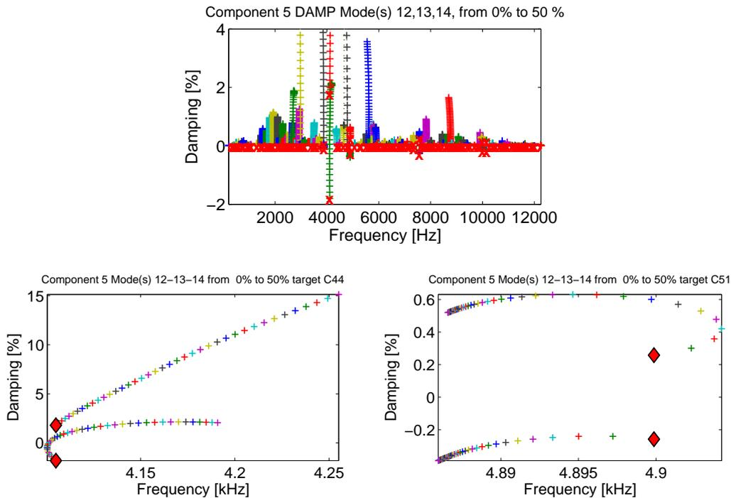
Figure 5.47: Effect of damping caliper mode 12 to 14 on the stability of the global system, from 0 (red diamond) to 50%. Zooms in are performed for modes C44 and C51
