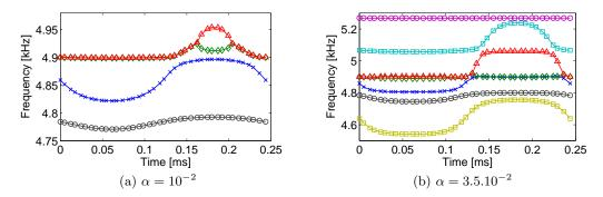
Figure 3.31: Frequency evolution of modes around mode C51 (4.9kHz) over an oscillation based on mode C44 pseudo cycle
