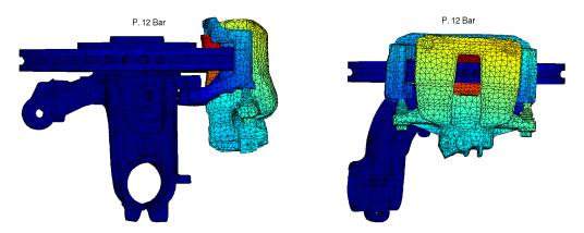
Figure 1.9: Static deformation of the industrial brake model for a braking pressure of 12 Bar
