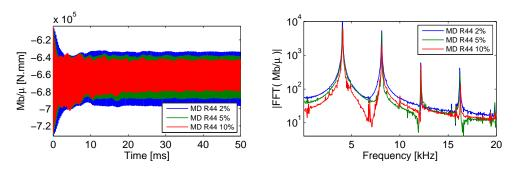
Figure 5.21: Braking torque and its FFT for a limit cycle continuation with mode R44 damping, as function of the ratio
