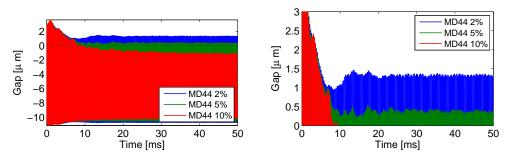
Figure 5.23: Effect of mode R44 damping on a slip-separation pattern, sample contact point. Left: global view. Right: zoom in
