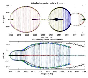
Figure 2.37: Details of the stability diagram as function of  $E_{zz}$ . (+) makers stand for the high  $E_{zz}$  value, ( $\diamond$ ) for the low value used in the reduction basis
