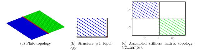
Figure 2.2: CMS applied to a square plate cut in two. (I) for interface, (Ci) for complementary DOF of structures #1 and #2
