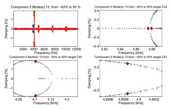
Figure 5.41: Effect of caliper mode 13 frequency tuning from -50 to +50 % on the global system stability at 12 Bar. Red diamond stands for the nominal state
