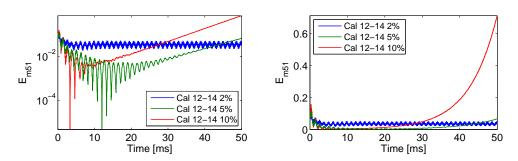
Figure 5.60: Effect of damping caliper mode 12 to 14 on the limit cycle obtained at 12 Bar, modal mechanical energies associated to mode C51
