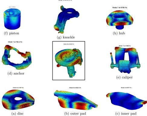
Figure 2.26: Real Brake assembly and components. Modeshape illustrations
