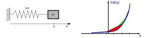
Figure 4.5: Exponential spring example showing approximations generated by the discretization in non linear cases, for a mass-spring system
