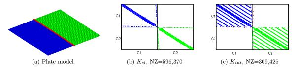
Figure 2.6: Finite element matrix topologies for the CMT formulation. Half-plate #1 in blue, #2 in green. Interface made of spring elements in red
