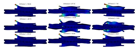
Figure 5.30: Principal shapes extracted from the limit cycle continuation. Top: nominal (no modal damping) simulation. Middle: 2% mode R44 damping. Bottom: 2% mode R45 damping
