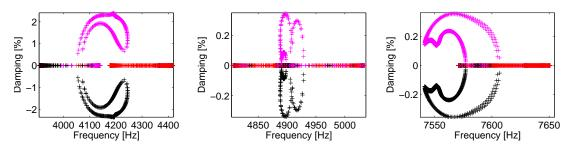
Figure 5.8: Dynamic stability diagrams for modes C44, C51 and C84 (left to right)
