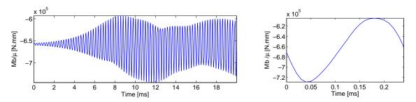
Figure 4.28: Limit cycle installation at 12 Bar triggered by mode C44 target and zoom in on a cycle at the simulation end
