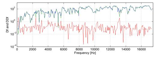
Figure 2.30: Frequency shift error. [-] Shift between the ABAQUS models ( $\Delta f_{abq}$ ). [-] Shift between the SDT models ( $\Delta f_{SDT}$ ). [-] Relative error between the predicted shift and the actual shift computed with ABAQUS ( $\Delta (\Delta f)$ )
