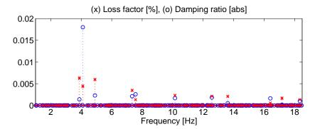
Figure 3.26: Loss factor due to friction in percent against the modal damping ratios in absolute values
