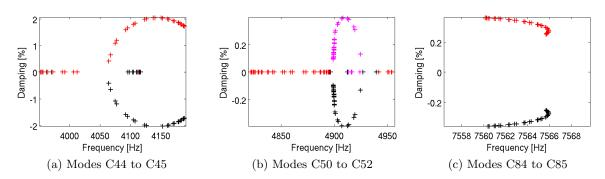
Figure 3.30: Pole evolution of sample modes as function of an oscillation over a pseudo cycle of mode C44 for amplitude  $\alpha = 10^{-2}$
