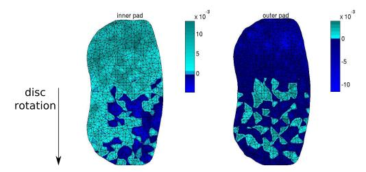
Figure 3.11: Convection term  $\frac{\partial u_{\theta}}{\partial \theta}$  [mm] for the real brake pads at 12 Bar. Data plotted on a Delaunay triangulation of the Gauss contact integration points
