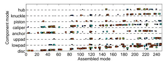
Figure 5.35: Real part sensitivity of the first 250 assembled modes as function of all retained component modes. The hotter the color, the larger the marker, the higher the sensitivity
