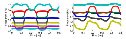
Figure 5.7: Frequency variation of the brake complex modes in the squeal limit cycle at 4 and 5 kHz
