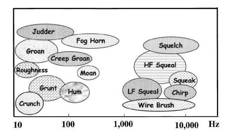
Figure 1.1: Brake noise classification by spectral contents, as proposed by Akay [1]
