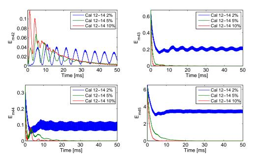
Figure 5.58: Effect of damping caliper mode 12 to 14 on the limit cycle obtained at 12 Bar, modal mechanical energies associated to mode C44
