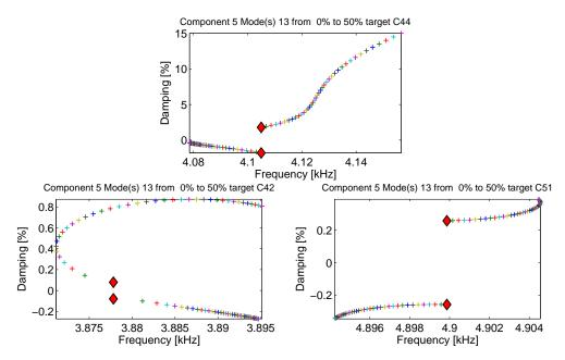
Figure 5.46: Effect of damping caliper mode 13 from 0 (red diamond) to 50% on the stability of the global system, zoomed in on system modes C44, C42 and C51
