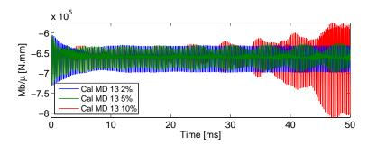
Figure 5.51: Effect of damping caliper mode 13 on the limit cycle obtained at 12 Bar, braking torque
