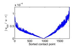
Figure 3.12: Convection term  $J(x_i)\frac{\partial u_{\theta}}{\partial \theta_i}$  [mm] sorted in increasing order (left) for both pads and comparison (right) to the disc rigid rotation term at 12 Bar, for a disc rotation velocity of 5rad/s
