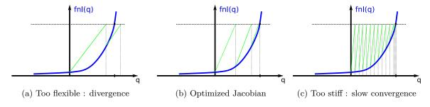
Figure 4.13: Convergence patterns for a Newton-Raphson algorithm with fixed Jacobian illustrated for a single DOF non linear spring showing an exponential shape
