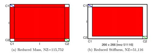
Figure 2.4: Topology of the assembled mass and stiffness matrices using Craig-Bampton reduction for the plate split in two. 20 interface modes kept for both half-plates
