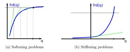
Figure 4.12: Convergence pattern for a genuine Newton-Raphson algorithm illustrated for a single DOF non linear spring depending on its evolution trend
