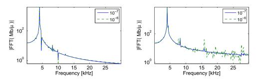
Figure 4.23: FFT of the braking torque signal between 1 and 10 ms (left) and 15 and 25 ms (right), as function of the time step
