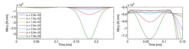
Figure 3.25: Braking torque as function of mode C44 pseudo cycle vibration amplitude, and zoom in on between 0 and 0.15ms
