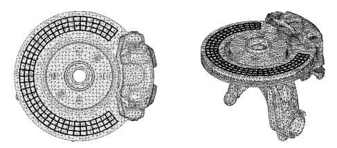
Figure 1.10: Observation mesh placed on the disc for Operational Deflection Shapes (ODS)
