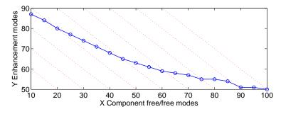
Figure 2.11: Number of enhancement modes kept by the orthogonalization process from the 100 retained as function of the number of component modes retained.
