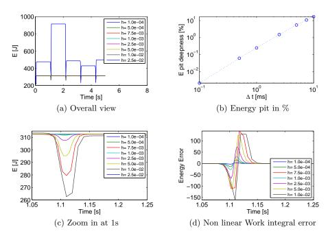
Figure 4.7: Mechanical energy of a mass-exponential spring launched with an initial velocity as function of the time step. Energy pits in percentage relative to the expected mechanical energy. Illustration of the integral approximation error (d), by computing the difference between the work assuming a piece-wise linear variation of the non linear exponential force between computation points and its exact formulation
