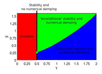
Figure 4.4: Newmark scheme stability diagram
