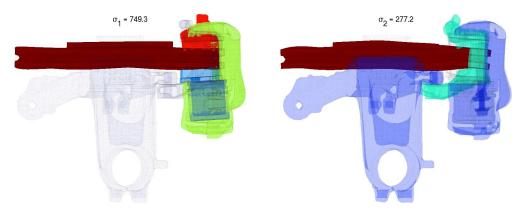
Figure 5.38: Projection of the main shapes computed by the SVD on the component mode model. Strain energy distribution by component
