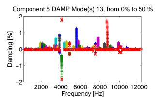
Figure 5.45: Effect of damping caliper mode 13 from 0 to 50% on the stability of the global system
