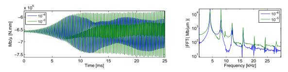
Figure 4.18: Braking torque signal obtained for the real brake model as function of the time step chosen. The FFT is computed from 10 to 20 ms
