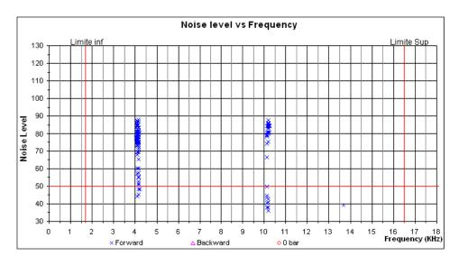
Figure 1.12: Experimental squeal results for the modeled brake
