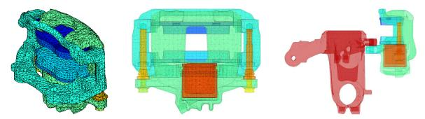
Figure 1.5: Stator part of the brake system
