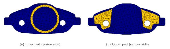
Figure 1.6: Braking pressure transmission areas on the pads
