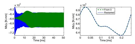
Figure 5.14: Difference evaluation between a limit cycle obtained from a restarted analysis with a 2% mode R44 damping or restarted from time 0. Left: new limit cycle establishment. Right: limit cycle identification
