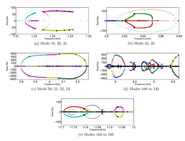
Figure C.4: Stability diagrams as function of the pressure, from 3 to 24 bars. Black edged yellow  $\diamond$  (resp. black edged red  $\diamond$ ) stand for the first (resp. last) design points of a sub-job
