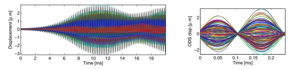
Figure 4.29: Limit cycle installation at 12 Bar trigged by mode C44 target, displacement measured on the disc ODS mesh, and zoom in on a cycle at the simulation end
