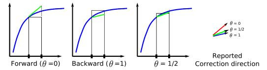
Figure 4.1: Illustration of the interpolation strategy as function of  $\theta$  for the Euler method
