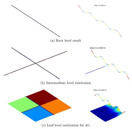
Figure 2.41: Sample restitution of a displacement of the root to its first and second level children
