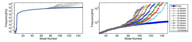
Figure 2.10: Diagonal of the elastic stiffness matrix block (1,1) as function of the number of free/free modes kept. The free blue line corresponds to the component #1 free/free mode frequencies, as a reference. Left: global picture. Right: zoom in.
