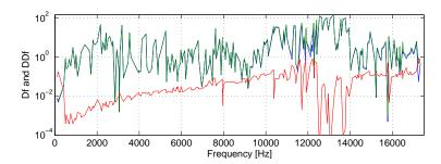
Figure 2.35: Frequency shift error. [-] Shift between the ABAQUS models  $(\Delta f_{abq})$ . [-] Shift between the SDT models  $(\Delta f_{SDT})$ . [-] Relative error between the predicted shift and the actual shift computed with ABAQUS  $(\Delta(\Delta f))$
