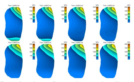
Figure 5.6: Outer pad contact stiffness cartography variation in the squeal limit cycle
