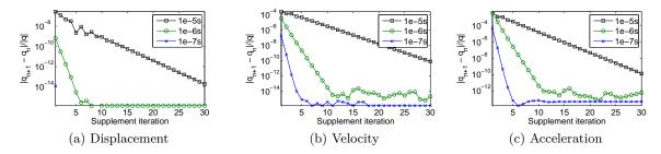
Figure 4.16: Real brake time simulation convergence pattern as function of the time step at 12 Bar
