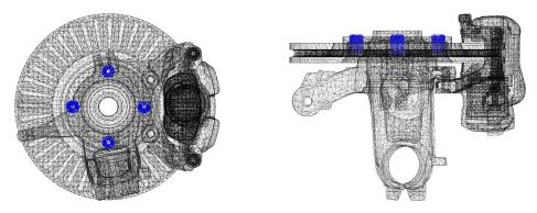
Figure 1.8: Bolt fixation DOF of the rotor with the wheel (o)
