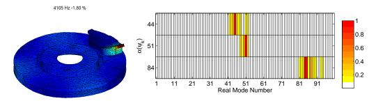
Figure 4.38: Unstable mode C44 and its projection on the real modes
