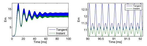
Figure 5.4: Actual mechanical energy of the non-linear system (*Instant*) against the total mechanical energy of the tangent system (*Tangent*)
