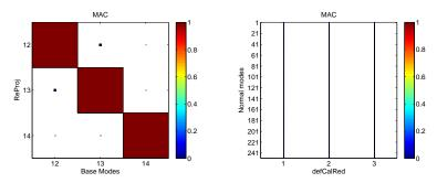
Figure 5.50: Left: MAC between the caliper component modes and the restitution of the projected shapes on the reduced time model restricted to the caliper. Right: MAC between the projected caliper modes and the system real modes
