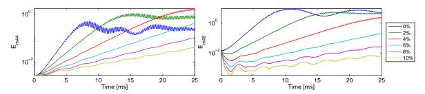
Figure 4.37: Modal sensor for modes R44 and R45 as function of mode R45 damping
