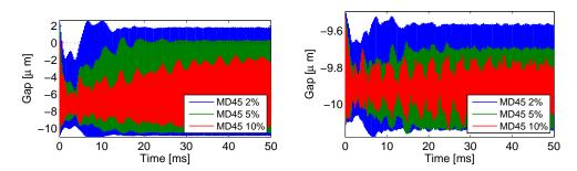
Figure 5.19: Effect of mode R45 damping on a slip-separation pattern, two sample contact points
