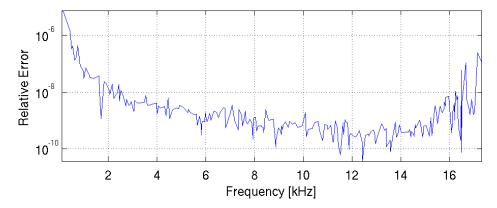
Figure 2.28: Difference between the full brake model and the reduced model: real frequencies
