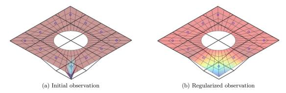
Figure 2.48: Initial and regularized observation for a given Gauss integration point (o) of the master surface
