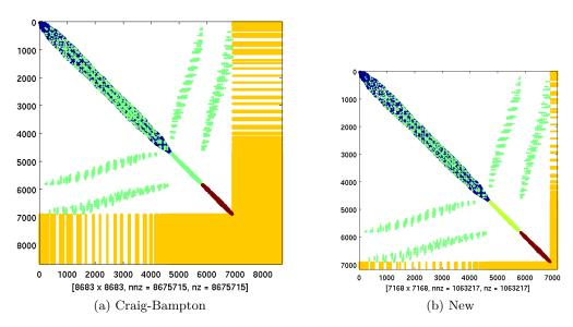
Figure 2.16: Reduced matrix topologies for the 4 nodes linear tetrahedron model. Left: Craig-Bampton reduction. Right: proposed reduction
