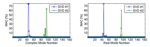
Figure 4.60: Correlation between the principal shapes given by the SVD and the brake steady state complex (left) and real (right) modes through a MAC computation
