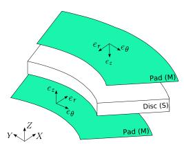
Figure 3.9: Local frame definition of the pad/disc contact
