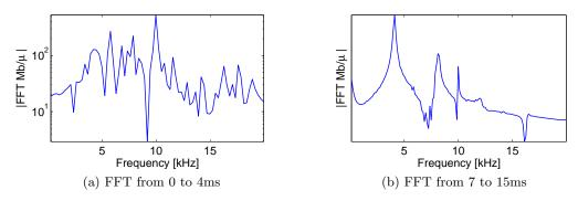
Figure 4.25: Braking torque FFT during the simulation
