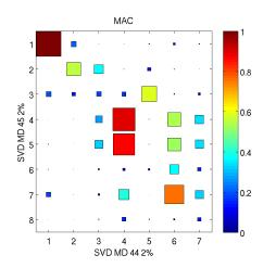
Figure 5.32: MAC between the SVD shapes extracted from the limit cycle continuation with 2% mode R44 damping and 2% mode R45 damping
