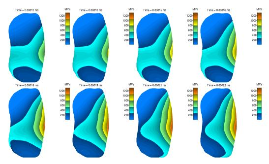
Figure 5.5: Inner pad contact stiffness cartography variation in the squeal limit cycle
