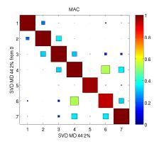
Figure 5.16: Difference evaluation between a limit cycle obtained from a restarted analysis with a 2% mode R44 damping or restarted from time 0 MAC between the shapes obtained by the SVD on the limit cycles
