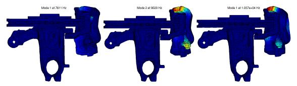
Figure 5.48: Caliper mode shapes 12, 13 and 14 projected on the global time model
