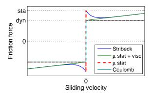
Figure D.1: Illustration of friction static models
