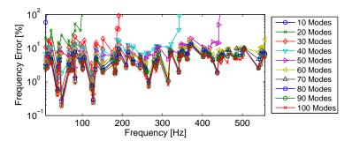
Figure 2.12: Frequency error using a reduction basis only featuring component free/free modes
