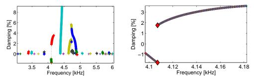
Figure 5.43: Effect of damping disc modes 18 and 20 from 0 (red diamond) to 20% on the stability of the global system, and zoom in on mode C44
