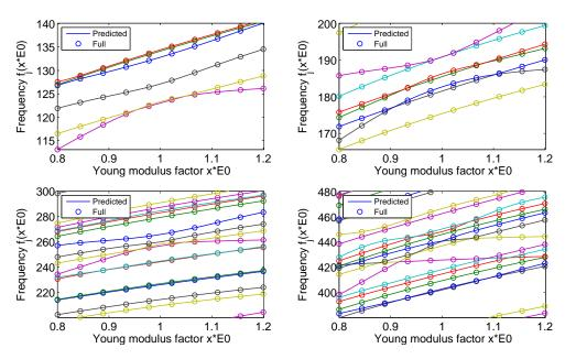
Figure 2.20: Plate frequency variation as function of the Young modulus variation of half-plate #1, predictions from the CMT (-) and recomputations (o)
