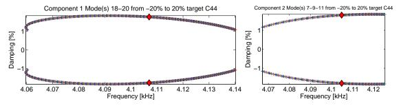
Figure 5.40: Attempt to alter mode C44 instability by tuning disc modes 18 and 20 (left) and by tuning the first pad bending modes (7, 9, 11) (right). Red diamond stands for the nominal state
