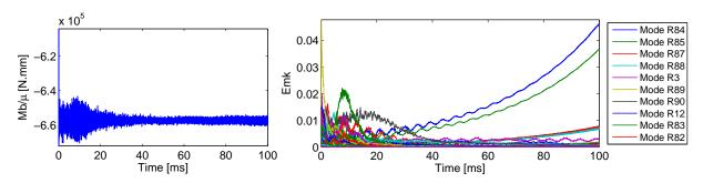
Figure 4.45: Brake squeal simulation at 12 Bar, braking torque and main modal mechanical energies. Modes R42 to R48 damped at 10%, initialization by a 10% pressure step
