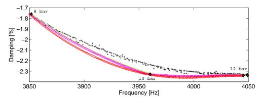
Figure C.5: Various interpolation strategies between 8 and 12 bar. + Linear interpolation between 8 and 12 bar. + Piecewise interpolation between 8 and 10 bars then 10 and 12 bar.  $\diamond$  Piecewise interpolation between 8 and 12 bar using 3 reduction bases at 8, 10 and 12 bar.  $\diamond$  3 points quadratic interpolation using 8,10 and 12 bar
