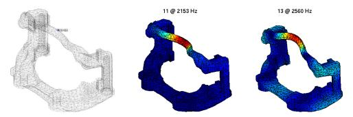
Figure 2.32: Local mass modification of the Anchor handle. Added mass location and the first two altered modes
