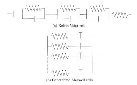
Figure 4.32: Viscoelastic rheological models, using cells of spring dashpot assemblies
