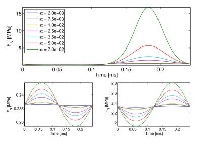
Figure 3.24: Sample contact force oscillation patterns on mode C44 pseudo cycle as function of the vibration amplitude
