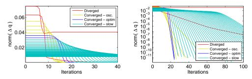
Figure 4.11: Convergence pattern plotting the correction increment quadratic norm as function of the iterations in the Newton-Raphson resolution and as function of the Jacobian parameter  $k_c$ . Left: linear y scale. Right: logarithmic y scale
