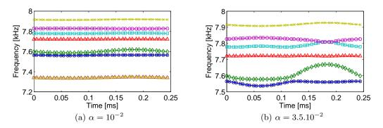
Figure 3.33: Frequency evolution of modes around mode C84 (7.5kHz) over an oscillation based on mode C44 pseudo cycle
