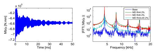
Figure 5.25: Left: Braking torque for a limit cycle continuation with mode R44 and R45 2% damping. Right: braking torque FFT for several modal damping strategies over modes R44 and R45
