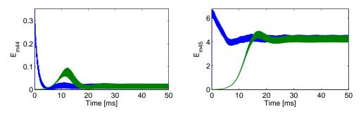
Figure 5.15: Difference evaluation between a limit cycle obtained from a restarted analysis with a 2% mode R44 damping or restarted from time 0. Modal sensor R44 and R45 results
