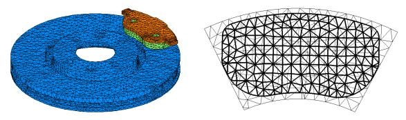
Figure 2.50: Pad/Disc model and superimposed interface discretization
