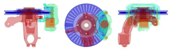
Figure 1.2: Global view of the industrial brake model provided by Bosch
