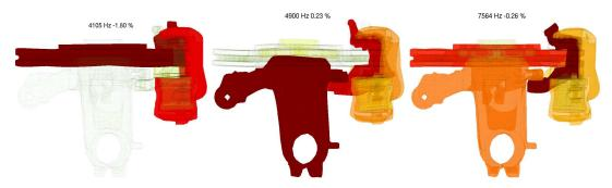
Figure 3.20: Main unstable modes at 12 Bar, C44, C51 and C84, strain energy plotted and ranked by components – from transparent blue (low) to solid dark red (high)
