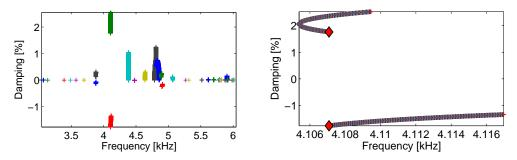
Figure 5.44: Effect of damping outer pad mode 7 from 0 to 20% on the stability of the global system and zoom in on mode C44
