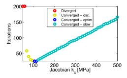
Figure 4.9: Number of iterations necessary to solve the simplified brake static state using the Newton-Raphson method and a fixed Jacobian  $k_c$  between 50 to 500 MPa. Convergence tolerance is fixed at  $\epsilon_{disp} = 10^{-9}$  in a maximum of 200 iterations
