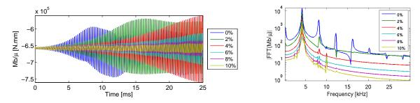
Figure 4.36: Braking torque and its FFT between 1 and 10ms as function of mode R45 modal damping for an initial excitation based on the original unstable mode C44
