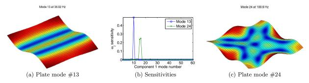
Figure 2.18: Sample sensitivity computation for plate modes #13 and #24. 60 component modes are retained for the reduced model and 100 assembled complex modes
