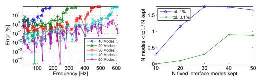
Figure 2.5: Convergence of the 2 components plate reduced by the Craig-Bampton method as function of the number of fixed interface modes kept for each component. Left: frequency error [%]. Right: fraction of modes under the tolerance against the number of interface modes kept
