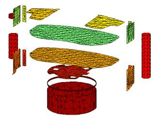
Figure 1.7: Contact elements of the brake system
