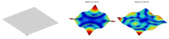
Figure 2.23: Plate node bearing the mass modification. Sample affected mode shapes plotted for the recomputed modes with an additional mass of 0.1 gram.
