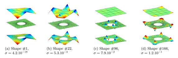
Figure 2.46: Shapes resulting from the SVD of [A] plotted on  $\Gamma_1$  and  $\Gamma_2$ . The gap is computed and plotted on the Gauss points of  $\Gamma$
