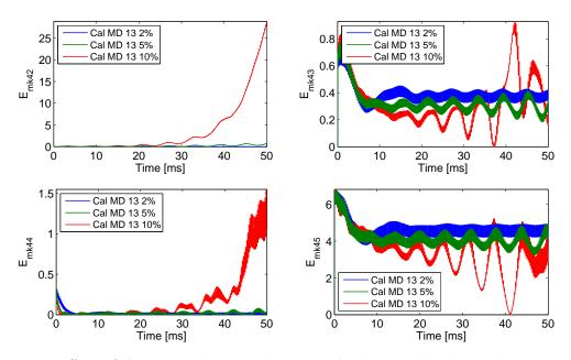
Figure 5.53: Effect of damping caliper mode 13 on the limit cycle obtained at 12 Bar, modal mechanical energies associated to mode C44
