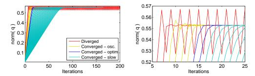
Figure 4.10: Convergence pattern plotting the displacement response quadratic norm as function of the iterations in the Newton-Raphson resolution and as function of the Jacobian parameter  $k_c$ . Left: global view. Right: zoom in a the optimized convergence points
