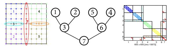
Figure 2.38: Plate sample partitioning, the corresponding elimination tree and reordered matrix
