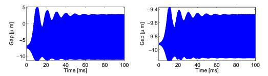
Figure 4.51: Gap computed at sample contact points, one showing a slip-separation pattern (left) and one far from separation (right)
