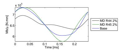
Figure 5.29: Identification of the new limit cycles from the continuation of the base computation with a 2% damping of either mode R44 or mode R45
