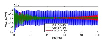
Figure 5.56: Effect of damping caliper modes 12 to 14 on the limit cycle obtained at 12 Bar, braking torque
