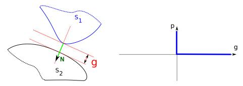
Figure 3.1: Contact normal (N) and gap (g) definition for two solids, and the Signorini contact-pressure law
