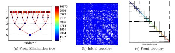
Figure 2.39: Disc mass matrix initial and reordered topologies with elimination tree. Tree color code: vertex DOF size
