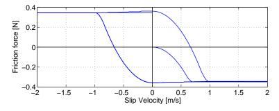
Figure D.5: Sample behavior of the Generalized Maxwell-Slip model
