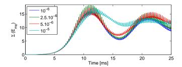
Figure 4.20: Total modal mechanical energy (modes R1 to R500) of the system as function of the time step
