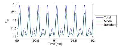
Figure 5.3: Differences between the modal mechanical energy and the total mechanical energy in the squeal limit cycle
