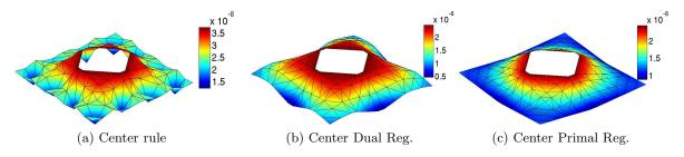
Figure 2.49: Gap observations obtained using the center integration rule for contact, observed on the rich 3x3 rule Gauss points Delaunay triangulation,  $\epsilon = 10^{-5}$
