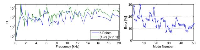
Figure 2.54: Left: Dynamic behavior differences between the use of a 6 point integration rule contact integration law, and the regularization strategy based on a 1 point integration rule for  $\epsilon = 10^{-3}$  (42% of quasi-compatible shapes kept). Right: Frequency differences observed at peaks
