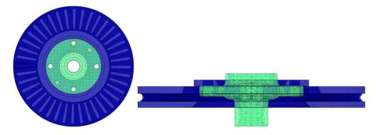
Figure 1.3: Rotor part of the brake system, disc (blue) and hub (green)
