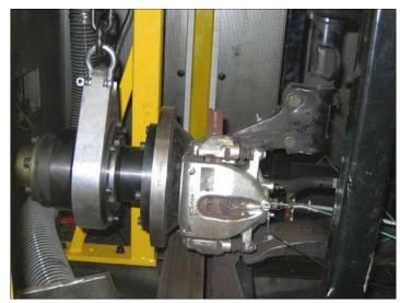
Figure 1.11: A squeal test bench at Bosch facilities
