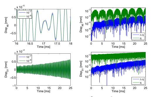
Figure 4.22: Relative displacement error between a  $10^{-7}s$  and  $10^{-6}s$  simulations featuring modal damping on the main instability. Left: displacement signals. Right: nominal signal at  $10^{-7}s$  q and error between the  $10^{-6}s$  and  $10^{-7}s$  simulations  $\Delta q$
