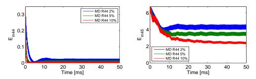
Figure 5.22: Modal sensors R44 and R45 for a limit cycle continuation with mode R44 damping, as function of the ratio
