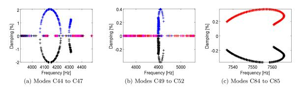
Figure 3.32: Pole evolution of sample modes as function of an oscillation over a pseudo cycle of mode C44 for amplitude  $\alpha = 3.5.10^{-2}$
