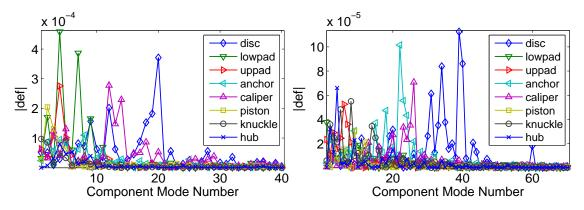
Figure 5.39: Projection of the principal shapes given by the SVD on the component modes through the component mode model. Left: SVD singular shape #1. Right: SVD singular shape #2
