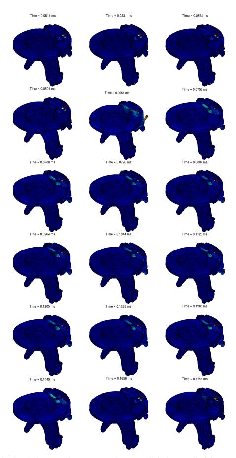
Figure 5.12: Identified moving shapes at several instants of the limit cycle, deformations plotted
