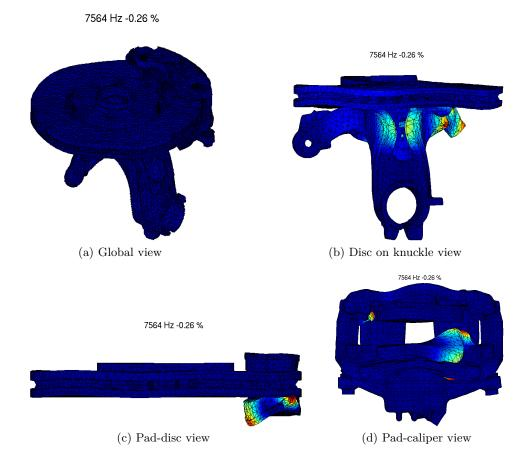
Figure 3.19: Mode C84 shape, colors are re-scaled for each sub-component view
