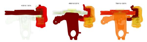
Figure 5.34: Main unstable modes at 12 Bar, C44, C51 and C84, strain energy plotted and ranked by components
