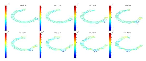
Figure 4.26: Vertical displacement response to the initial pressure step at the simulation start plotted on an observation mesh of the disc. Color code: displacement [mm]
