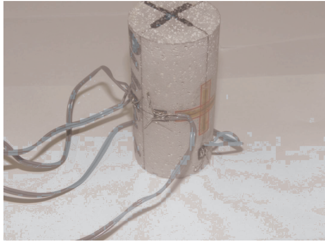
Figure 7.1: Affixed (L) longitudinal and (T) transverse strain gauges on a cylindrical sample
