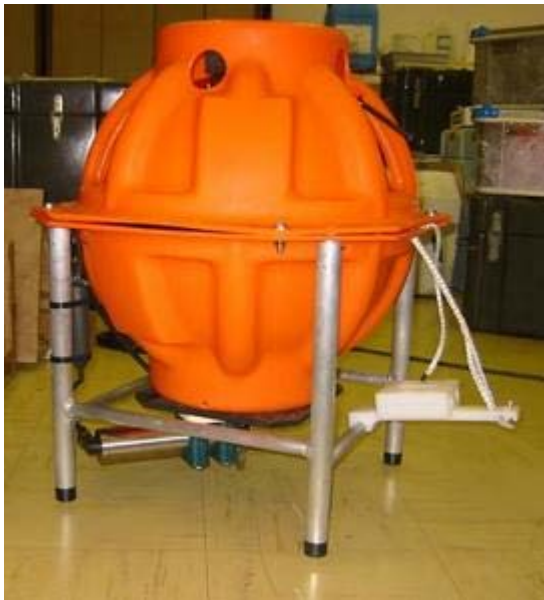
Fig. C6. Overview of a LotOBS with the arm that deploys the pressure-resistant case containing the geophones. The hydrophone, visible in the photograph on the right, is fixed on the instrument's frame, ~0.4 m above the seafloor.
