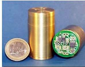
Fig. C12. Picture of geophone SEND “Full Tilt” (height: ~5 cm).
