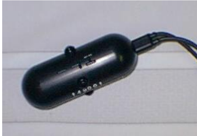
Fig. C5. Picture of hydrophone HTI 90U (length: 10.2 cm)
