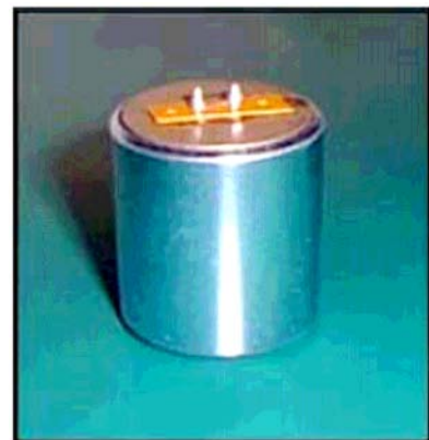
Fig. C2. (Left) Geophone Geospace 4.5 Hz GS11-D characteristics and frequency response curve. (Right) Picture of geophone Geospace 4.5 Hz GS11-D (height: 3.35 cm).
