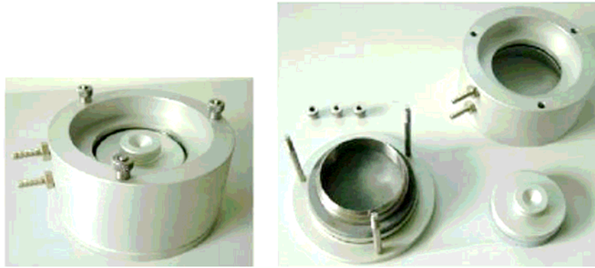
Fig. D14. Picture of a permeametric cell with its accessories (assembled on the left).
