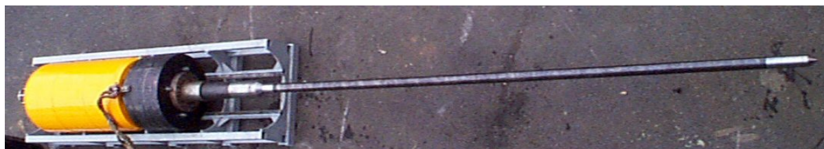
Fig. D1. An Ifremer piezometer with a 3 m long needle presented in its cradle.
