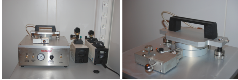
Figure 3.4: Images of the demolding system.
