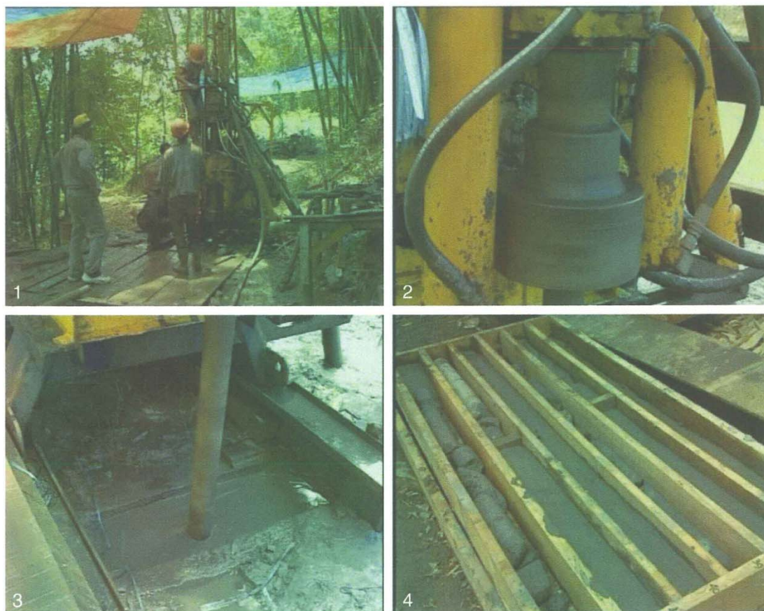
Fig. 3. Rotative corer used for cores 3 and 4. (1) Overall view of the rotary corer; (2) metallic claw and rotation driver; (3) coring barrel collecting sediments, the nature of the coring system tend to mix soft-sediments, and disrupt their orientation therefore we did not practice either palynological or paleomagnetic measures; (4) sample conservation in wood boxes, without plastic case, also seriously limited the range of analysis we could perform on cores, however a rotary corer was the only solution to pierce through andesit lava that represent almost 40% of core 4 (111,5 m depth).
