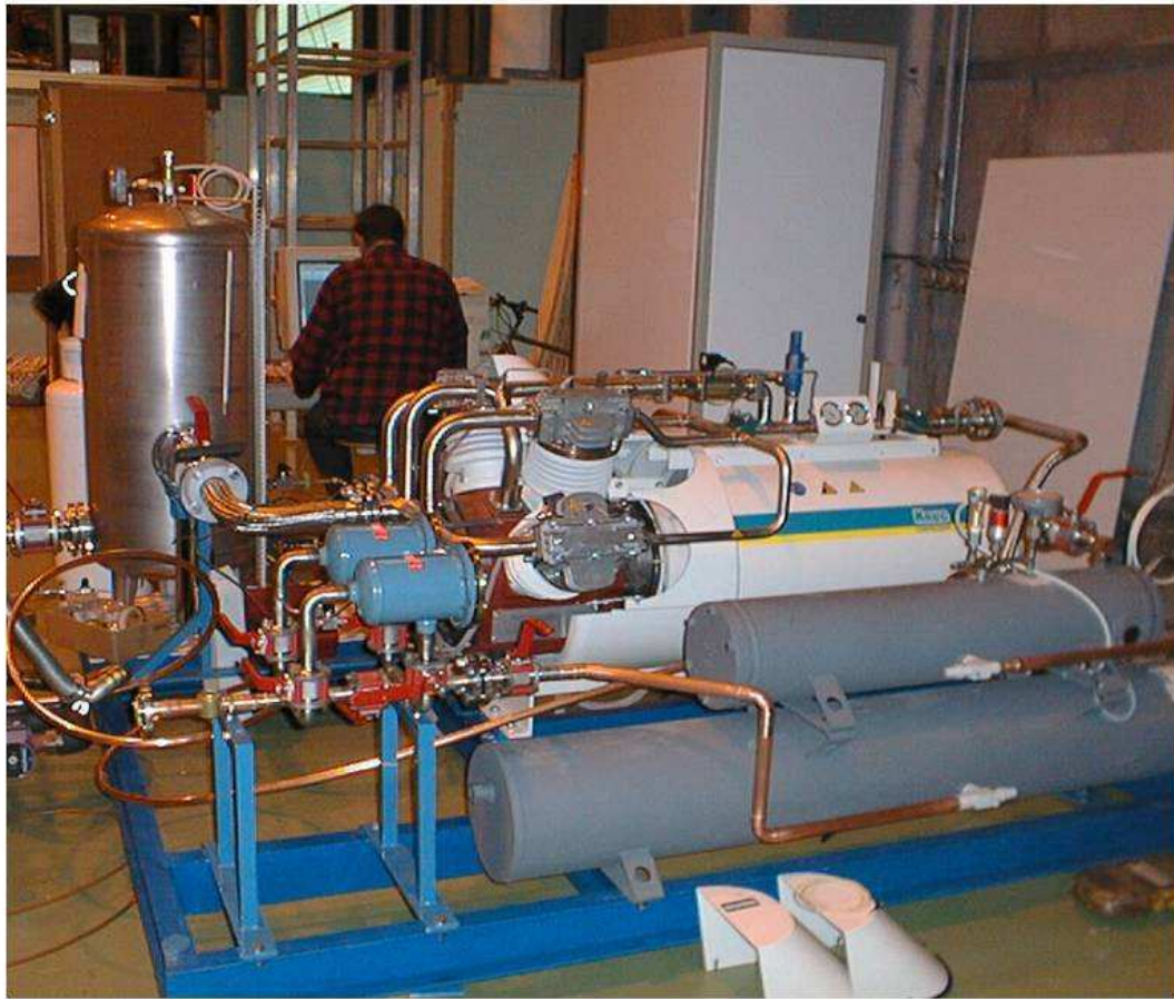
Fig. 4.24. Piston compressor (oil-less, single stage, maximum output pressure 8\text{bar}_{\text{abs}} ) and condenser (foreground) used in multi-channel \text{C}_3\text{F}_8 evaporative cooling demonstrator tests; aspiration buffer tank behind.
