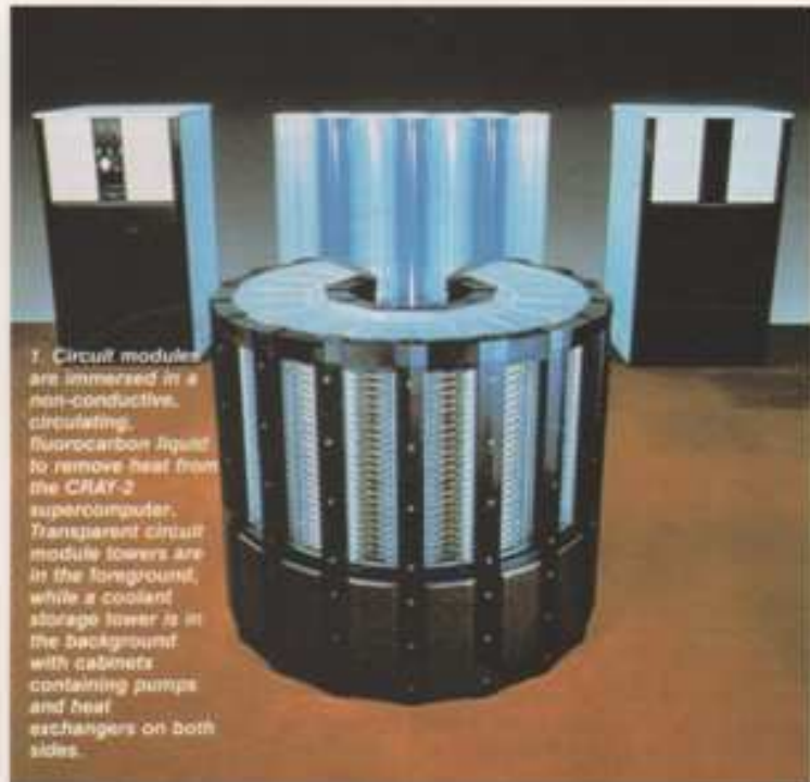
2. Cooling fluid is pumped through the circuit module towers and heat exchangers.
