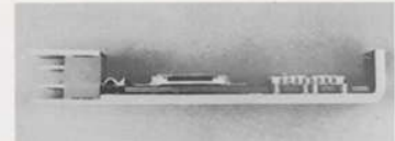
Figure 3 To bear the coefficient of thermal expansion of glass-epoxy multilayer boards, engineers at GE bonded about 42% an incompressible mixture with 42% nickel — between board layers, as it, fastened in this cross section of a LamCores MLB connector frame assembly.
