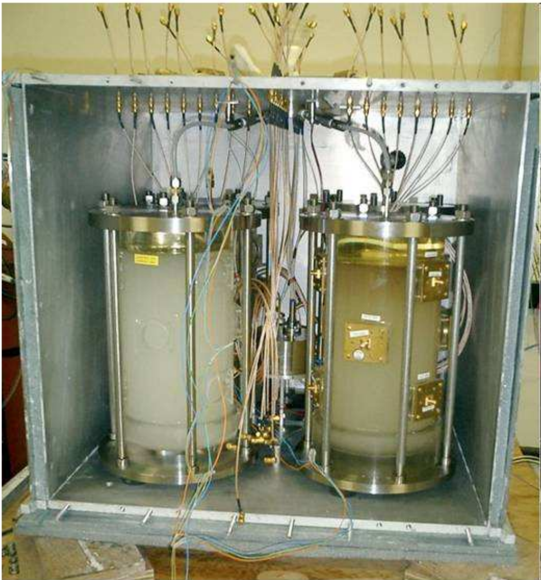
Fig. 8.1. Two of the cylinders of the Picasso dark matter experiment. The connections the piezo acoustic sensors for the triangulation of C_4F_{10} droplet explosion sare shown, together with the tube for C_4F_{10} repressurization.
