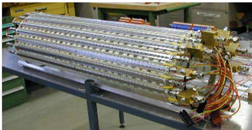
Fig. 4.21 Pixel dummy thermal series staves built for 6kW evaporative cooling demonstrator
