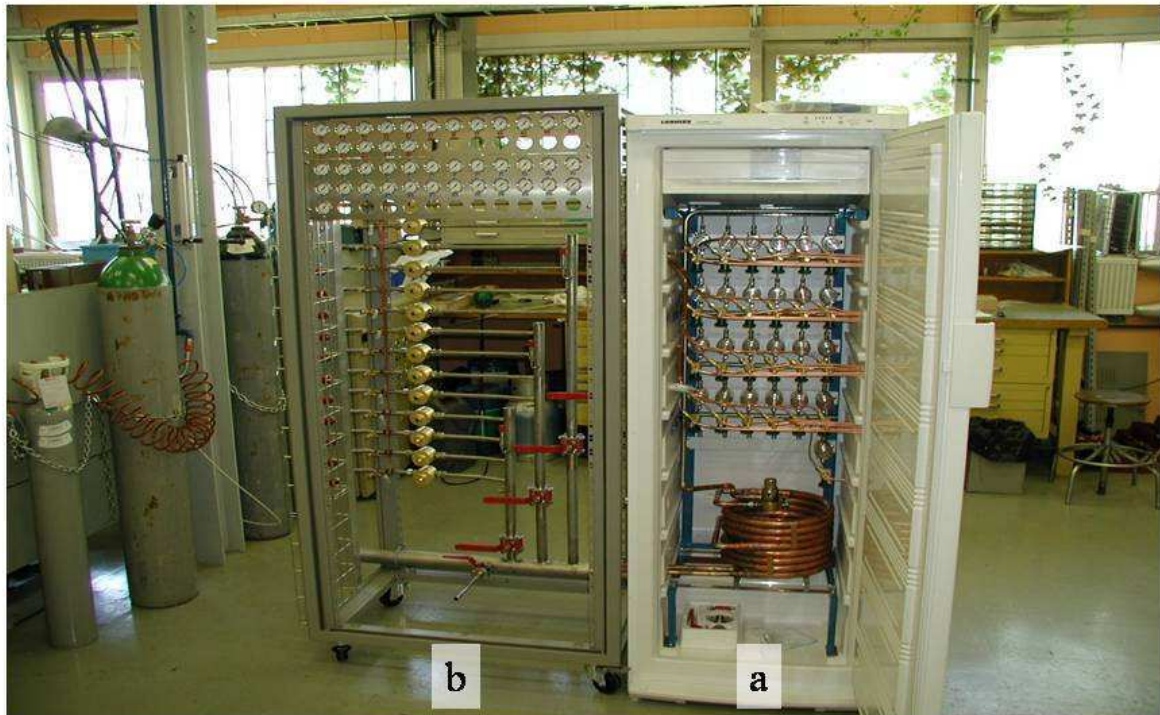
Fig. 4.26. Precooled C_3F_8 liquid flow regulators (a) and evaporation pressure defining back-pressure regulators (b) in the multi-channel demonstrator.
