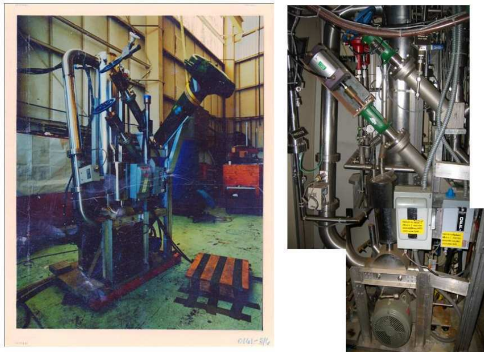
Fig. 2.31. Two views of the Paxton RU80 supercharger assembly: Left - the high flow bypass with high Cv butterfly valve; Centre rear - 300 litre aspiration buffer tank; Centre above electric motor - the water cooled output buffer tank
