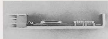
Figure 3 To bear the coefficient of thermal expansion of glass-epoxy multilayer boards, engineers at GE bonded about 42% an incompressible mixture with 42% nickel — between board layers, as it, illustrated in this cross section of a LamCores MLB connector frame assembly.
