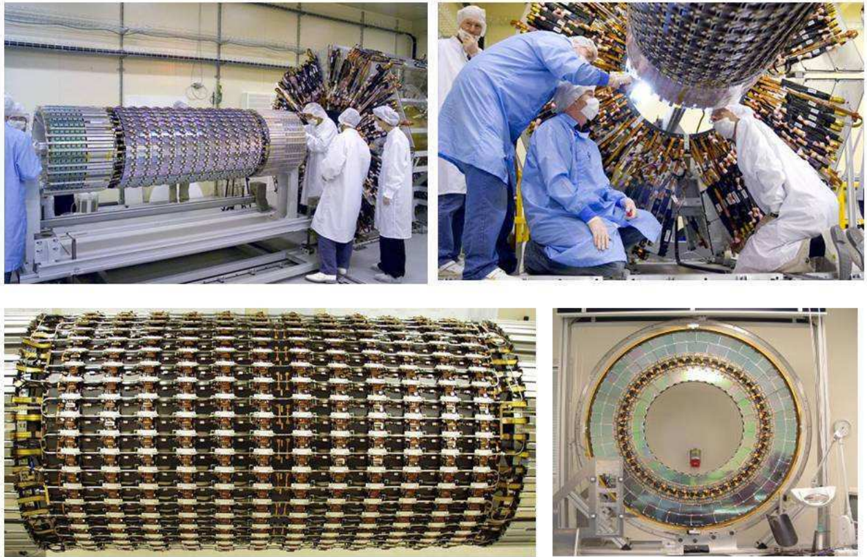
Fig. 4.20 Illustration of the SCT on detector evaporative cooling channel 'quartets' on the outermost SCT layer 4, together with one half of the coolant delivery and exhaust tubing cooling. Complete SCT forward disk for comparison.
