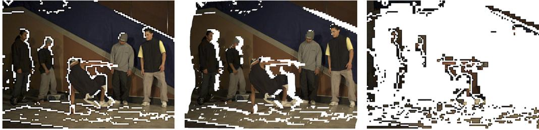
Figure 5.10: One iteration of filling disocclusions. Left:  $\Omega_{k-1}$  polygon soup at iteration  $k - 1$ . Center:  $\Omega_{k-1}$  projected in  $V_i$  (Disocclusions). Right: Selected quads from  $V_i$ .
