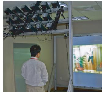
(c) Front-projection 3D display with single-lenticular screen
