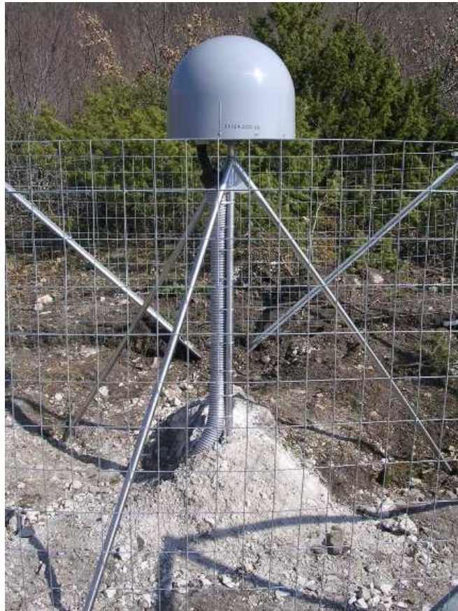
Figure C.1a. Station monument of VAGA.
