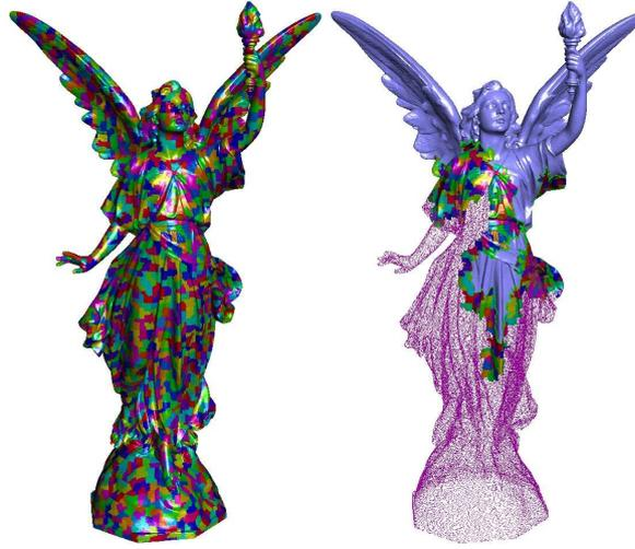
Figure 3.3: Out-of-core compression of the “Lucy” model with the approach of [Isenburg and Gumhold 2003]. The left picture shows the partition of the mesh. The right picture illustrates the compression process. The already compressed clusters are rendered as points, while the rest is rendered as triangles. The cached clusters are coloured. The boundary of the active region is drawn in green. (Figure taken from [Isenburg and Gumhold 2003]).
