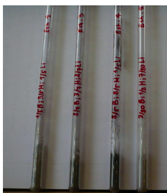
Figure 5.3. Samples of the three-phase system sealed in ampoules under vacuum
